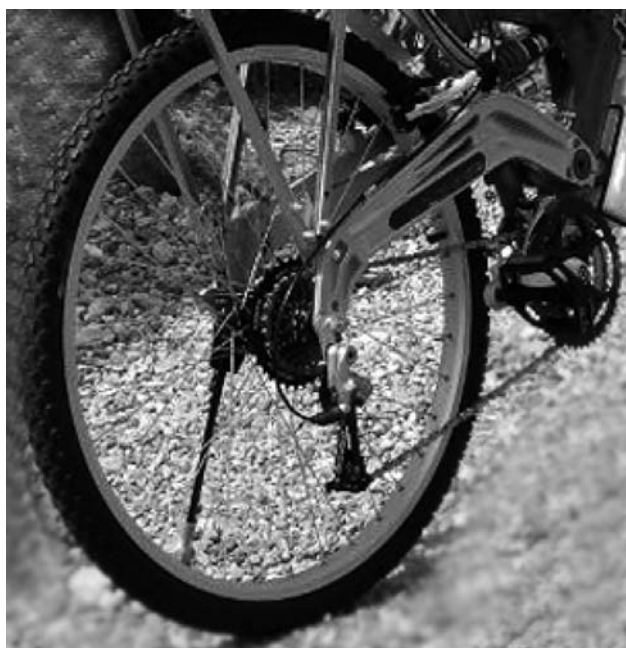
FIGURE 4.25 Bicycle chain drive.
