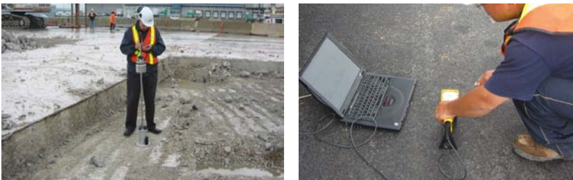
Fig. 5 Portable FWD was used to determine the M_r directly on the surface of the granular base, granular subbase or subgrade during construction (left). Field testing of asphalt concrete pavement with impact-echo equipment to determine cracking and interface conditions (right)
