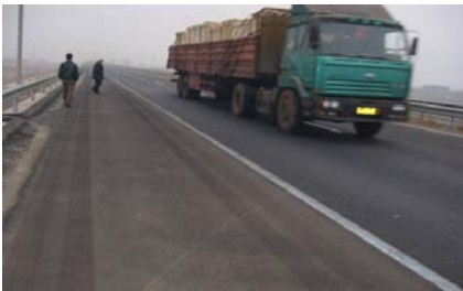
Fig. 2 Typical heavily overloaded truck with poor axle and tire distribution of loadings
