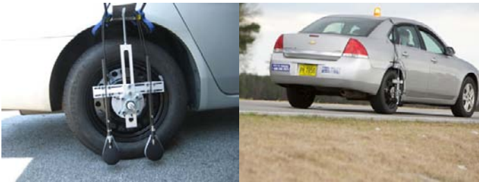
Figure 1. Microphones with windscreens, mounting fixture and cables (Left)
