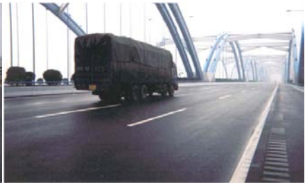
Fig. 2 Typical heavily overloaded truck with poor axle and tire distribution of loadings
