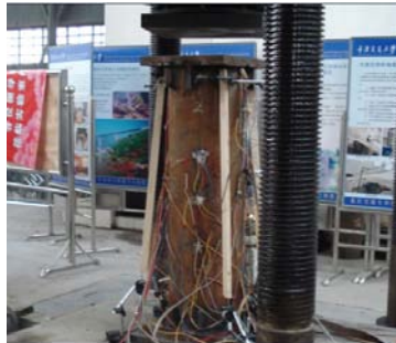
Figure 7 CFST specimen after welding
