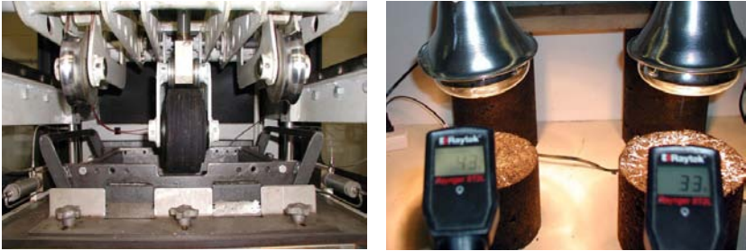
Fig. 4 APA Asphalt Concrete Testing (Left). Hydrated Lime Surface Treatment To Reduce Asphalt Pavement Temperature (Right)
