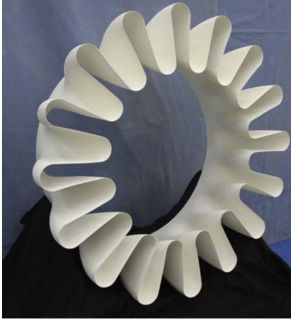
Figure 12.13 Subscale oxide/oxide ceramic matrix composite turbine engine mixer exhaust nozzle demonstrated at the NASA Glenn Research Center.
