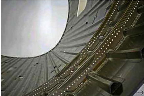
Figure 3.9 Composite fuselage assembly section; the skin panels are manufactured by the AFP process [6].
