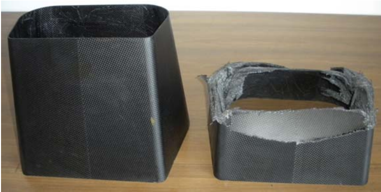
Figure 13.11 Attenuator before and after dynamic test.
