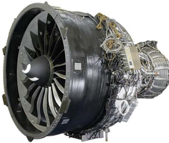
Figure 12.4 Polymer matrix composite fan case for GENx engine used in the Boeing 787 aircraft ( http://www.geaviation.com/commercial/engines/genx/ ).
