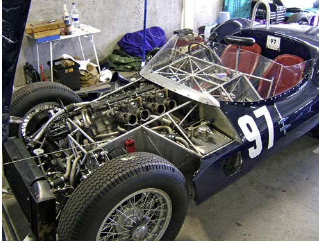
Figure 4.4 Late 1950s Maserati Tipo 61 (aka Birdcage Maserati). Extreme example of an automotive space frame body structure.
