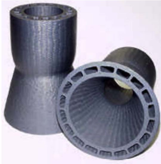
Figure 12.19 Cooled ceramic matrix composite thrust chamber for rocket propulsion.
