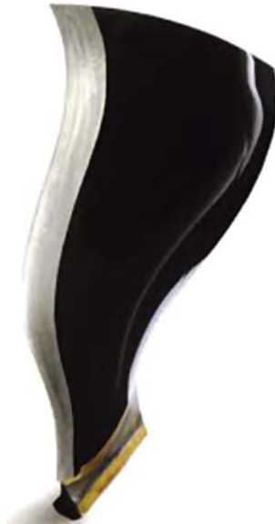
Figure 12.2 Polymer matrix composite fan blade used in the GE-90 gas turbine engine ( http://www.gereports.com/post/74545209282/blast-from-the-past-edisons-discovery-powers ).
