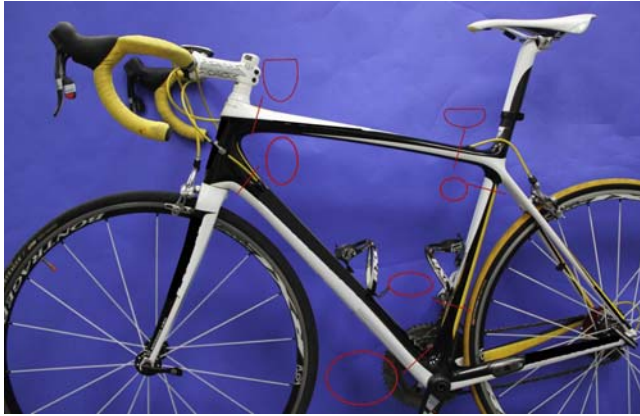
Figure 4.7 High-end carbon fiber racing bicycle frame. From a structural efficiency perspective, bicycle frames such as these are perhaps the most structurally optimized of any consumer product. Every tube at every cross-section has been optimized for shape, wall thickness, and fiber orientation.
