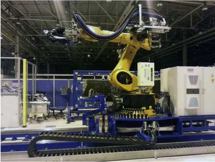
Figure 3.17 Robotic drilling machine.
