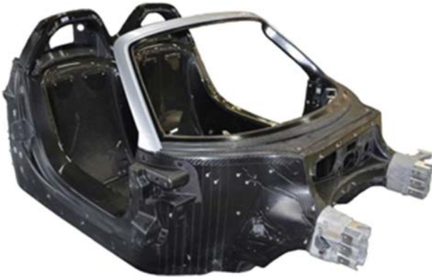
Figure 5.2 Mubea Carbo Tech developed carbon fiber monocoque for the Porsche 918 Spyder. Gardiner, G., 2014. More from JEC: High-Quality Carbon Fiber Monocoques in Two Hours. (Online) Available: http://www.compositesworld.com/blog/post/more-from-jec-high-quality-carbon-fiber-monocoques-in-two-hours .
