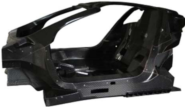
Figure 5.3 Mubea Carbo Tech developed Volkswagen’s new XL1 hybrid diesel featuring a carbon fiber monocoque. Gardiner, G., 2014. More from JEC: High-Quality Carbon Fiber Monocoques in Two Hours. (Online) Available: http://www.compositesworld.com/blog/post/more-from-jec-high-quality-carbon-fiber-monocoques-in-two-hours .
