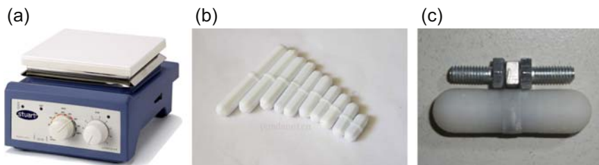
Figure 16.2 (a) Hot plate and magnetic stir bar. (b) Stir bars in various sizes. (c) Stir bar construction.
