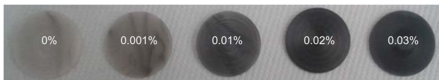
Figure 16.14 Rheology specimens prepared having 0, 0.001, 0.01, 0.02, and 0.03% wt carbon nanotube content.
