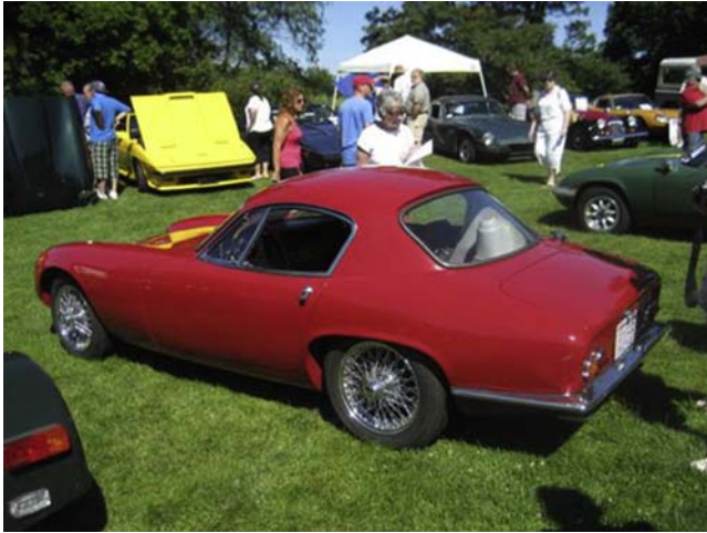
Figure 4.5 Late 1950s Lotus Elite—perhaps the most successful effort to produce an automobile body structure that most closely approaches a true monocoque.
