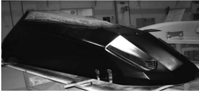
Figure 5.4 The all-composite car body manufactured from the resin infusion process.
