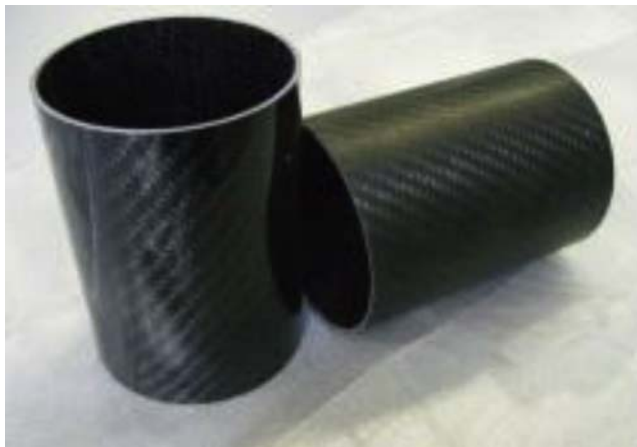
Figure 17.2 An example of a filament-wound rocket tube based on graphite fibers and epoxy resin.
