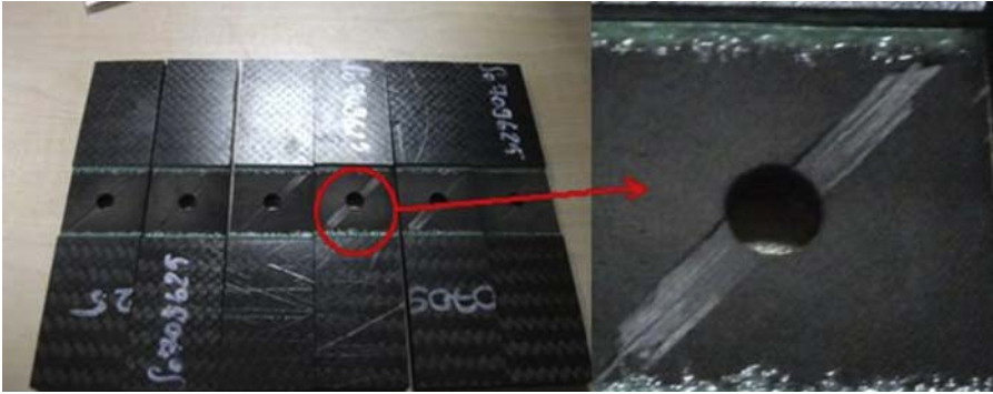
Figure 3.19 Hole flaking after drilling operation on composite parts.
