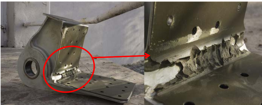
Figure 3.5 Shimming application on actuator fittings.
