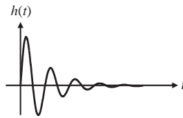
Figure 4.29 Impulse response function for Example 2
