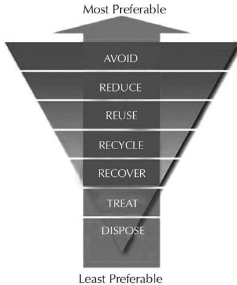
FIGURE 8.3 The waste hierarchy diagram illustrates how waste avoidance is preferred, above re-use and recycling. Disposal in landfill represents the lowest level of the waste hierarchy (diagram: courtesy of the author, 2010). On the municipality level, a more strategic charging structure (levies) for waste disposal can accelerate sustainable waste management and reward residents who are separating their waste.
