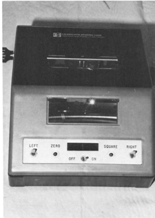
Figure 20. RID viewer for measuring diameter of the precipitate rings. The RID plate is placed on the top of the viewer.
