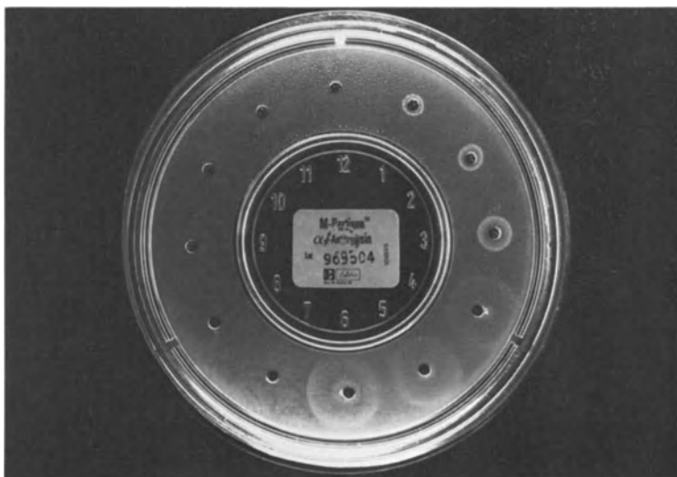
Figure 31. Quantitation of \alpha_1 -antitrypsin by a radial immunodiffusion method.
