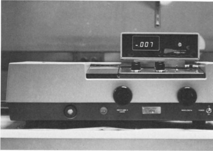
Figure 27. Hitachi Digital Spectrophotometer Model 102 utilized for measuring turbidity in fibronectin immunoassay.
