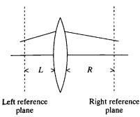
We can characterize the incoming ray by its slope m and its intercept x with the left reference plane. Likewise, we characterize the outgoing ray by slope n and intercept y.
