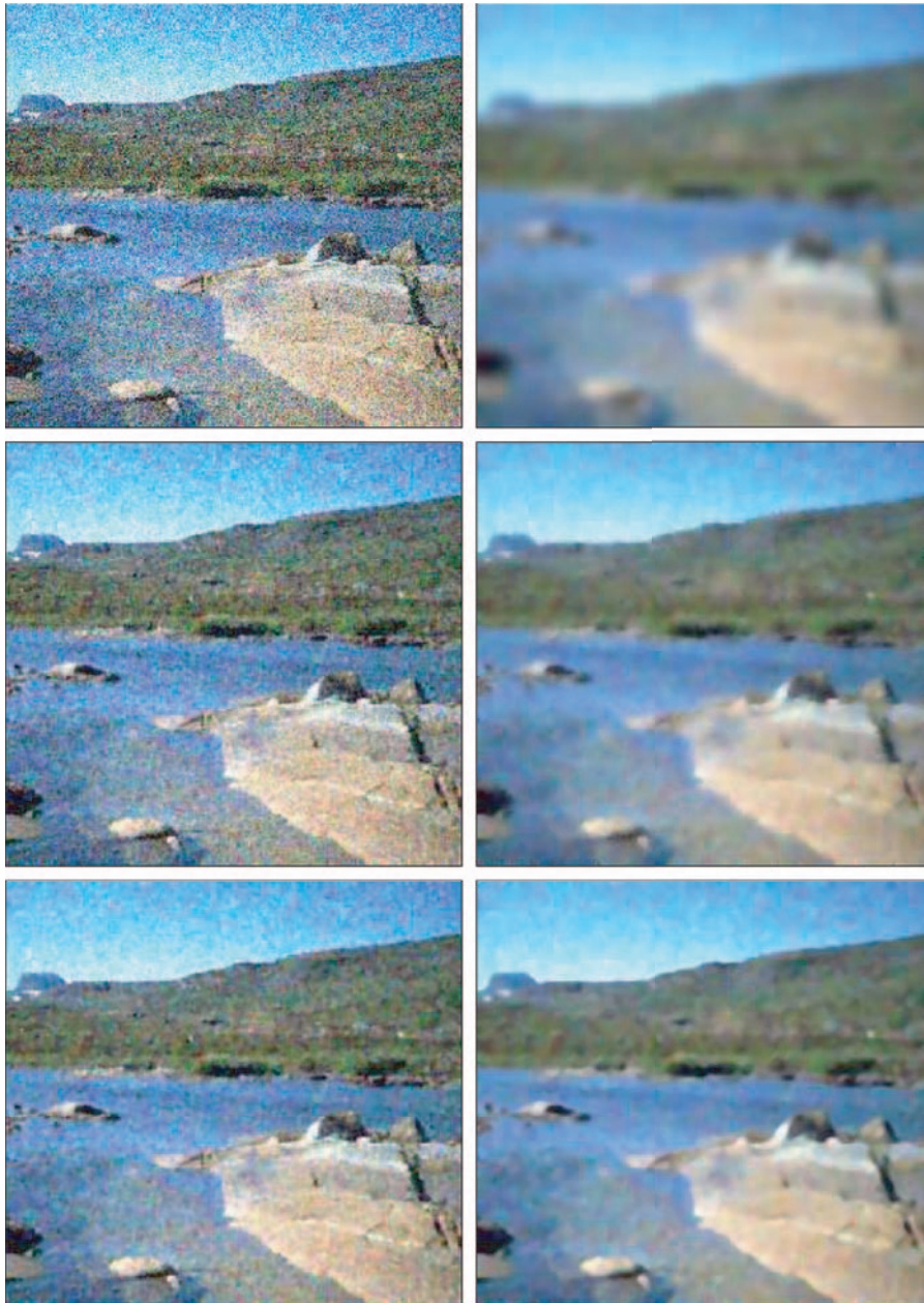
Fig. L. Diffusion filtering of colour images. (a) Top left: Noisy color image. (b) Top right: Homogeneous diffusion. (c) Middle left: Linear isotropic diffusion. (d) Middle right: Linear anisotropic diffusion. (e) Bottom left: Nonlinear isotropic diffusion. (f) Bottom right: Nonlinear anisotropic diffusion. From [89].
