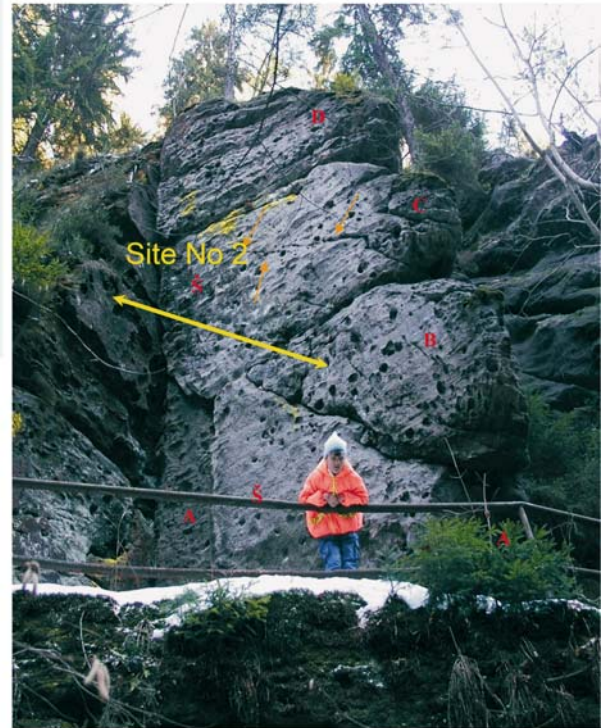
Fig. 14.5. New method of correlograms was used to decipher short, only 4.5 months lasting time series and to launch a rock fall early warning for a rock pillar just above a tourist trail at the bottom of the Wild Gorge of Kamenice River. a Current time/displacement plot from the monitoring key site (for its position see photo) is showing only one irreversible jump shortly after the beginning of measurement. b Temperature/displacement correlogram: ordered patterns of diagonal, from left to right elongated dot clouds represent well correlated responses of rocks to temperature changes. In contrary to the current plot, many temperature independent micro slip events are clearly visible as dot groups violating the left-right diagonal patterns. The high density area of the slip events is marked by a red curve
