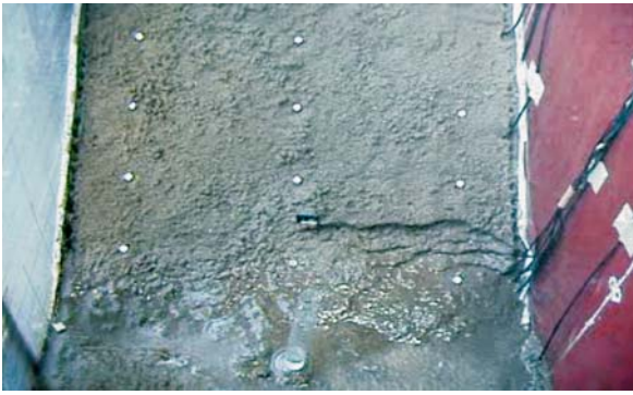
Fig. 16.6. Initiation of rainfall-induced instability from bottom of slope during model tests (case 9 by Shimoma et al. 2004)
