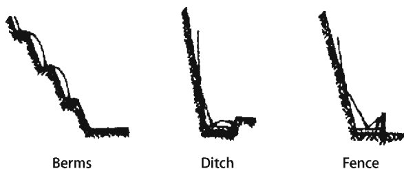
Fig. 31.16. Possible measures to reduce the damage due to rockfalls. Selected after Spang and Rautenstrauch (1988)
