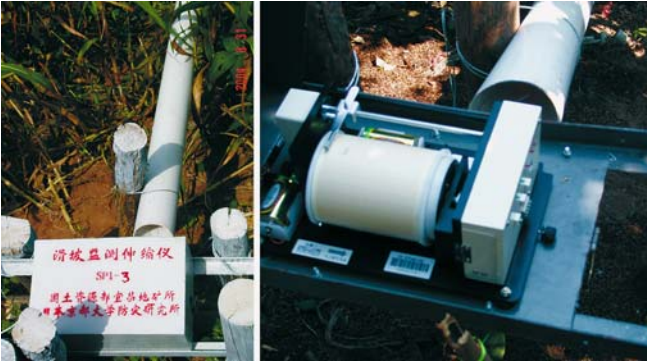
Fig. 40.8. Extensometer installed in Shuping landslide. The deformation is recorded on the rolled paper and also saved in a memory (visible in the right side)
