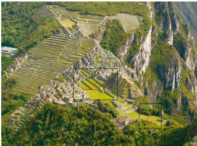
Fig. 4.2. Photo of the archaeological site taken from the top of Mt. Huaynapicchu with localization of two extensometric profiles. Red color: opening; magenta: closing
