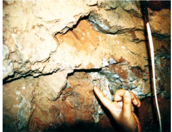
Fig. 9.6. Close-up view of the slickenside within the gently dipping fault (potential sliding surface) found in the lower tunnel
