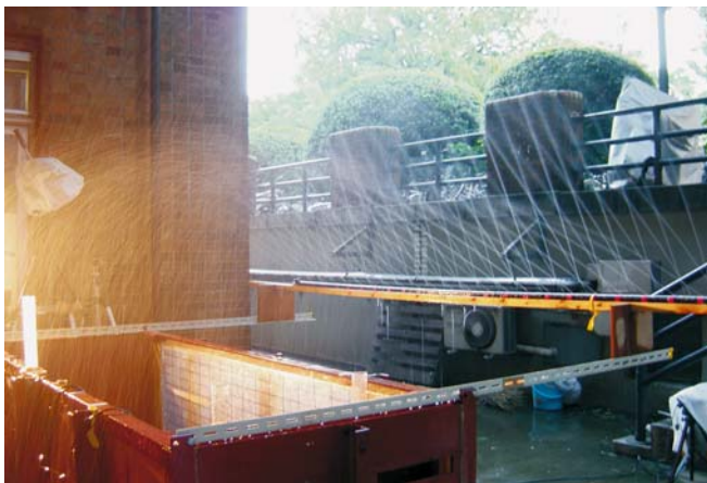
Fig. 16.8. Model test on slope failure with artificial rainfall
