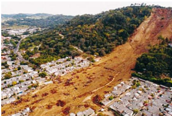
Fig. 41.2. Las Colinas landslide in El Salvador, January 2001, triggered by an earthquake (magnitude = 7.7). The landslide caused more than 600 fatalities
