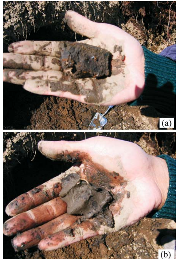
Fig. 25.7. Soil sample taken from lower part of active layer. a Frozen state immediately after sample was taken from scarp. b Soil sample after being melted by hand
