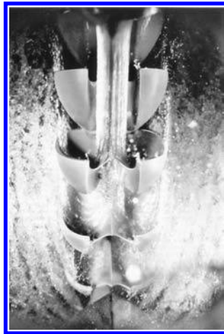
FIGURE 5.16: Water sheets observed at model scale.
