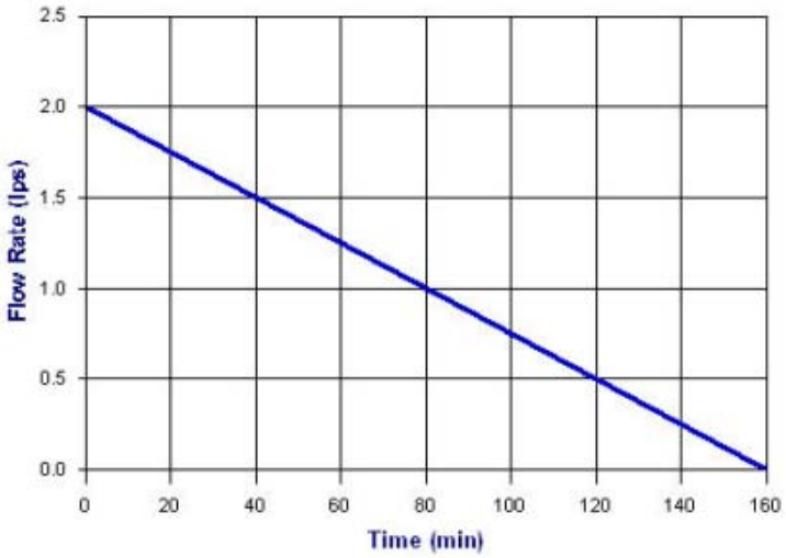
Figure 4: Example of linear gradual reducing inflow hydrograph.
