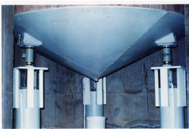
Figure 2: The load cells and foundation of the cylinder.
