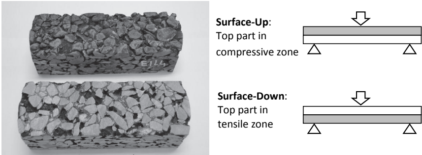
FIG. 3. Picture of the beams from the test section of A50 (left) and two configurations for the stiffness test in 3-point bending test (right).
