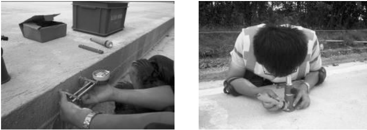
FIG. 3. Crack width measurement by LVDT (left) and Microscope (right)
