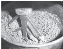
Mortar mixture after adding the aggregate in the cement paste and before the second phase of water dosing
