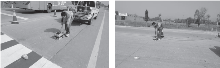
FIG.2. The testing sites based on GPR technology (left: the test along the traffic direction; Right: the test vertical with the traffic direction).
