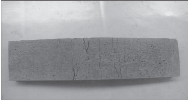
FIG.4. Multiple cracking along the length of the sample.
