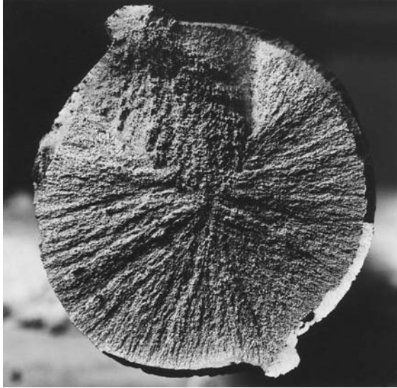
Figure 5.17 Radial markings pointing back to an internal flaw in steel reinforcing bar. (Courtesy of Roger Slutter, Lehigh University.)
