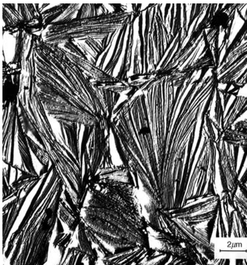
Figure 2.64 Sheaf-like stacks of crystal lamellae in polychlorotrifluoroethylene, which represent intersecting spherulites. 94 (Reprinted with permission from John Wiley & Sons, Inc.)
