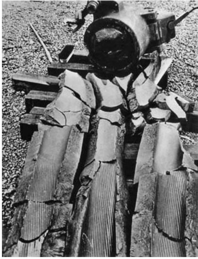
Figure 11.17 Fragments from exploded 175-mm gun tube. (After Davidson et al. 27 )
