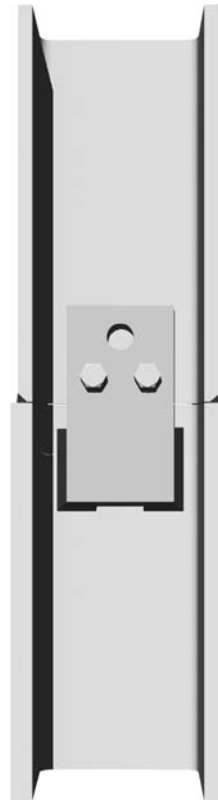
FIGURE 11.40 Column connections may be welded rather than bolted. The connector plate is welded to the lower column section in the fabricator’s shop. The hole in the connector plate is used to attach a lifting line during erection. The bolts hold the column sections in alignment, while the flanges are connected in the field with partial-penetration welds in bevel grooves. Partial-penetration welding allows one column to rest on the other prior to welding.
