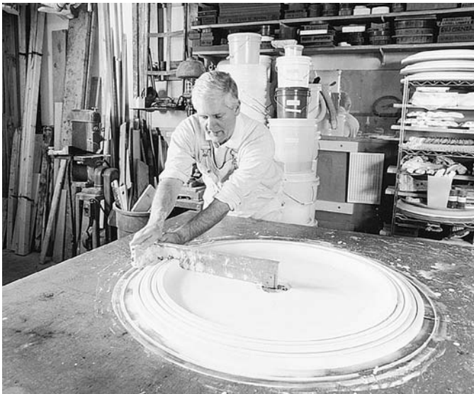
FIGURE C Sculptor David Flaharty runs a circular plaster medallion on a bench in his shop.
