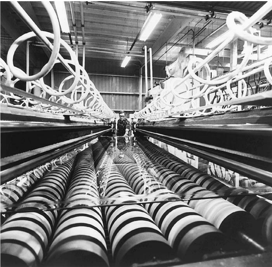
FIGURE 17.6 Track-mounted cutting devices score the ribbon of cooled float glass as part of a computer-controlled cutting operation that automatically produces the glass sizes ordered by customers. (Courtesy of PPG Industries)
