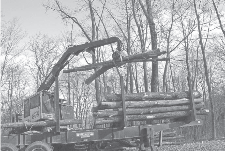
FIGURE 3.6 Loading logs onto a truck for their trip to the sawmill. (Photo by Donald K. O'Brien)
