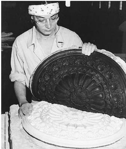
FIGURE A Removing the flexible rubber mold from a cast plaster ornament. (Courtesy of Dovetail, Inc.)
