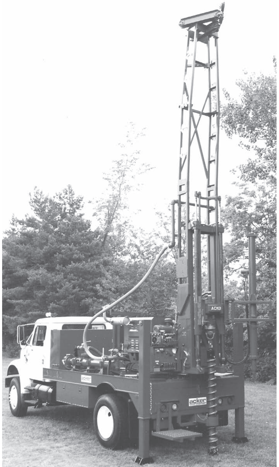
FIGURE 2.7 A truck-mounted drilling rig capable of core drilling to 1500 feet (450 m). (Courtesy of Acker Drilling Company, Inc.)
