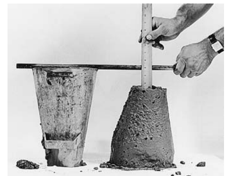
FIGURE 13.12 Photograph of slump being measured. (Reprinted with permission of the Portland Cement Association from Design and Control of Concrete Mixtures, 12th edition; Photos: Portland Cement Association, Skokie, IL)
