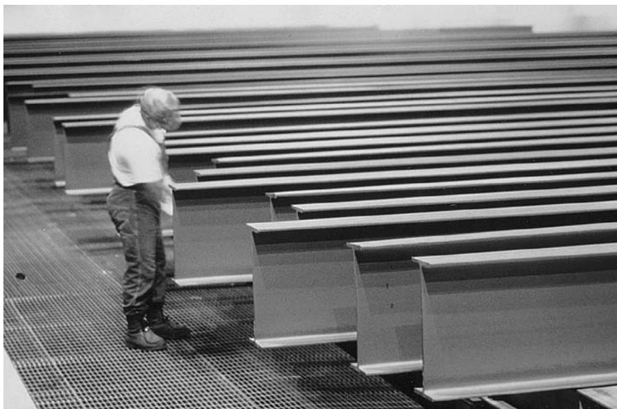
FIGURE 11.9 Wide-flange shapes are inspected for quality on the cooling bed. (Photo by Mike Engestrom. Courtesy of Nucor-Yamato Steel Company)
