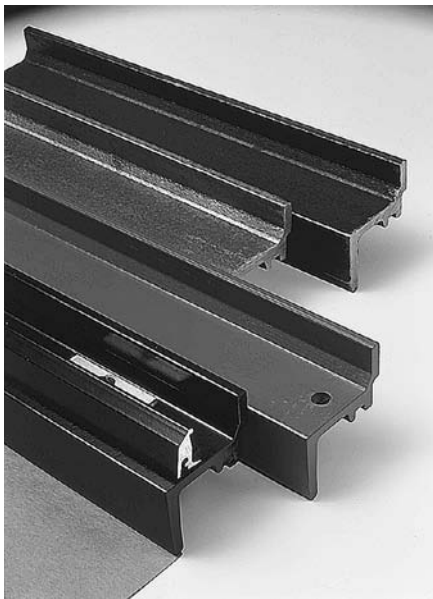
FIGURE 18.14 These samples of hot-rolled steel window frame sections demonstrate a range of permanent finishes. The nearest sample includes a snap-in aluminum bead for holding the glass in place. ( Steel windows by Hope's; photography by David Moog )
