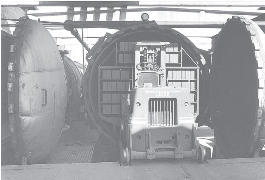
FIGURE 9.21 A forklift truck loads newly molded concrete masonry units into an autoclave for steam curing. (Reprinted with permission of the Portland Cement Association from Design and Control of Concrete Mixtures , 12th edition; photos: Portland Cement Association, Skokie, IL)
