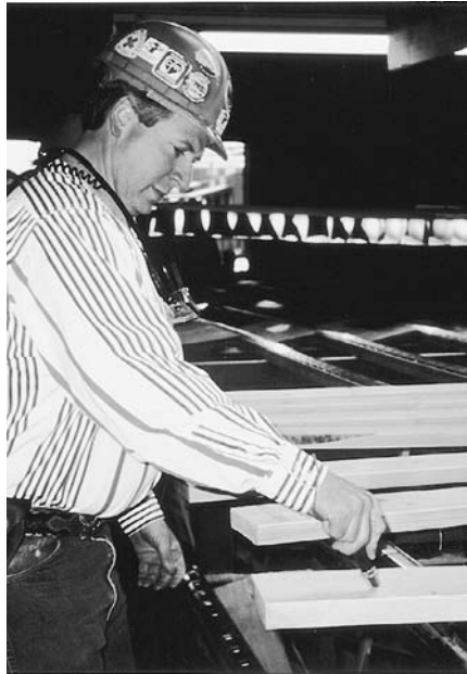
FIGURE 3.18 A grader marks the grade on a piece with a lumber crayon preparatory to applying a gradestamp. (Courtesy of Western Wood Products Association)
