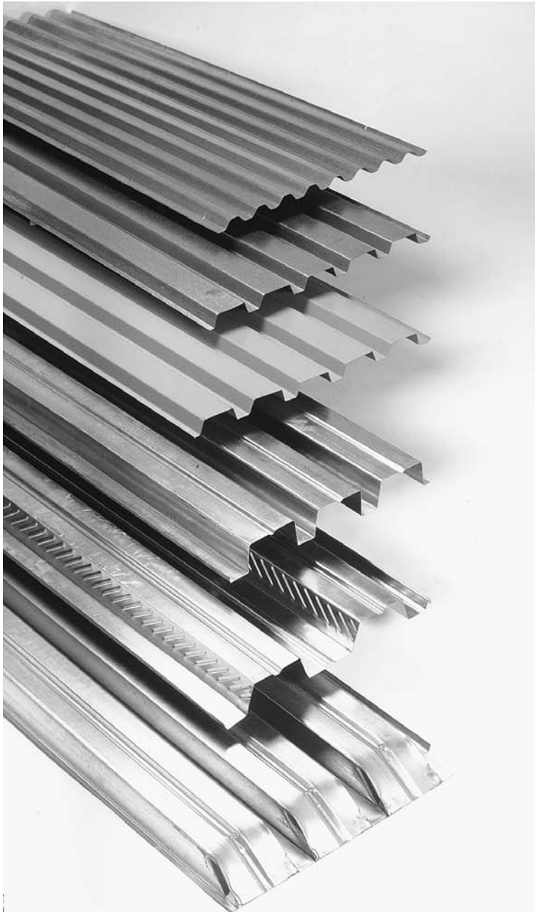
FIGURE 11.61 Samples of corrugated steel decking. The second sample from the bottom achieves composite action by keying of the concrete topping to the deformations in the decking. The bottom sample has a closed end, which is used at the perimeter of the building to prevent the concrete topping from escaping during pouring. (Courtesy of Wheeling Corrugating Company Division, Wheeling-Pittsburgh Steel Corp.)
