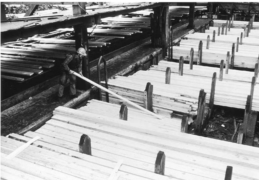
FIGURE 3.8 Sawn lumber is sorted into stacks according to its cross-sectional dimensions and length. (Courtesy of Western Wood Products Association)
