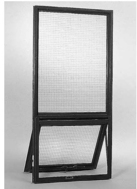
FIGURE 18.16 With fire-rated glazing such as wired glass, shown here, a steel window can be fire rated. This window features an awning sash below a fixed light. ( Steel windows by Hope's; photography by David Moog )
