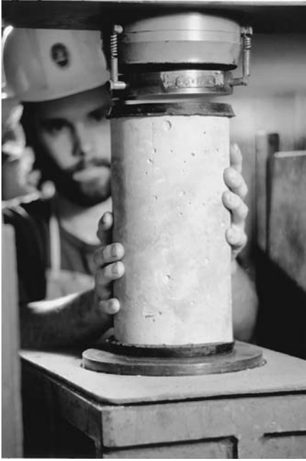
FIGURE 13.13 Inserting a standard concrete test cylinder into a structural testing machine, where it will be crushed to determine its strength. (Reprinted with permission of the Portland Cement Association from Design and Control of Concrete Mixtures, 12th edition ; Photos: Portland Cement Association, Skokie, IL)
