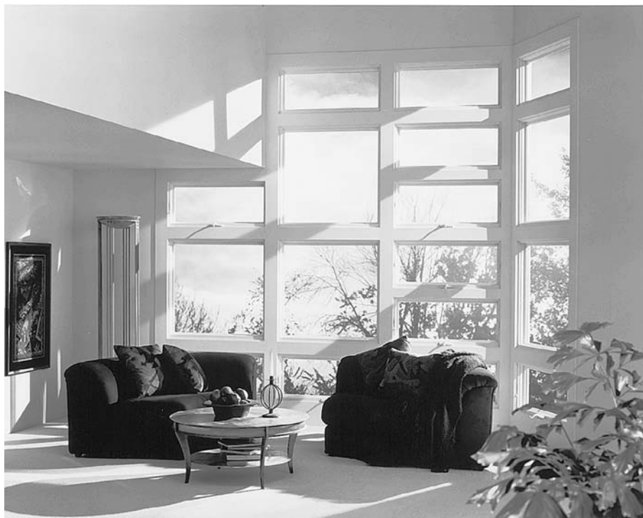
FIGURE 18.4 Awning and fixed windows in coordinated sizes offer the architect the possibility of creating patterned walls of glass. (Photo courtesy of Marvin Windows and Doors)
