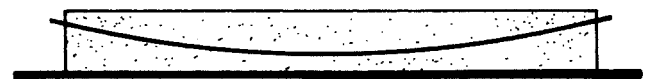
1. In posttensioning, the concrete is not allowed to bond to the steel strands during curing
