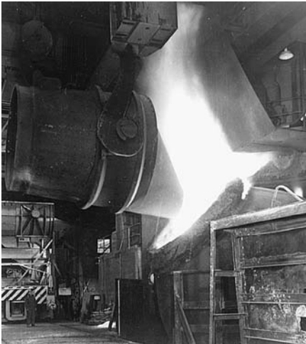
FIGURE 11.6 Molten iron is poured into a crucible to begin its conversion to steel in the basic oxygen process. (Courtesy of U.S. Steel Corp.)
