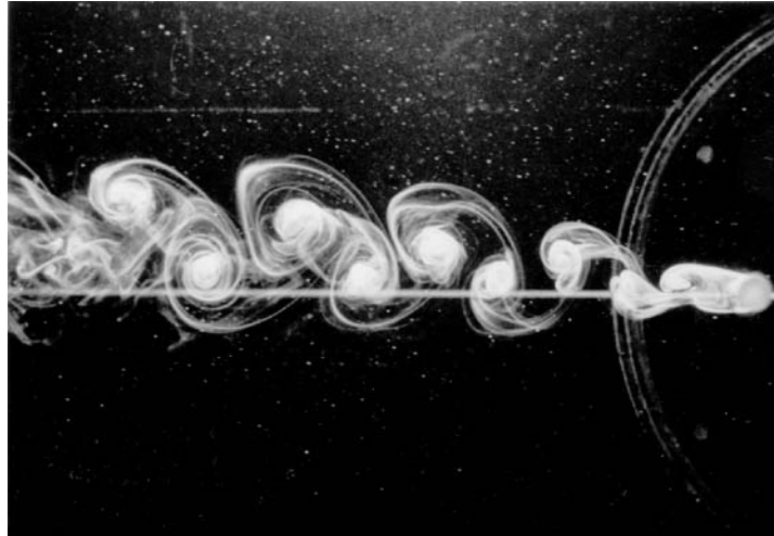
PLATE 3 Vortex street generated by a circular cylinder. (Photograph courtesy of the National Research Council of Canada.)
