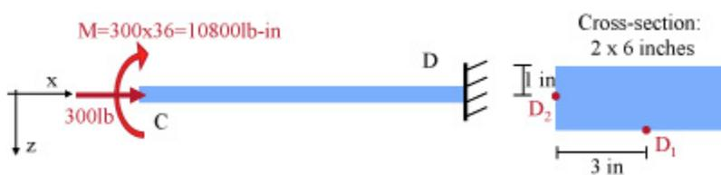
**Figure M-10** The beam in Figure M-9 can be reduced to the one shown here by moving the applied force at C, as typically done in statics.
