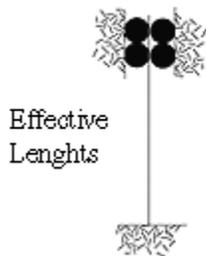
**Figure O-17** A cantilever column braced at the free end in the weak buckling direction.
