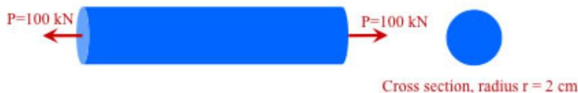
The maximum load this bar can sustain,  $P_{max}$ , is that load that creates a stress equal to the ultimate stress. Then,
