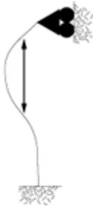
**Figure O-15** Mode I buckling of a fixed-pin column, and schematic designation of the effective length,  $0.7L$ .
