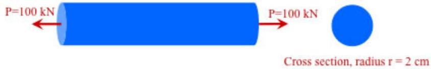
The stress on each cross section is:  $\sigma = \frac{P}{A} = \frac{100\text{kN}}{\pi(0.02)^2} = 79,577.5 \text{ kPa}$
