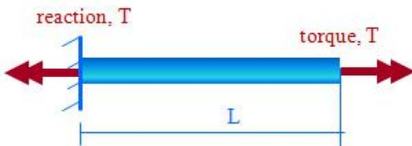
**Figure F-4** Free body diagram of a shaft
