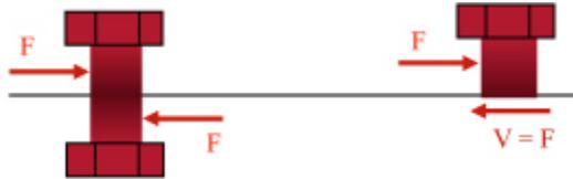
The shear force  $V$  is equilibrated by the internal shear stresses acting on the cross section.
