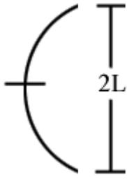
**Figure O-13** Mode I buckling shape of a cantilever beam of length  $L$ , and its mirror image.
