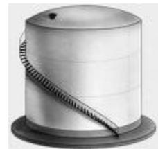
**Pressure Tanks: 8** A cylindrical pressure tank is constructed by welding together sheet metal at angle  $\phi$  as shown. Two options are considered, one for  $\phi = 30^\circ$  and one for  $\phi = 50^\circ$ . Which of the two is more efficient, with respect to creating the least shear stress on the weld.
