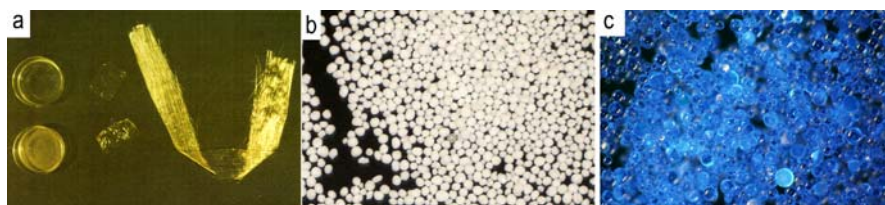
Fig. 15 Optical images of DNA-based materials for environmental purpose. a DNA–alginate hybrid matrix coagulated by \text{Ca}^{2+} , in fiber, film, and gel form. b DNA-immobilized porous glass beads prepared by UV-irradiation. c DNA–polyacrylamide hydrogel beads synthesized by inverse suspension polymerization
