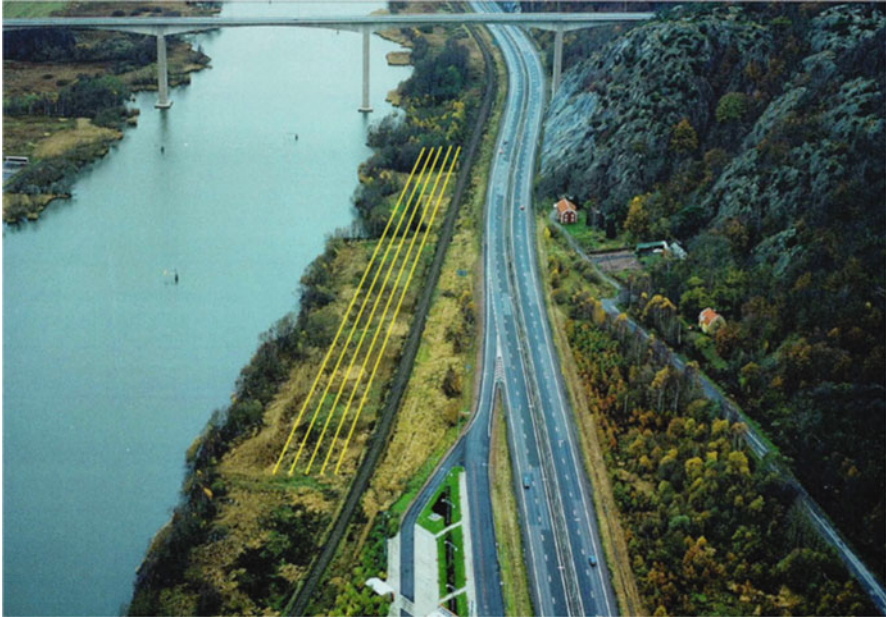
Fig. 17.2 Aerial photograph overlooking the investigation site from the south. The approximate locations of the ERT profiles (400 m long and 5 m apart) have been indicated in yellow (Photograph provided by the BViV project organization)
