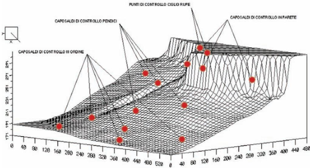
Fig. 22.16 Schemes of geotechnical monitoring net in Orvieto
