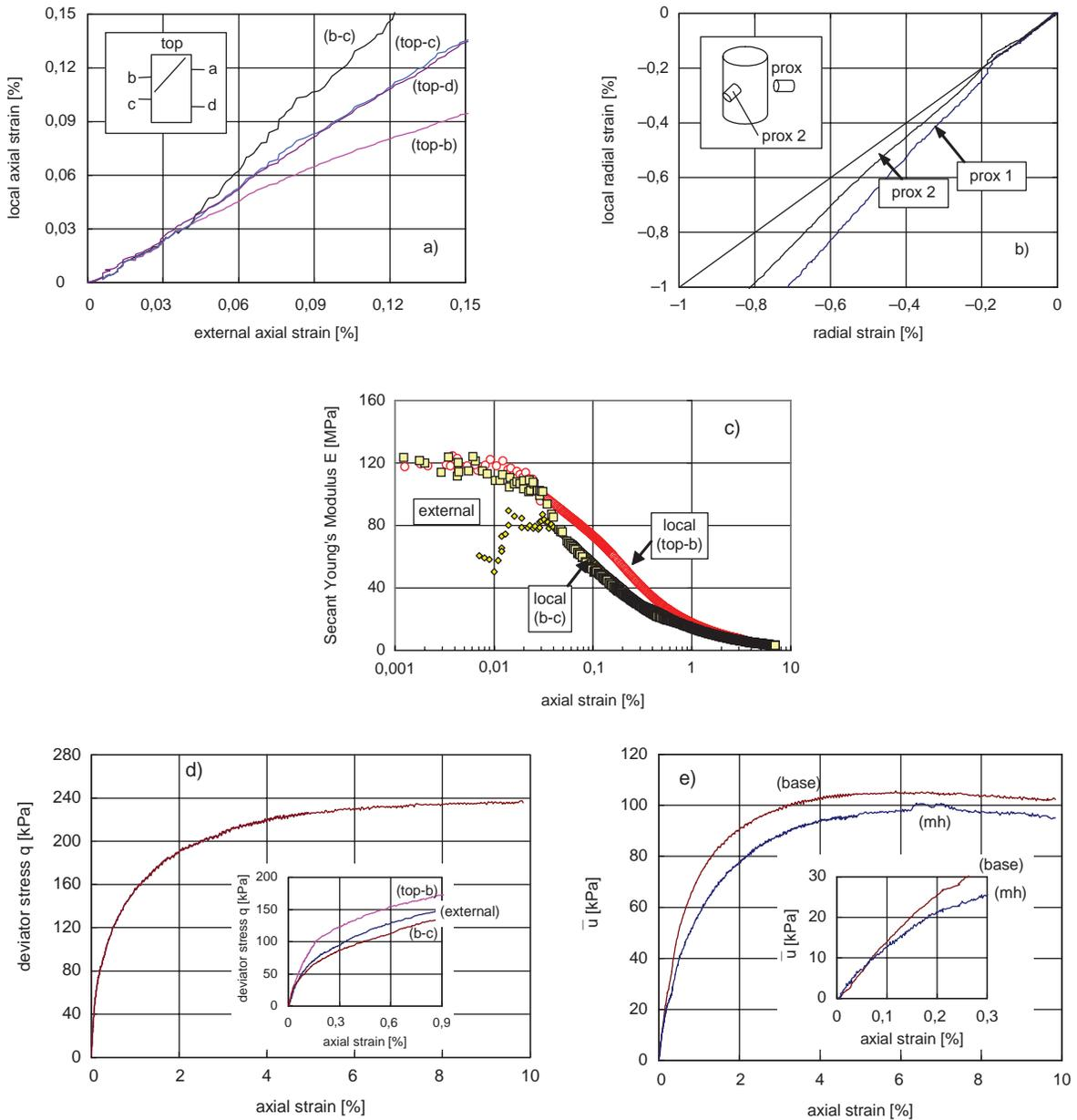
**Fig. 4.2** Results of an undrained triaxial test on the Bisaccia clay subjected to a confining stress of 400 kPa (Olivares, 1998): (a) local axial strains; (b) local radial strains; (c) secant Young modulus; (d) stress-strain curve; (e) local excess pore pressures
