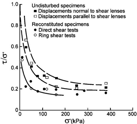
**Fig. 4.4** Residual strength of the Laviano highly fissured clay shale (Picarelli, 1980)
