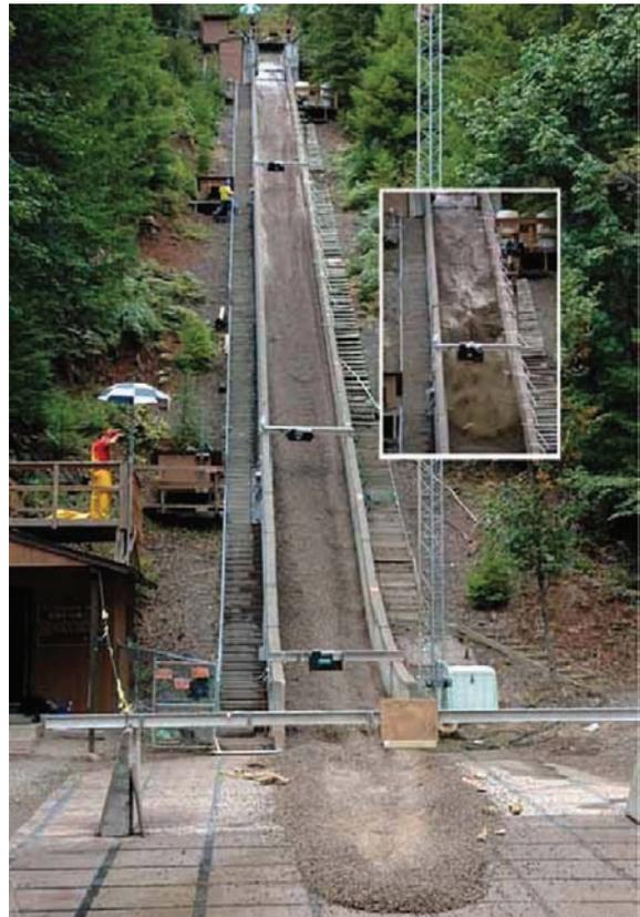
**Fig. 24.4** An completed debris flow experiment at the U.S. Geological Survey flume located in the H.J. Andrews Experimental Forest, Oregon (USA). The inset shows a debris flow moving down the flume. (Photograph from Logan and Iverson, 2007)
