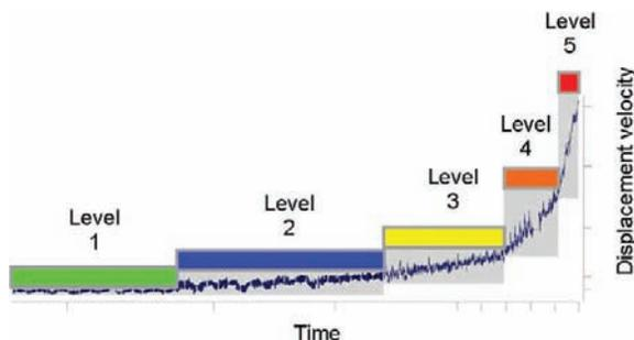
**Fig. 3.17** Illustration of the alarm levels as function of displacement velocities (*vertical axis*: displacement rate in mm/day; *horizontal axis*: relative time before failure)
