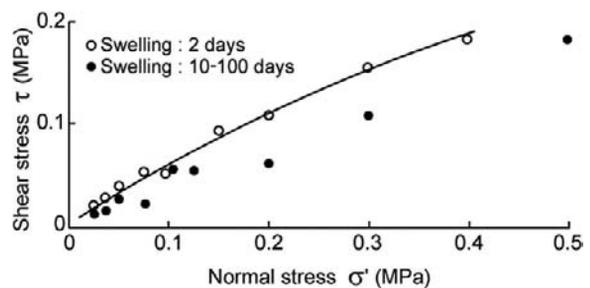
**Fig. 4.8** Results of direct shear tests on the Bisaccia clay shale for normal stresses lower than the swelling pressure and after a different swelling time (Picarelli, 1986)
