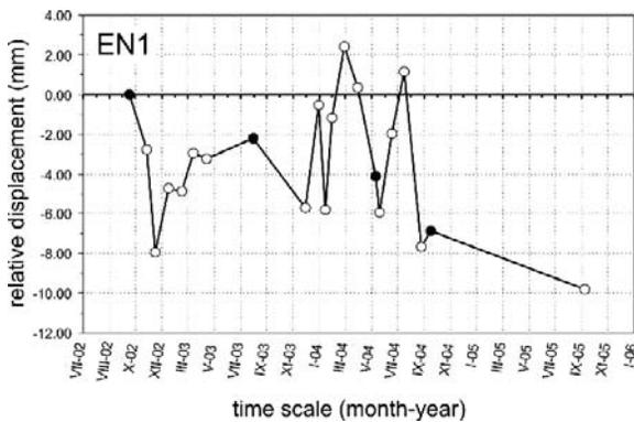
**Fig. 15.5** The graph of extensometric measurement at the site EN1 – Plaza North. (Black points are our control measurements, in white colour are presented measurements done by INC)
