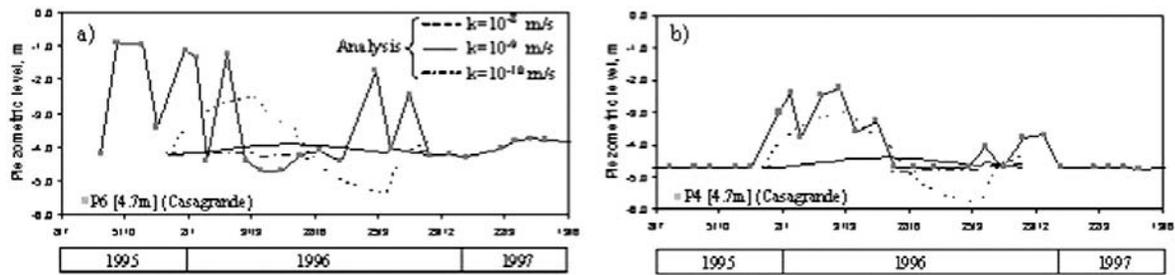
Fig. 4.25 Measured and calculated water levels in the piezometers P6 and P4 (Comegna et al., 2007)
