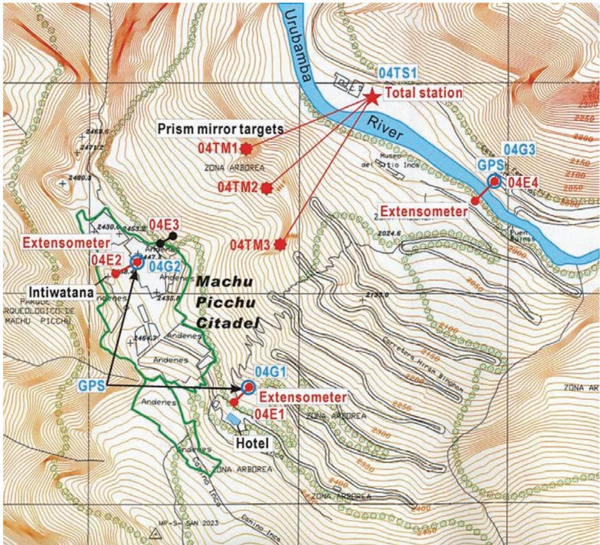
**Fig. 13.13** Location of extensometers, GPS and Total Station
