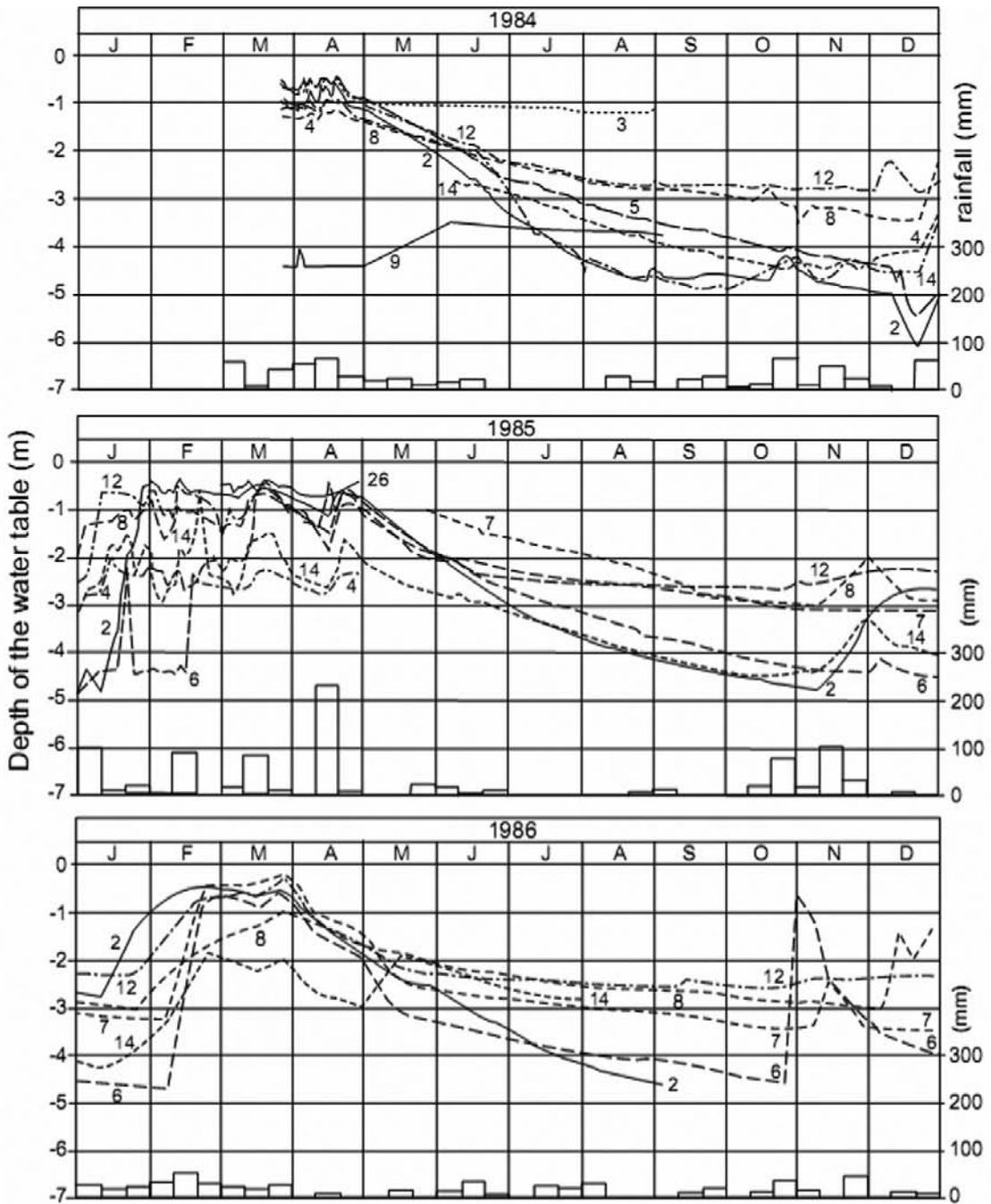
Fig. 4.22 Water level readings at standpipe piezometers (Picarelli and Viggiani, 1988)
