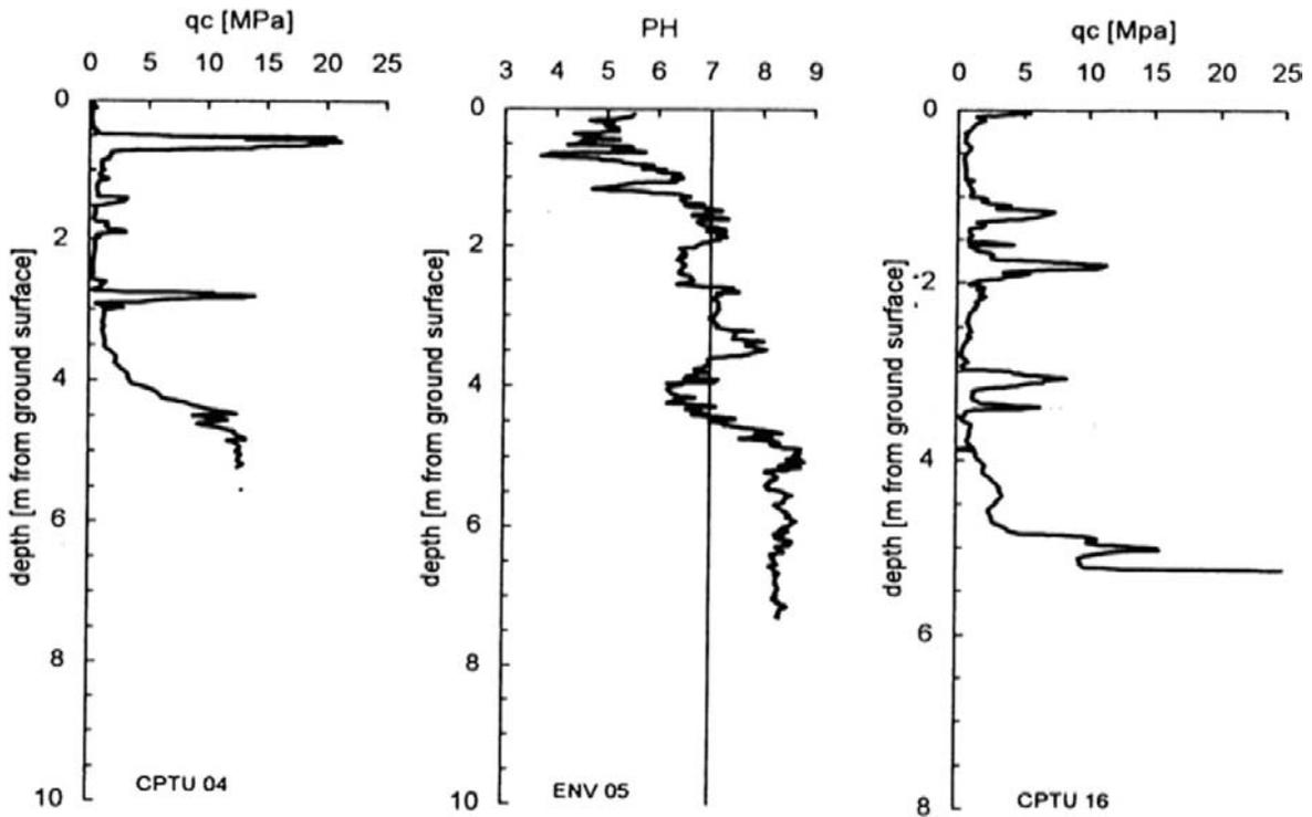
**Fig. 4.13** Results of CPTU and environmental cone tests along two cross sections in a mudslide in the Bisaccia clay shale (Picarelli et al., 1998)
