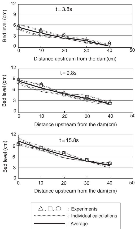
**Fig. 5.10** Experimental and calculated bed levels behind the dam at different times
