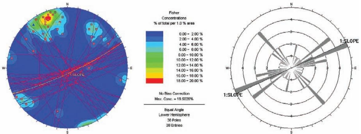
**Fig. 22.25** Joints orientation sets of the W part of Bamiyan cliff (stations 1–10) represented through stereonet (left) and rose diagram (right)
