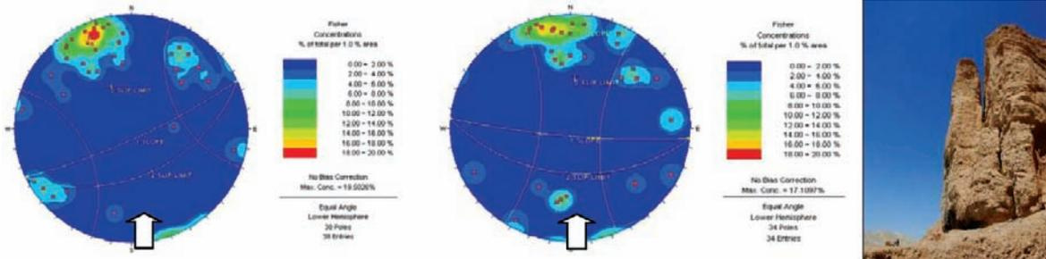
**Fig. 22.27** Results of kinematic analysis for toppling for W side (left) and E side of the cliff (middle); the arrows show the region where toppling is possible (between slip limit and lower stereonet border). Toppling evolution in the cliff (right)
