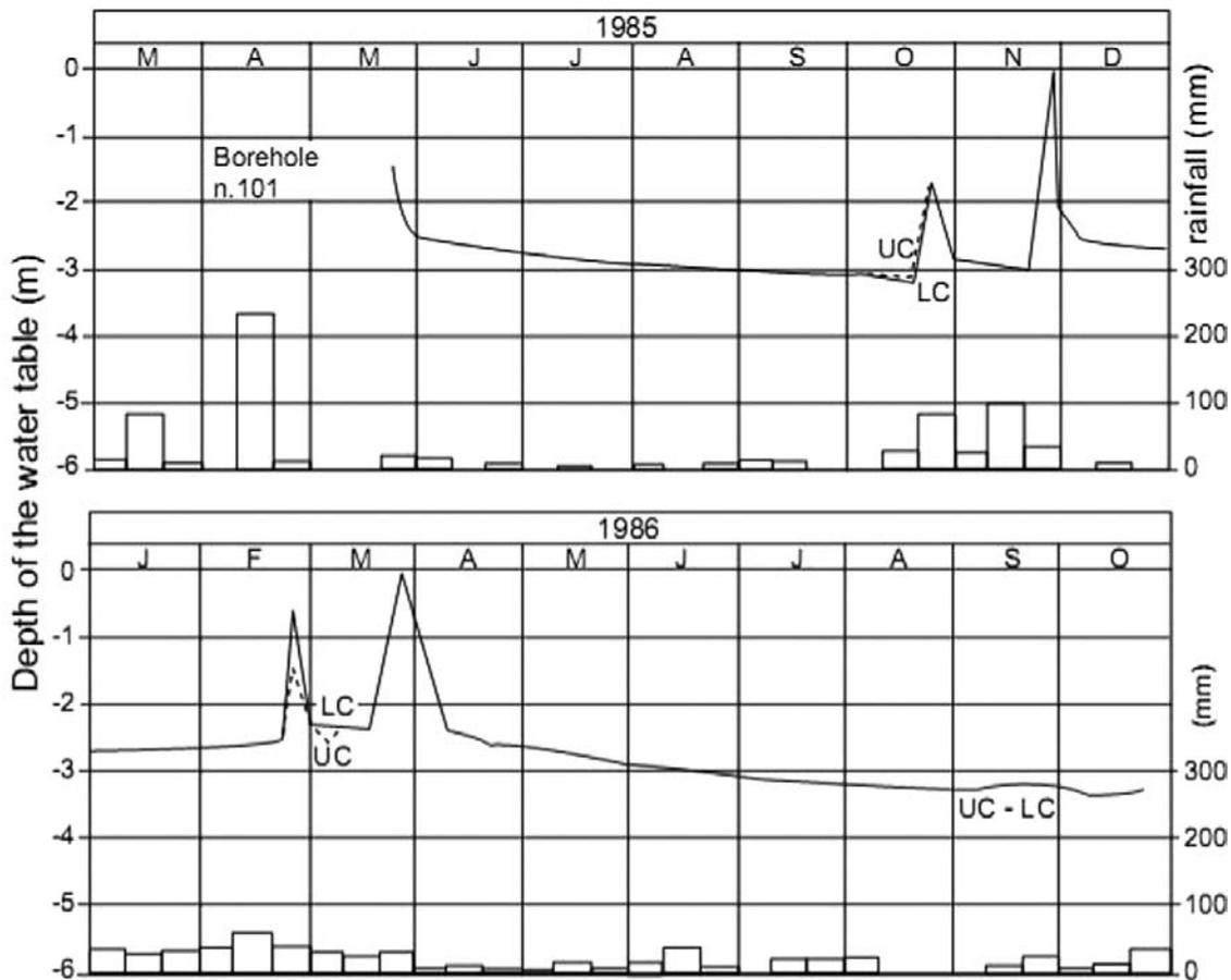
Fig. 4.23 Water level readings at the Casagrande piezometers no 101 (Picarelli and Viggiani, 1988)
