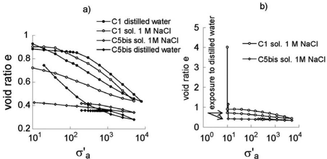
**Fig. 4.11** Results of oedometer tests on undisturbed specimens exposed to different liquids (from Picarelli et al., 1998)
