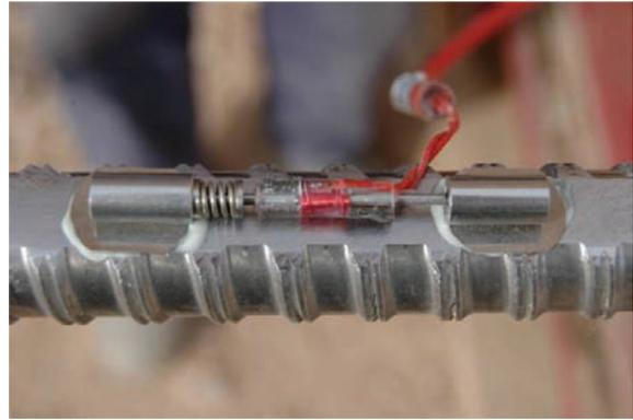
**Fig. 10.31** Detail of a strain gauge
