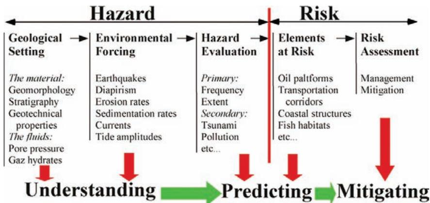
**Fig. 6.29** General framework for risk assessment for submarine slides (from Nadim and Locat 2005)
