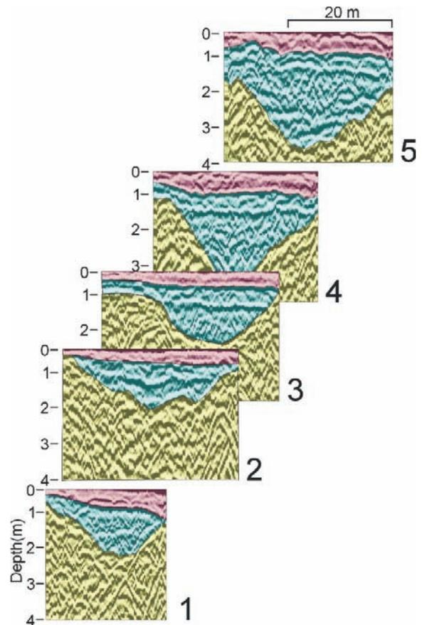
**Fig. 16.6** Interpretation of the parallel radar profiles across the Planza in Machu Picchu
