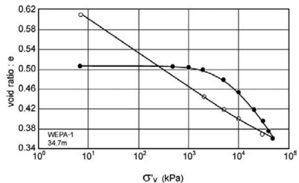
**Fig. 4.6** Results of a one-dimensional compression test on the Culebra clay shale (Banks et al., 1975)
