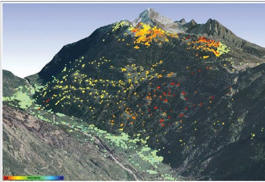
**Fig. 7.9** PSInSAR monitoring of Mount Padrio (Ferretti et al. 2005)
