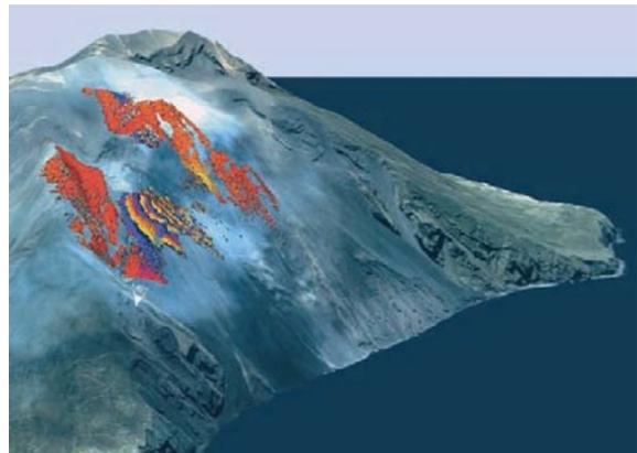
**Fig. 23.7** 3D model of the Stromboli Island (Sciara del Fuoco slope and NE crater) with an interferogram obtained from the GB-InSAR. The position of the radar is shown with the white symbol. The interferogram spans a time interval of 11 min (from 11.17 UT to 11.28 UT of 9 March 2007) showing a velocity greater than 300 mm/h
