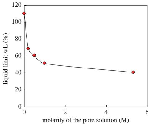
**Fig. 4.9** Dependence of the liquidity limit of the Bisaccia clay shale on the nature of the pore liquid (from Picarelli et al., 1998)
