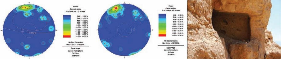
**Fig. 22.28** Results of kinematic analysis for planar sliding for W side (left) and E side of the cliff (middle). Planar rockslide involving an ancient cavity (right)
