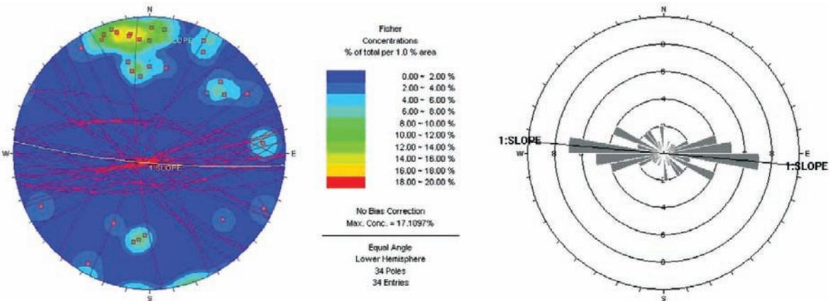
**Fig. 22.26** Joints orientation sets of the E part of Bamiyan cliff (stations 11–17) represented through stereonet (left) and rose diagram (right)
