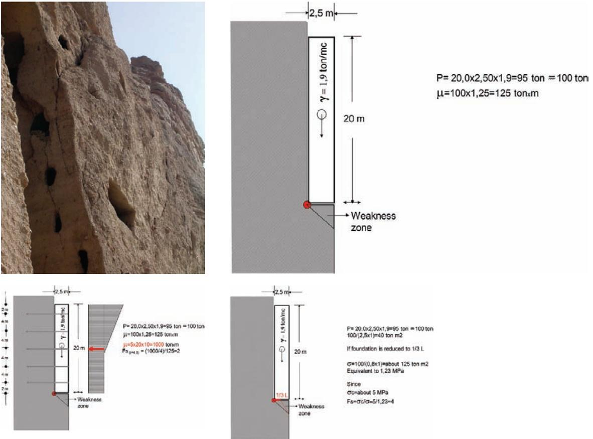
**Fig. 10.14** The external block prone to collapse, the geometrical distribution of load and the assumption for calculation, moment calculation of anchors and the related factor of
