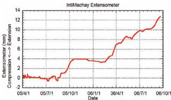
**Fig. 13.16** Monitored record of extensometer (04E3) installed in IntiMachay below the Plaza
