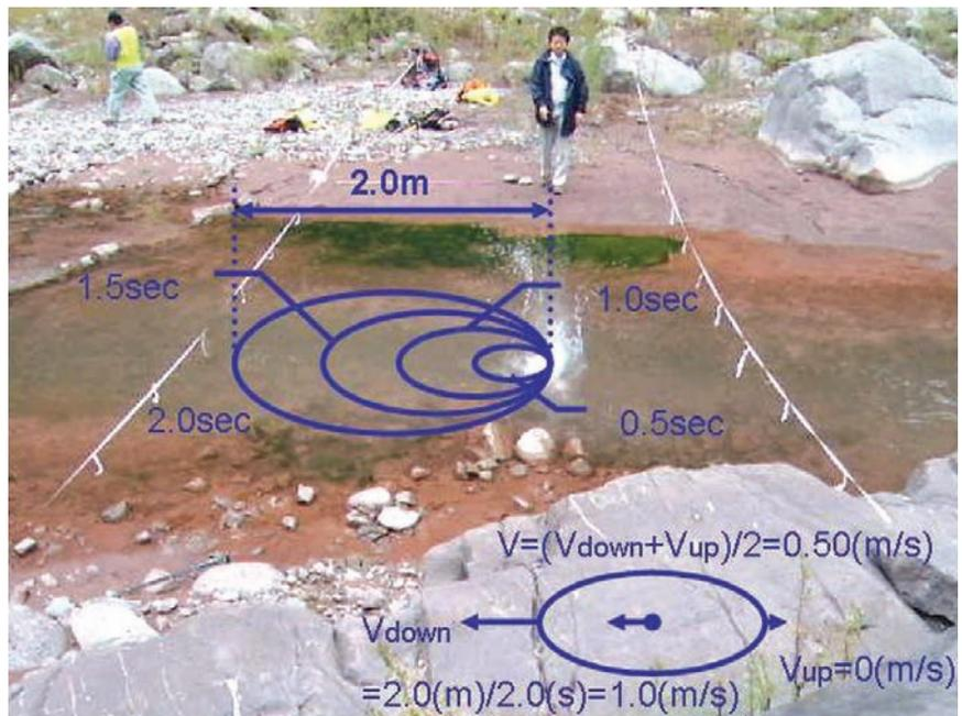
**Fig. 8.4** Measurement of discharge seeping out from the toe of the avalanche mass
