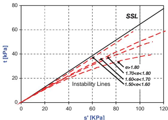
**Fig. 4.14** Instability Lines of a loose volcanic ash (Lampitiello, 2004)
