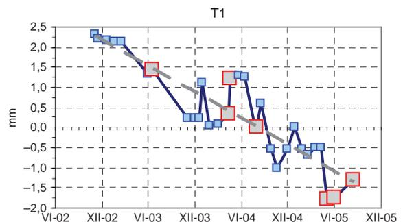
**Fig. 15.4** The graph of dilatometric measurement at the locality T - Temple. The site T1 is on the east face of the block located. (Red points are our controle measurements, blue ones were measured by our Peruvian partners from INC)
