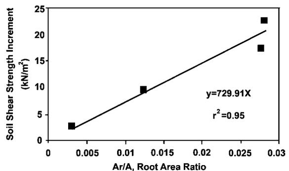
**Fig. 33.7** The effect of tree roots area on the increment shear strength of soil (source: Shafaei Bajestsn M. and Salimi Golsheikhi, M. 2002)
