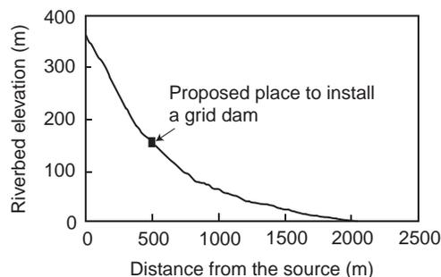
**Fig. 5.12** The longitudinal profile of the river and the position at which a grid dam will be installed
