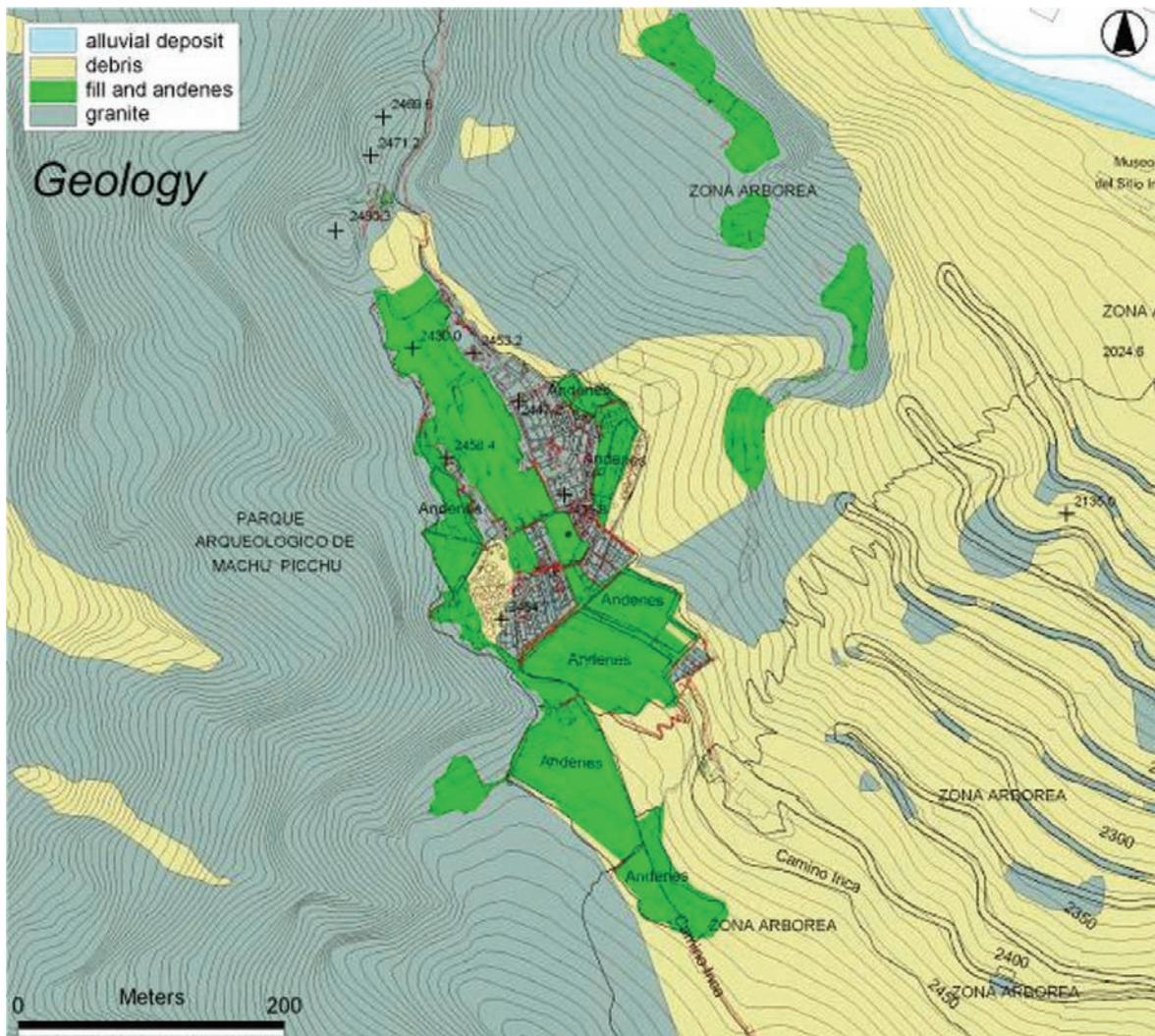
**Fig. 22.11** Sketch of local geological map of the Inca citadel of Machu Picchu (by Canuti et al., 2005)
