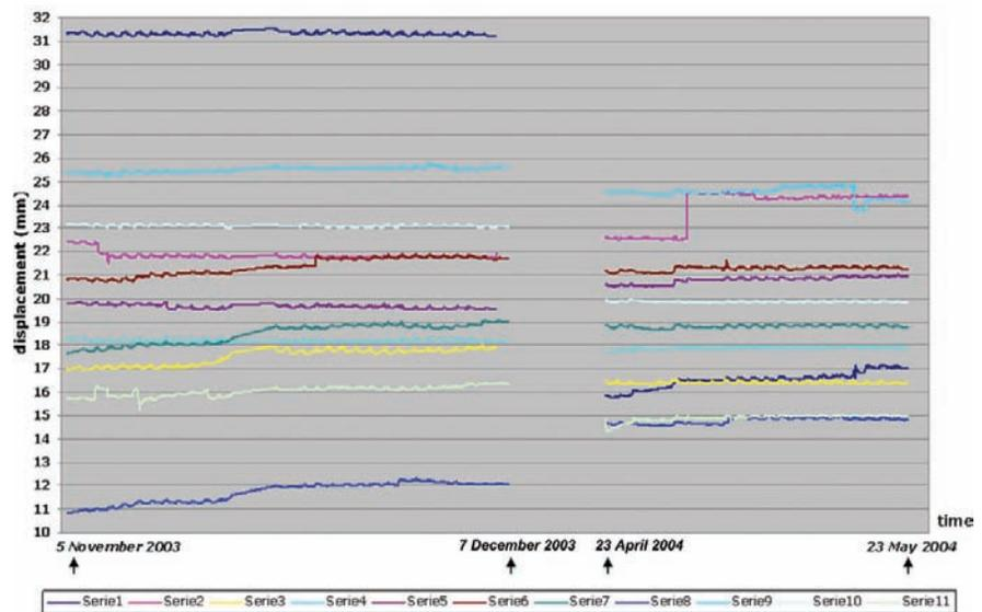
**Fig. 10.23** Time evolution of the 11 extensometers operating in the period 5th November – 7th December 2003 and 23 April – 23 May 2004 in the Eastern wall of the niche, and showing no remarkable movements on the cliff. Some minor step have been caused by climbers, who hit the gauge placed on the cliff
