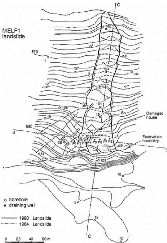
**Fig. 4.20** The Melfi landslide and piezometers installed in the landslide area (Picarelli and Viggiani, 1988)
