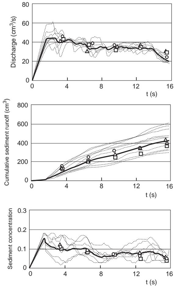
**Fig. 5.11** Calculated and experimental hydrographs, cumulative sediment runoff and sediment concentrations just downstream of the dam
