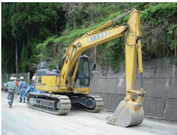
**Fig. 32.9** Backhoe operated by Unmanned Construction System (UCS). Robot arm and surveying camera are set at the operating location. Operator remotely controls the machine by the robot arm and camera
