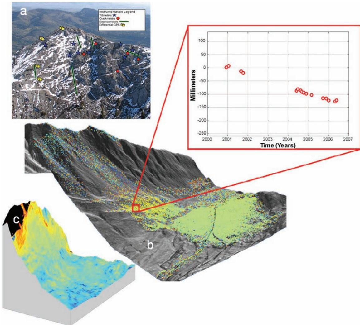
**Fig. 7.5** InSAR monitoring of Frank slide, Canada, modified from Mei et al., 2007
