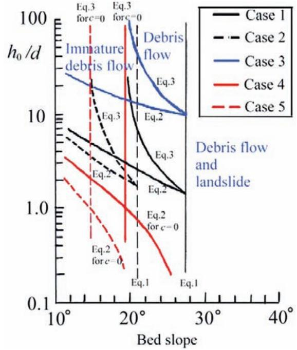
**Fig. 5.3** The occurrence criteria of debris flows and immature debris flows
