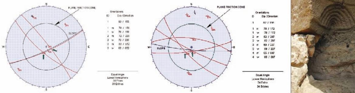
**Fig. 22.29** Results of kinematic analysis for wedge failure for W side (left) and E side of the cliff (middle); the arrows show the intersections of planes that may cause sliding inside the potential area (crescent shaped region between slope limit and lower friction cone). Potential wedge sliding along the cliff (right)
