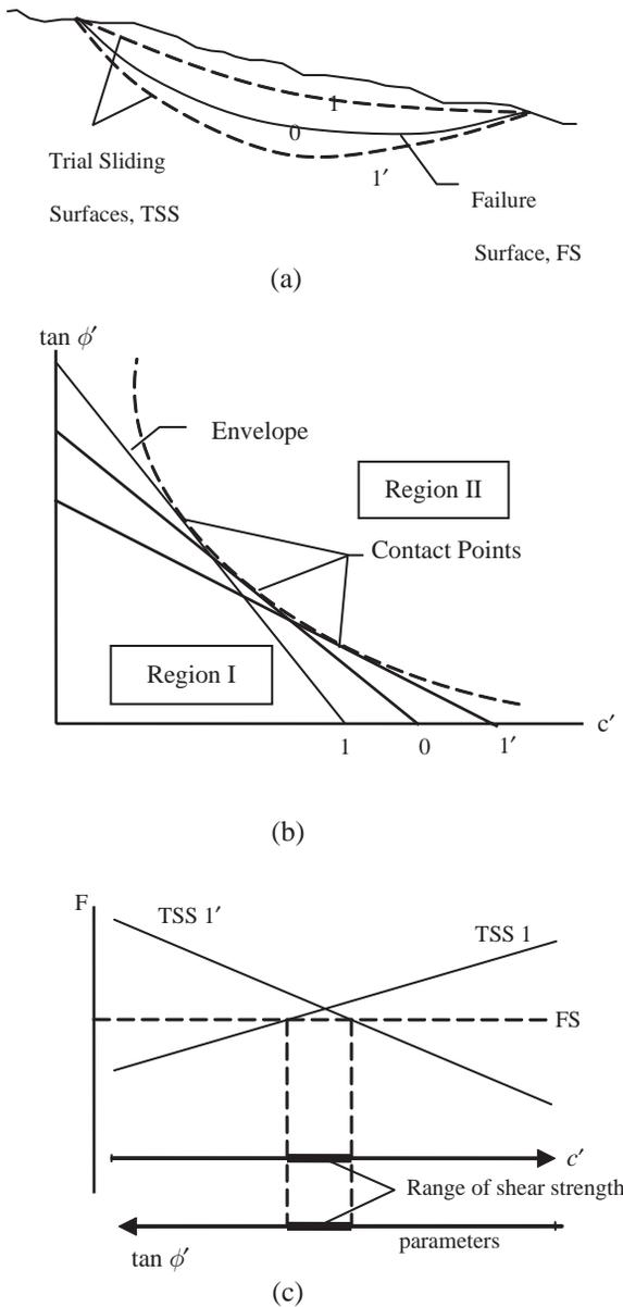
**Fig. 32.11** Back Calculation of the Shear Strength Parameters from Slope Failures. The two unknowns ( $c'$  and  $\phi'$ ) can be simultaneously determined from the following two equations involving the slope safety factor:  $F=1$  and  $F=\text{minimum}$
