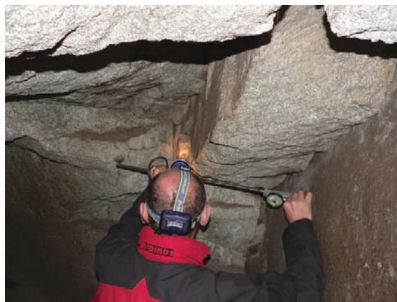
**Fig. 15.2** An example of dilatometric measurement – locality W (Wayna Picchu). Visitors are allowed to enter this area, thus the measurement is needed here
