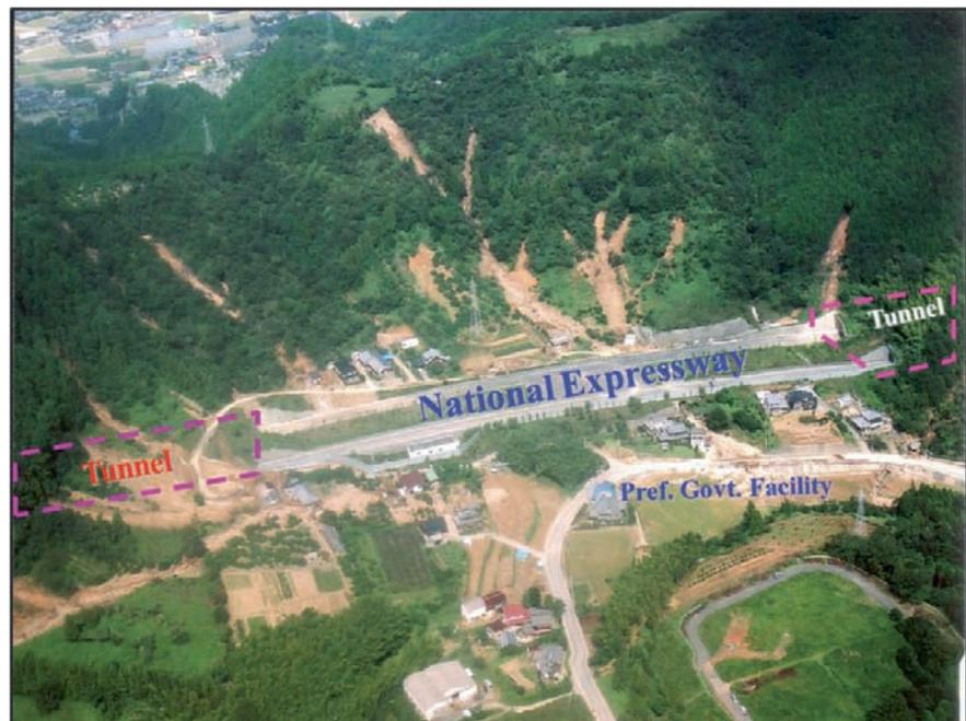
**Fig. 26.1** Widespread landslide in Saijo covering the tunnel and national expressway
