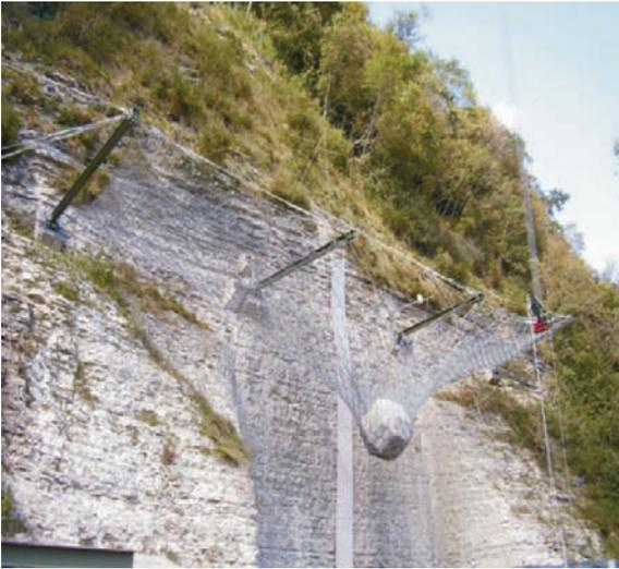
**Fig. 32.16** Full Scale Modeling of the Behavior of the Rockfall Protection Fences: Rock blocks of different sizes are dropped vertically onto the protection net to assess its deformation and breaking time
