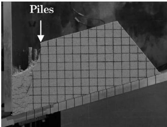
**Fig. 32.18** Slope Condition after the Centrifugal Loading Experiment: Slope failure occurred around the piles inserted into the slope
