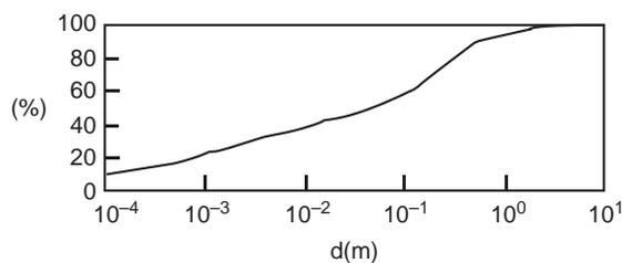
**Fig. 5.13** Particle size distributions in the riverbed
