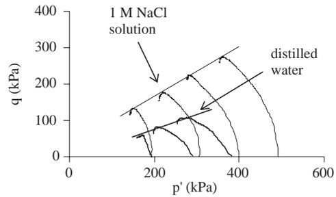
**Fig. 4.10** Comparison of the failure envelopes of reconstituted Bisaccia clay mixed with distilled water and with a NaCl solution (from Di Maio and Onorati, 2000)
