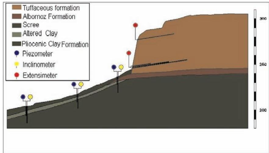
Fig. 22.17 Geology of Orvieto cliff and the monitoring net
