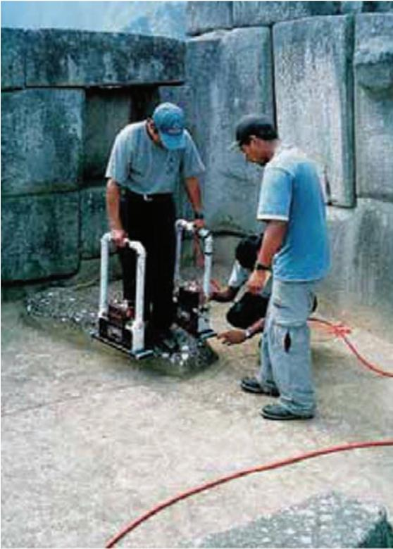
**Fig. 16.5** Sensors, 200 MHz transmitter and receiving antenna assemblies of GPR in Machu Picchu
