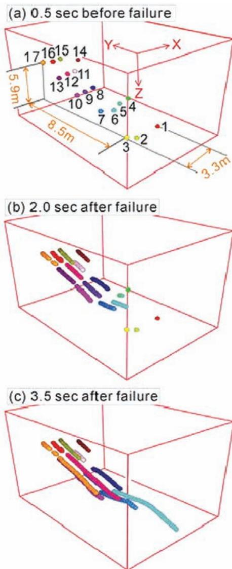
**Fig. 24.12** Snapshots of the three-dimensional movements of the targets. (a) 0.5 second before failure (24 627 s), (b) 2 seconds after failure (24 929.5 s), and (c) 3.5 seconds after failure (24 631 s)
