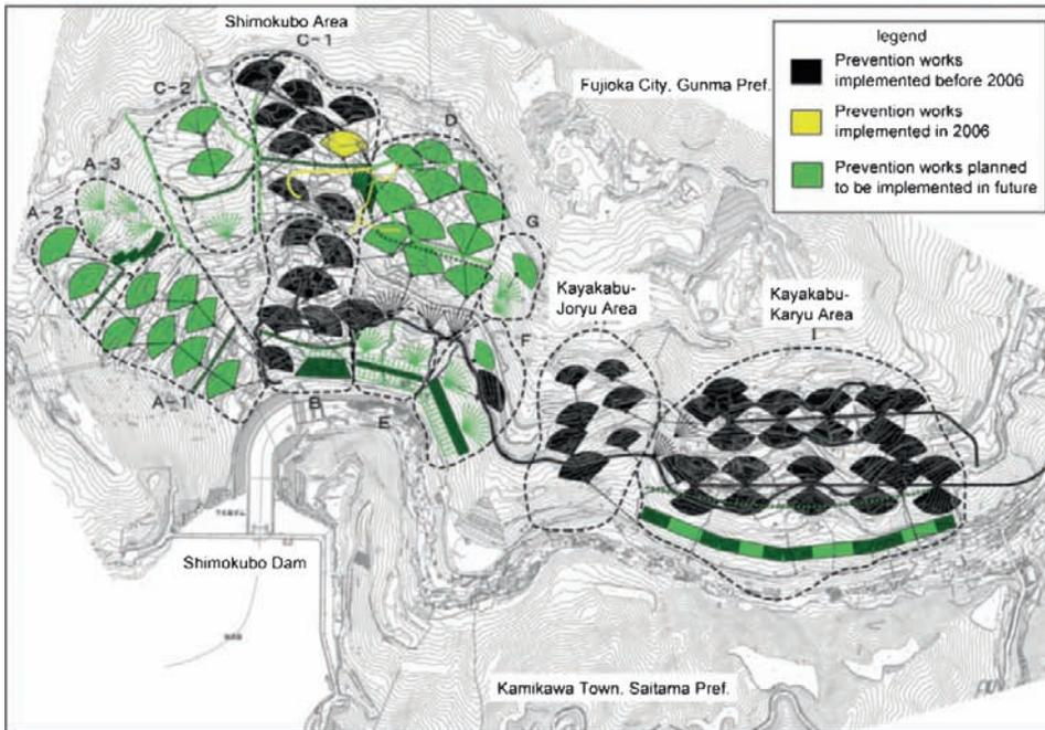
**Fig. 32.17** Yuzurihara Landslide, Japan: Landslide area comprising several blocks (*upper*). Map of the mitigation
