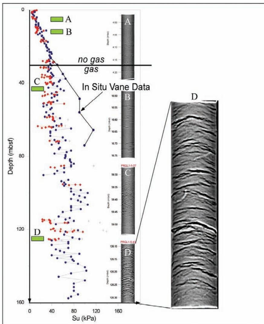
**Fig. 6.30** PRGL1-5 CAT-Scan images and undrained shear strength profile for PRGL1-5: example of a strength profile obtained from in-situ testing and laboratory tests on samples from a Gulf of Lions site. (PRGL1: Borehole name in the Gulf of Lions). Green bars indicate position of samples used for CATSCAN analysis, mbsf: metres below sea floor
