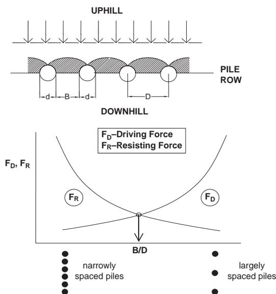
**Fig. 32.12** Design of Piles to Stabilize Landslides. Both driving and resisting force acting on each pile in a row should be considered to derive the optimum non-dimensional pile interval ratio  $B/D$
