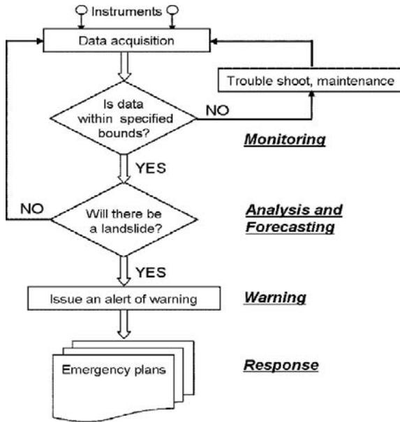
**Fig. 3.11** Block diagram of a typical early warning system (DiBiagio and Kjekstad 2007)
