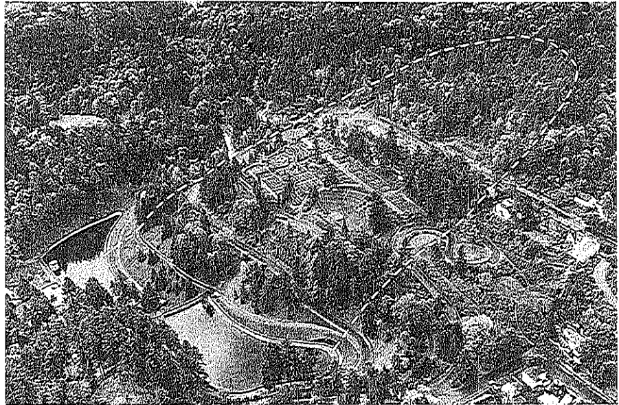
Figure CH-1.1 Washington Park Reservoirs Slide. The two reservoirs are at the lower left, and the outline of the 1700-foot long landslide is shown by the broken white line.
