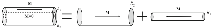
Fig. 6.33 The hollow magnetized cylinder behaves like two massive bars of radius R_1 and R_2 , respectively, whose magnetizations are in opposite directions
