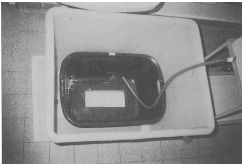
Fig. 1) Scald burn injury model (waterboiler, connection tube, bath, basket with cut out piece)
