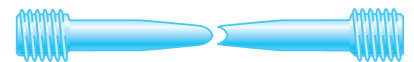
FIG. 2.6 Failed tensile test specimen showing necking, or narrowing, of the cross section.
