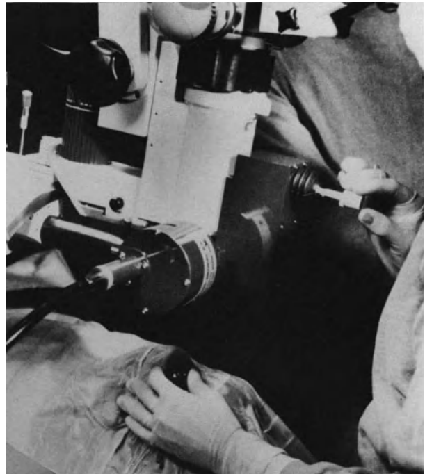
Figure 20. Instrumentation for intraoperative argon laser photocoagulation. Attachment of the biophysical medical argon laser to the Zeiss OPMI 6 microscope.
