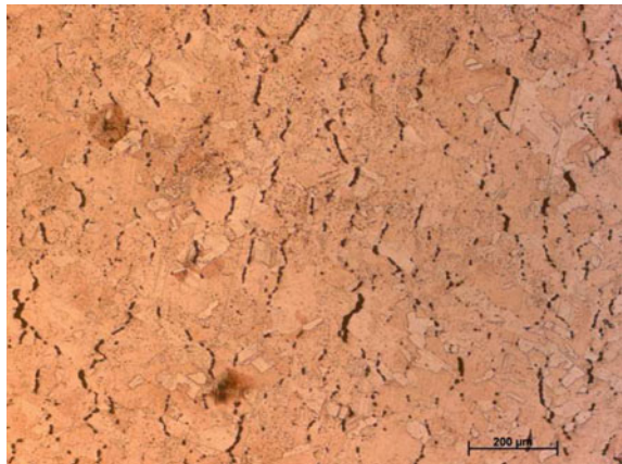
Fig. 12.28 Micrograph of copper specimen tested 20 h under constant stress of 10 MPa (stress direction horizontal ) and temperature level of 550 °C (Ozhoga-Maslovskaja 2014)
