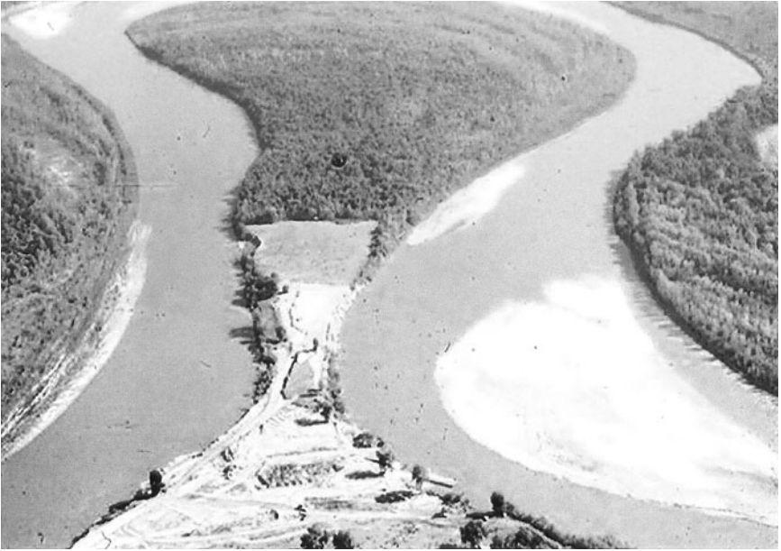
Fig. 4-4. Impending natural channel realignment or cutoff Source: USACE Vicksburg District
