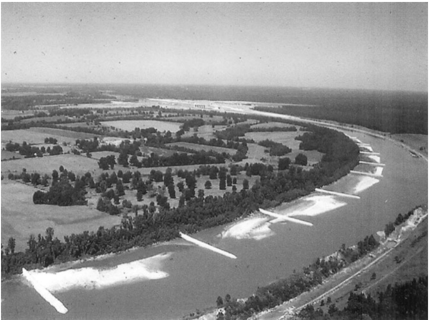
Fig. 4-3. Additional contraction structures Source: USACE Vicksburg District
