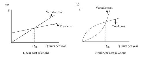
*Figure 31.10* Linear and nonlinear breakeven graphs.
