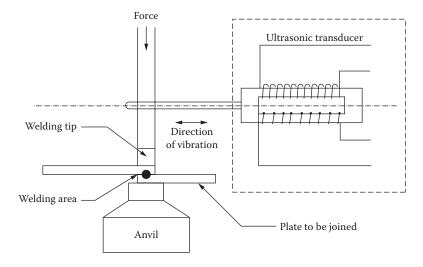
Figure 19.14 Ultrasonic welding (solid state).
