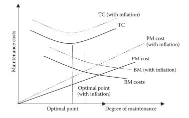
*Figure 41.2* Maintenance costs (including total, preventive, and breakdown). *Note*: preventive maintenance – PM; breakdown maintenance – BM; and total cost – TC.
