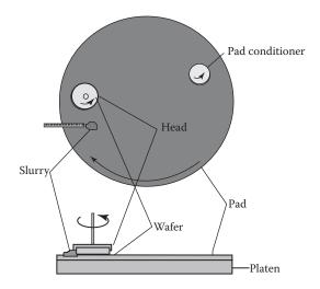
Figure 42.4 Schematic of a CMP system.
