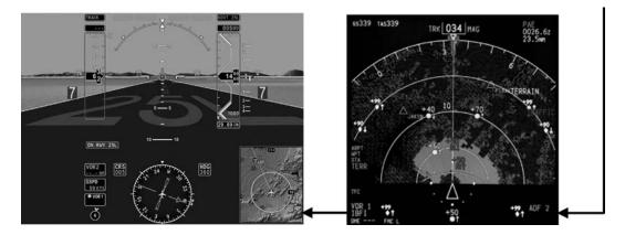
*Figure* 26.5 Heading indicator via the Integrated Primary Flight Display (IPFD) and TCAS. (Courtesy of Honeywell International Inc.)
