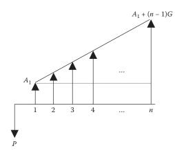
Figure 31.6 Arithmetic gradient cash flow with nonzero base amount.
