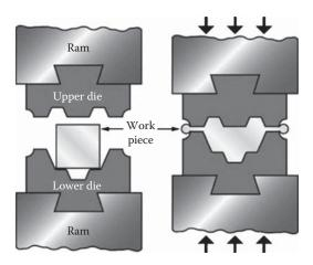
Figure 21.5 Open-die forging (CES Edupack, 2012).
