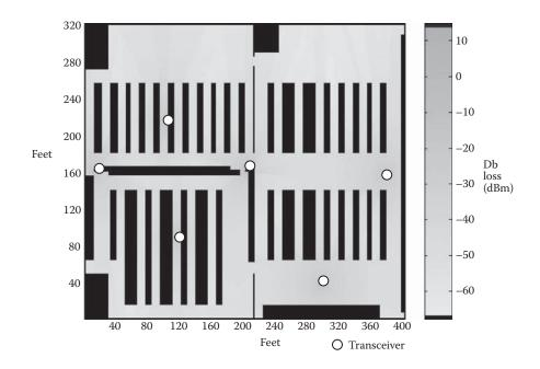
*Figure 36.12* Overlay of site survey results on a warehouse layout.
