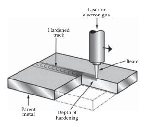
Figure 21.31 Laser surface hardening and melting (CES Edupack, 2012).
