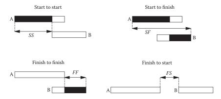
Figure 52.10 Lead-lag relationships in precedence diagramming (from Badiru and Pulat, 1995).
