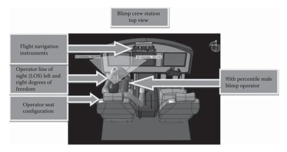
*Figure 26.6* Crew station human modeling (operator vision, display, seat, and rudder evaluation). National Institute of Aviation Research (NIAR).
