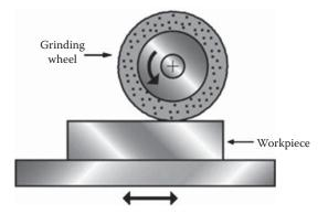
*Figure 21.16* Grinding—used for finishing in general or machining hard materials (CES Edupack, 2012).
