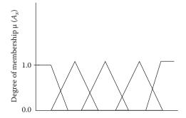
Figure 51.8 Triangular shaped membership function with trapezoidal shoulders.
