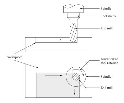
Figure 19.8 End milling.
