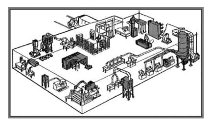
Figure 45.3 Examples of local exhaust ventilation systems.
