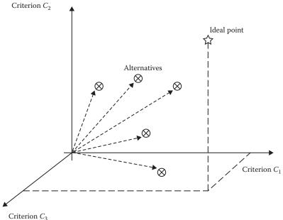
Figure 35.6 Illustration of compromise programming.
