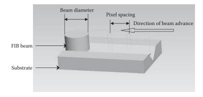
Figure 17.1 Schematic of FIB milling.
