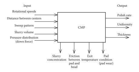
*Figure* **42.5** CMP process inputs and outputs.
