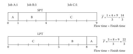
*Figure 53.1* Optimality of SPT for min  $\overline{F}$  (single machine Gantt charts comparing optimal with nonoptimal).
