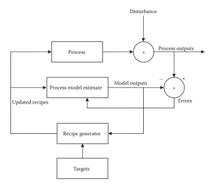
Figure 42.3 Structure of run-to-run controller.
