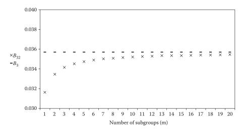
*Figure* **43.3**  $B_{32}$  and  $B_3$  for  $\alpha = 0.001$  below LCL and n = 3.
