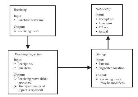
Figure 36.7 Current receiving process flow diagram.
