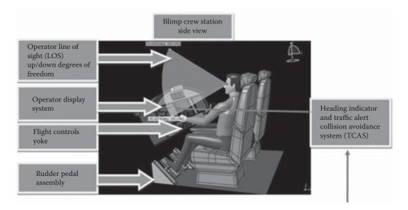
*Figure 26.4* Crew station human modeling (operator vision, display, seat, and rudder evaluation). National Institute of Aviation Research (NIAR).
