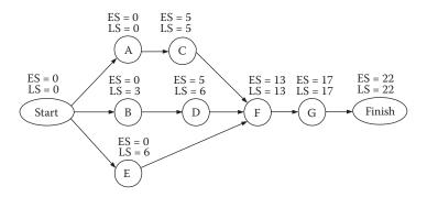
Figure 52.25 AON network for the example project.
