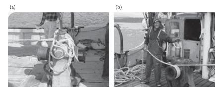
*Figure 45.8* PtD solution for fishing vessel. (a) Captan-type winch with fishing lines wound around. (b) Fishing captain demonstrating use of an emergency-stop (e-stop) mounted on winch.
