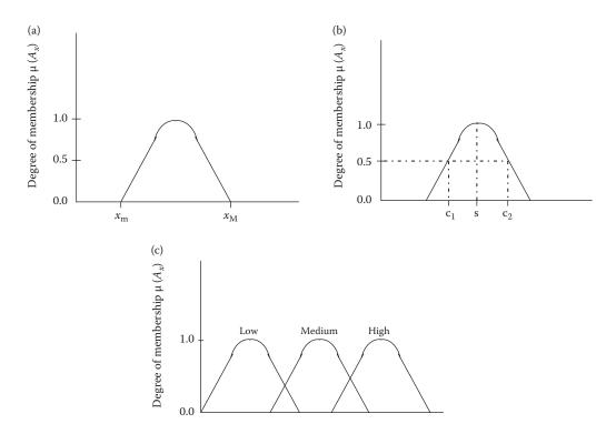
*Figure 51.4* (a)  $\pi$ -Shaped membership function. (b)  $\pi$ -Shaped membership function with crossover points. (c) Overlapping  $\pi$ -shaped membership function.
