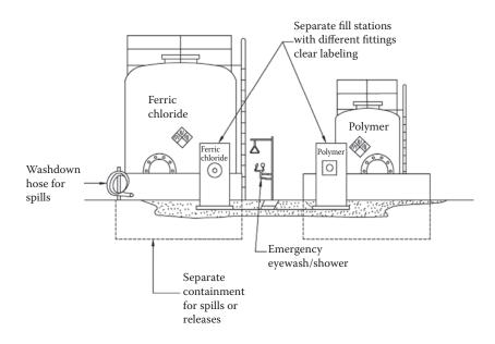
Figure 45.5 Chemical fill station diagram.
