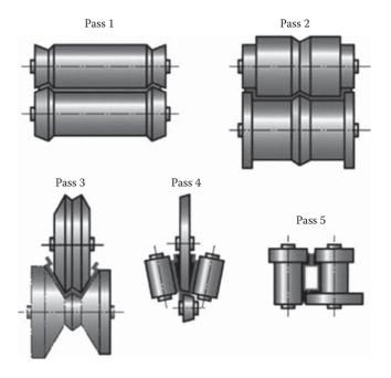
Figure 21.10 Roll forming of sheet metal (CES Edupack, 2012).
