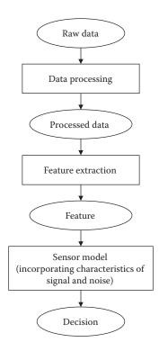
*Figure* **39.2** Data, features, characteristics, and sensor models in the attack-norm separation approach to cyber attack detection.
