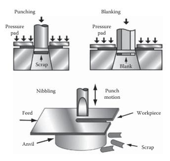
Figure 21.9 Punching, blanking, and nibbling processes (CES Edupack, 2012).
