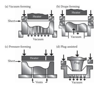
*Figure 21.15* Thermoforming processes assisted by vacuum (a), vacuum and drape moving against the vacuum (b), pressure (c), vacuum and plug moving in the direction of the vacuum (d).
