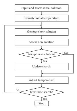
Figure 49.5 The structure of the SA algorithm.
