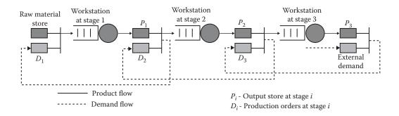
*Figure 20.1* Three-stage Kanban system.
