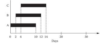
Figure 52.29 Gantt chart for network with lead and lag constraints (from Badiru and Pulat, 1995).
