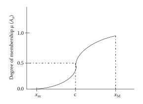
Figure 51.3 Growth S-shaped membership function with crossover point (c).
