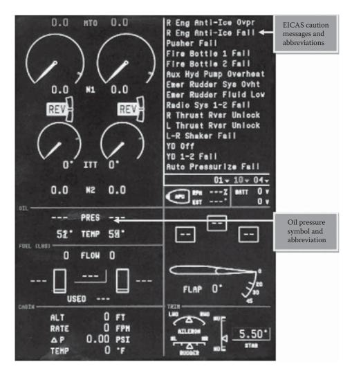
*Figure 26.7* Engine information and crew alerting system (EICAS). (Courtesy of Honeywell International Inc.)
