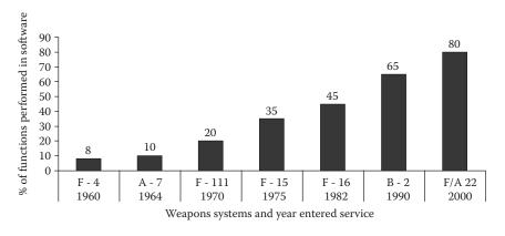
*Figure 32.1* Software growth in weapons systems. (From Fields, C., Task Force on Defense Software, Report from the office of the Undersecretary of Defense for Acquisition and Technology, Defense Science Board, Washington, DC, 11–12, 2000.)
