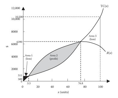
Figure 29.15 Break-even chart for revenue and cost functions.
