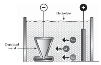
Figure 21.27 Electroplating (CES Edupack, 2012).
