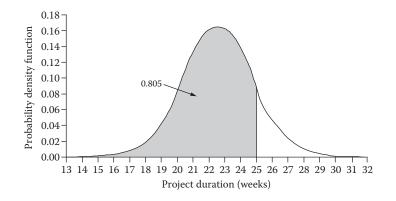
Figure 52.34 Example of probabilistic analysis with PERT.
