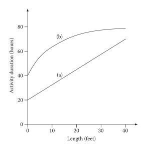
Figure 52.7 Two examples of activity duration as a function of length.
