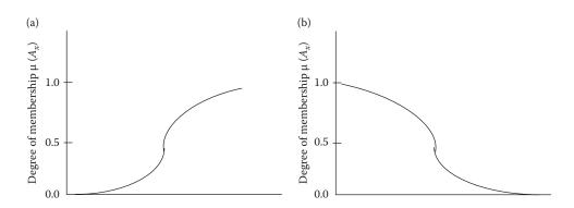
Figure 51.2 (a) Growth S-shaped membership function. (b) Decline S-shaped membership function.
