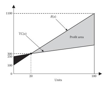
Figure 29.14 Area of profit versus area of loss.
