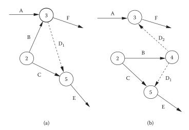
Figure 52.18 Subnetwork with two dummy arcs: (a) incorrect (b) correct.
