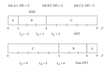
Figure 53.2 Optimality of EDD to Min Max lateness (single machine problem).
