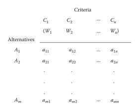
*Figure 37.1* Structure of a typical decision matrix.
