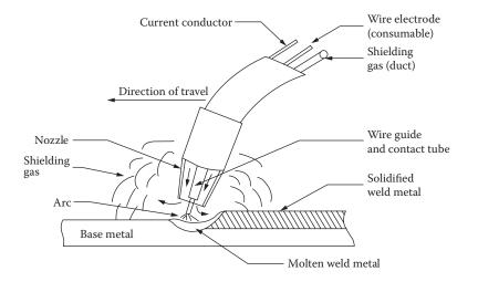
Figure 19.15 Gas metal arc welding (GMAW).
