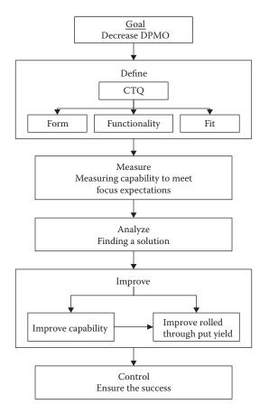
Figure 40.3 Six Sigma implementation process.
