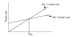
Figure 31.11 Breakeven between two alternatives with linear relations.
