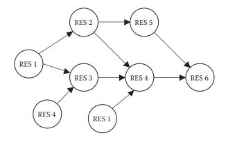
Figure 54.5 Basic critical resource diagram.
