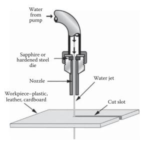
Figure 21.33 Water jet cutting (CES Edupack, 2012).
