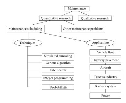
Figure 41.5 Methods and applications of maintenance scheduling.
