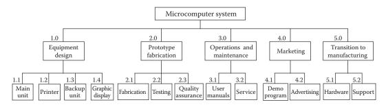
Figure 52.1 WBS for a microcomputer.
