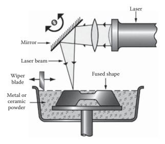
Figure 21.36 Selective or direct laser sintering (CES Edupack, 2012).
