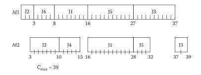
*Figure 53.4* Gantt chart of an optimal schedule. For the example in two  $C_{max}$  problem schedule, using Johnson's algorithm.
