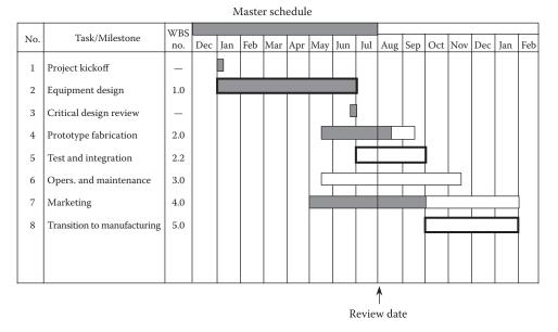
*Figure 52.13* Gantt chart for the microcomputer development example.
