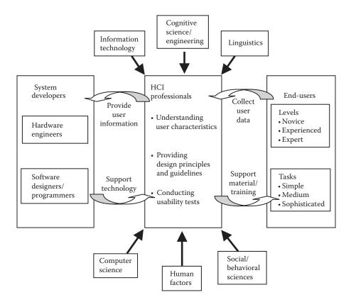
*Figure* 25.3 Conceptual diagram of relationships among system developers, HCI professionals, and end users. Not all of the related fields in HCI are present.
