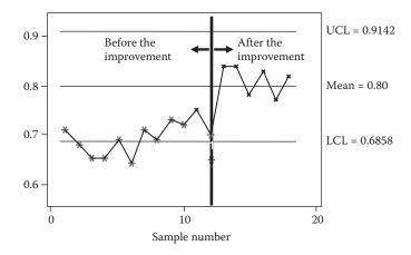
*Figure 18.5* X-bar chart for CSI. (1) The control limit 80% was the target established by the project team since it was considered to be world-class practice. (2) The upper and lower limits were determined based on three-sigma variations.
