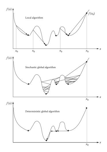
Figure 49.3 Types of structure of local and global minimization algorithms.
