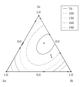
Figure 17.6 Contour plot for melting point.
