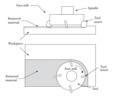
Figure 19.7 Face milling.
