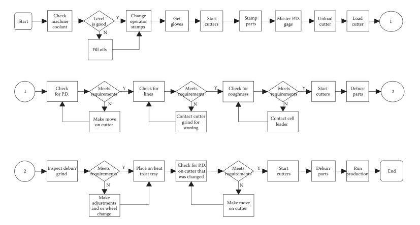
*Figure 18.4* Value-stream mapping of the cutter body process.
