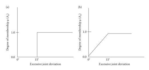
*Figure 51.1* (a) Crisp set for excessive joint deviation. (b) Fuzzy membership function for exvessive joint deviation.
