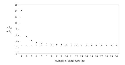
*Figure 43.2*  $B_{42}$  and  $B_4$  for  $\alpha = 0.005$  above UCL and n = 3.
