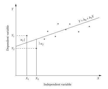
Figure 52.8 Typical scatter diagram.
