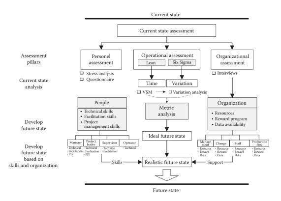
Figure 40.5 Assessment model flow for the implementation of Lean and Six Sigma.
