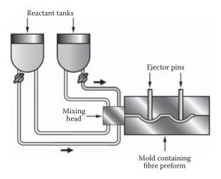
Figure 21.13 Reaction injection molding (CES Edupack, 2012).
