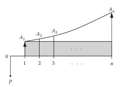
Figure 29.7 Increasing geometric series cash flow.
