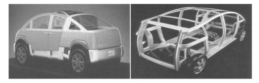
Figure 22.19 Aluminum concept car and body frames (Buchholz, 1999).
