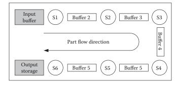
Figure 28.3 Serial process configuration.
