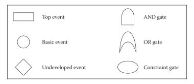
Figure 46.6 Basic fault tree symbols.
