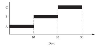
Figure 52.27 Gantt chart for serial network (from Badiru and Pulat, 1995).
