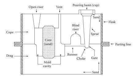
Figure 19.1 Sand casting.
