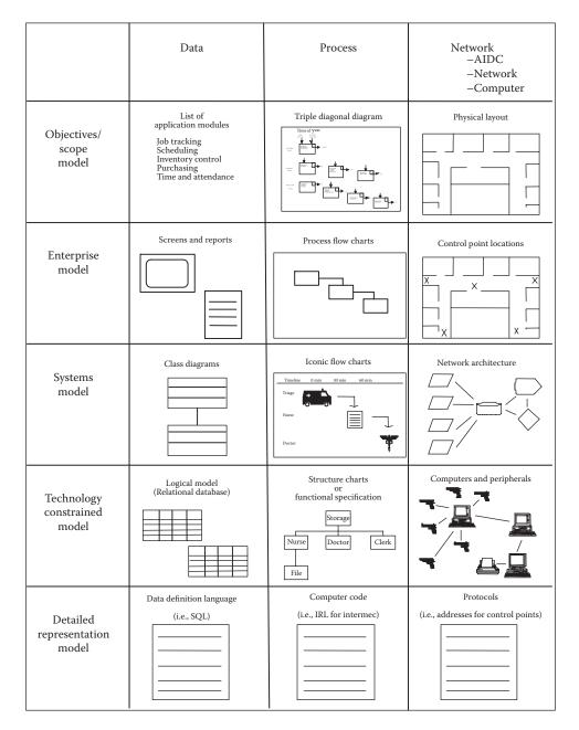
Figure 36.1 Zachman framework for enterprise systems architecture.
