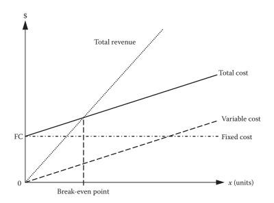
Figure 29.11 Break-even point for a single project.
