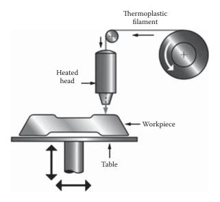
Figure 21.35 Fused deposition modeling (CES Edupack, 2012).
