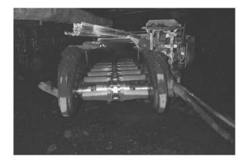
*Figure 45.9* Design improvements to the onboard conveyor of a continuous coal mining machine reduce noise exposures. Coating the chain conveyor and flight bars protects mine operators' hearing, and extends the life of the chain.
