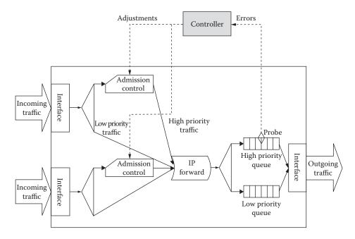
*Figure 39.1* A QoS model of a router with PID feedback control. (From Yang, Z., Ye, N., Lai, Y.-C., *Qual. Reliab. Eng. Int.*)
