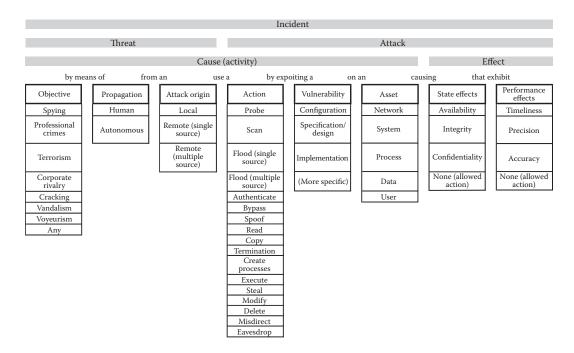
*Figure 39.3* The System-Fault-Risk framework for attack analysis and classification. (From Ye, N., Newman, C., and Farley, T., *Information Systems Frontiers*.)
