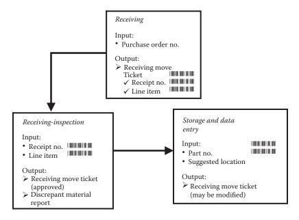
Figure 36.8 Proposed receiving process flow diagram.
