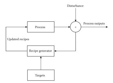
Figure 42.1 A feedback-controlled process.
