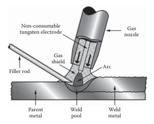
Figure 21.25 Tungsten inert gas welding (CES Edupack, 2012).
