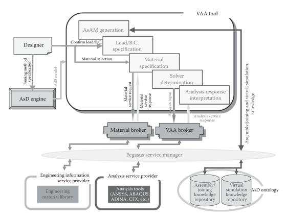
Figure 22.13 Service-oriented VAA architecture.
