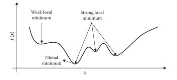
Figure 49.1 Types of minima for unconstrained optimization problems.
