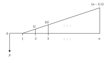
Figure 29.5 Arithmetic gradient cash flow with zero base amount.
