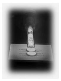
Figure 21.28 Physical vapor deposition (CES Edupack, 2012).
