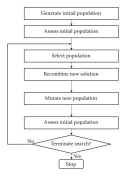
*Figure* **49.6** The basic structure of a genetic algorithm.
