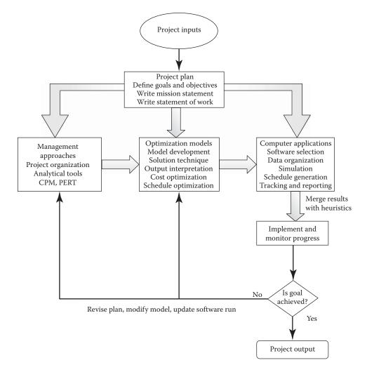
Figure 33.6 Flowchart of integrated project management.
