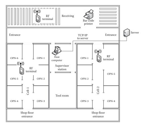
Figure 36.11 Overlay of material tracking system on facility layout.
