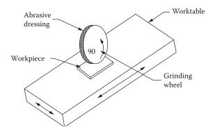
Figure 19.11 Grinding.
