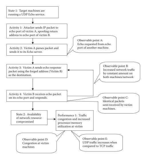
*Figure* **39.4** Cause-effect chain of a UDP storm attack on computer networks. (From Ye, N., Newman, C., and Farley, T., *Information Systems Frontiers*.)
