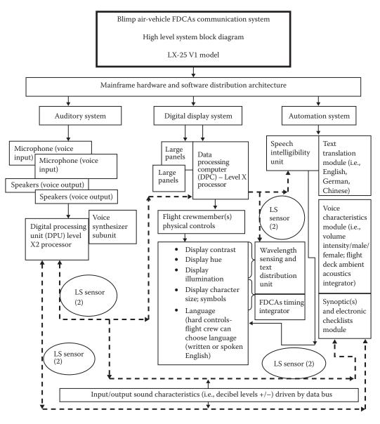
*Figure 26.8* Integrated XYZ Blimp high-level communication system block diagram—FDCASs and flight crew interface logic diagram part I. (Courtesy of Dujuan B. Sevillian.)
