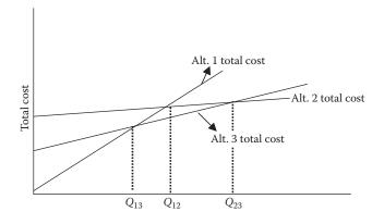
Figure 31.12 Breakeven between three alternatives with linear relations.
