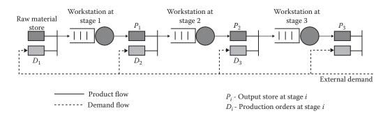
Figure 20.2 Three-stage base stock system.
