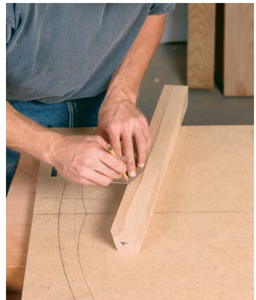
LAY OUT THE SECOND POMMEL CUT. The template drawing of the back of the seat, a straightedge, and a curved cardboard template are used to lay out the second cut that will finish up the rough pommel shape.
