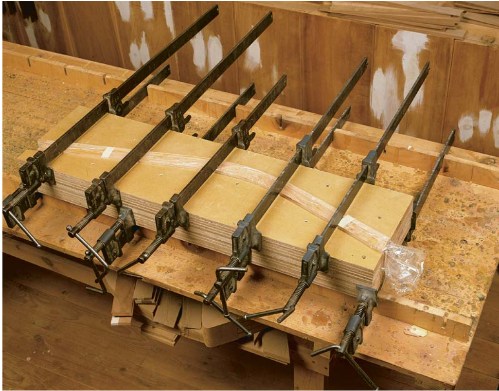
SIMPLE FORM MAKES bent-lamination easy. Plywood scraps form two mating halves with square outside edges to provide even clamping pressure over the length of the back-leg lamination.
