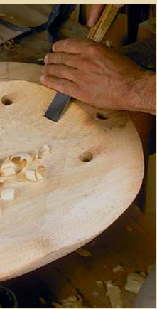
details with gouges. STEP 6: Smooth the seat contour with sandpaper.
