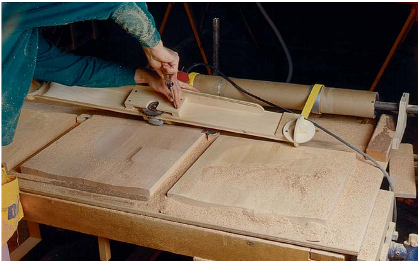
WHEN DUPLICATING A SEAT, Trimble moves his jig with the grain, taking ¼ in. at a pass. In actuality, the carving wheel cuts across the grain. To minimize grain tearout, Trimble makes an initial L-shaped swath with the cutter, which reveals the seat's pommele. Here, part way through a seat, he adjusts the guard.
