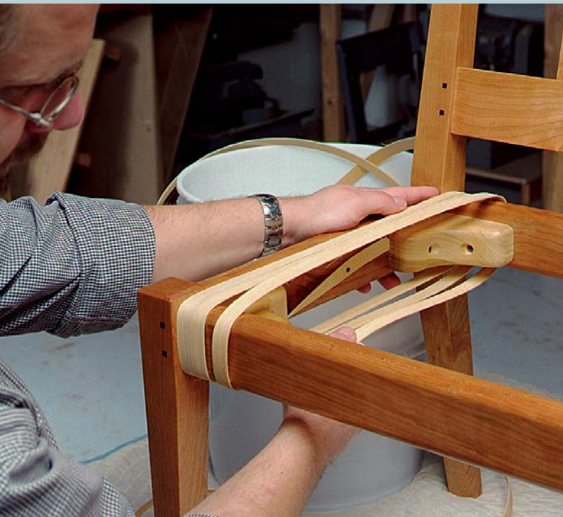
BEGINNING THE WARP. The first length of reed goes under the front seat rail and over the back and continues in this way to the end of the seat.
