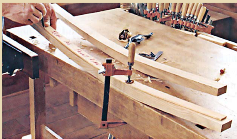
USING THE SIDE TEMPLATE , cut all of the legs from one wide 8/4 board to ensure uniform color (left). Lay out the legs for best grain orientation and strength (above).
