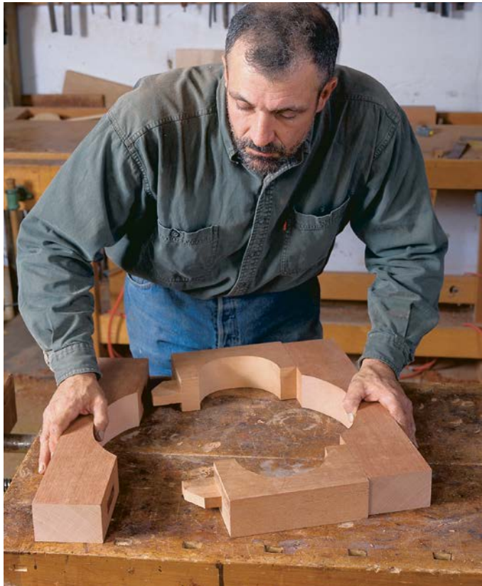
ASSEMBLE THE FRAME. The bulk of the frame has been reduced by bandsawing arc-shaped segments prior to assembly.
