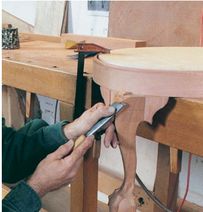
KNEE WORK. WITH THE LEG dry-fitted, rough-shape the upper leg, blending the knee to the frame. Final fairing with a rasp is done after glue-up.
