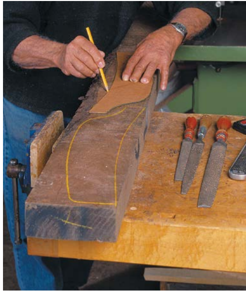
INTERLOCKING LAYOUT. Tracing a plan-view pattern, the author lays out chair arms in a 12/4 walnut board. He flops the pattern and nests the layouts to get as many arms as possible from the board.
