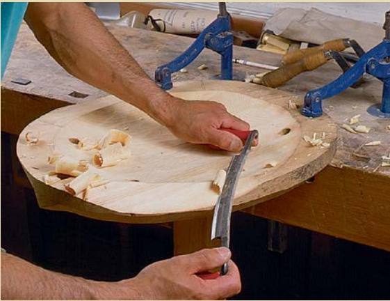
STEP 3: Shape convex surfaces with a drawknife.
