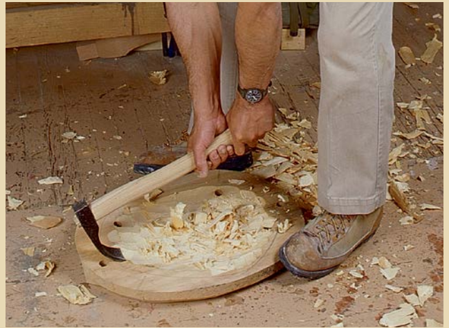
STEP 1: Rough the seat hollow with an adze.
