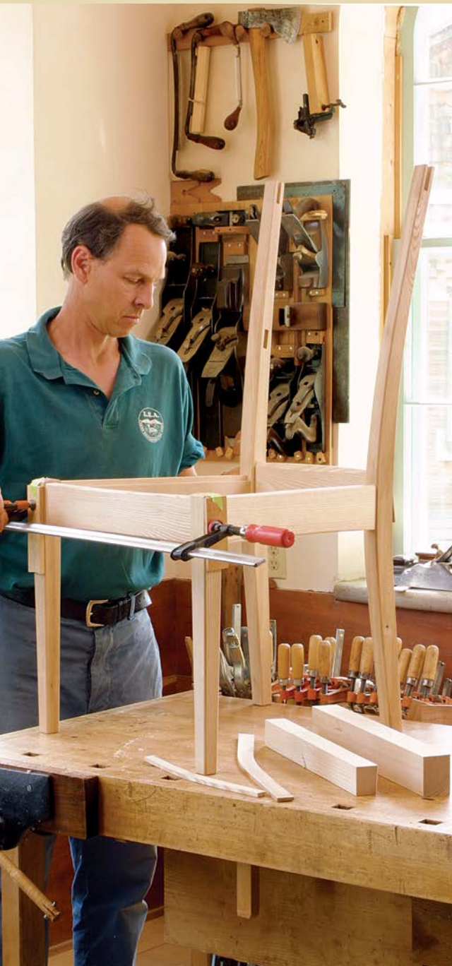
DRY-CLAMP THE SEAT FRAME. After hand-fitting all of the joinery in the seat frame, clamp it together and fit the upper cross-pieces to the actual chair.
