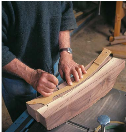
ADDING ANOTHER DIMENSION. With the arm blank jointed and planed, the author traces a second pattern to establish the general contours of the arm's elevation.
