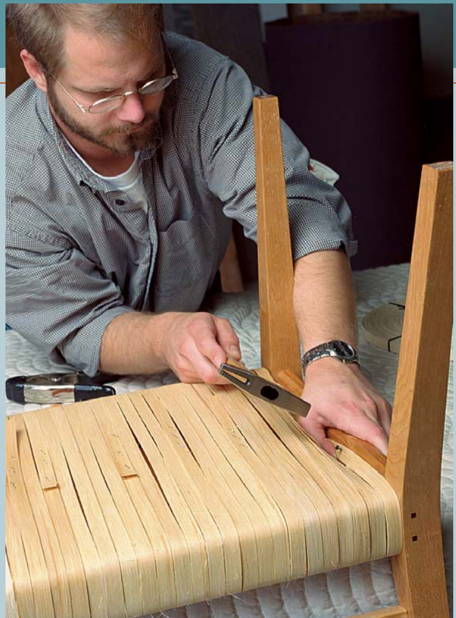
ENDING THE WARP. When you reach the side rail, pull the reed underneath the seat and use a #3 upholsterer's tack to secure it to the seat rail.
