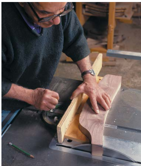
GOOD REFERENCES. The compound angle where the arm will join the chair's back leg is cut on the tablesaw while the arm is still flat on the top and bottom. A simple, curved plywood jig steadies the curved side of the arm for the cut.
