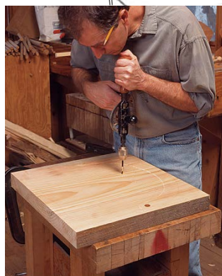
QUICK DEPTH GAUGE. Two holes drilled 1 in. deep provide the main points of reference for carving out the seat.
