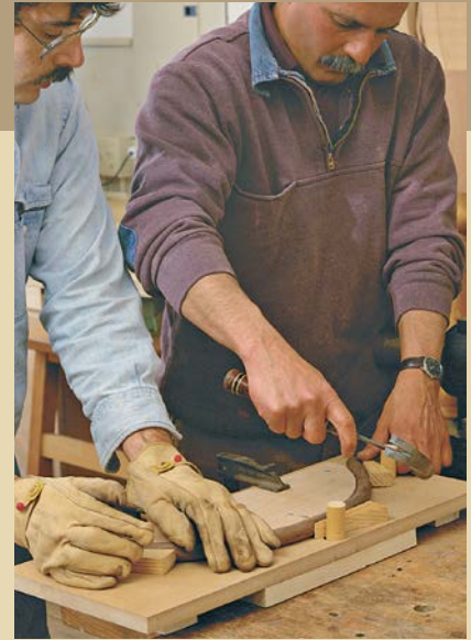
RAIL-BENDING JIG. Four hands are better than two for forcing the steamed rail into shape. The author is assisted by Les Katz, one of his students. Wedges hammered between the plywood form and the wooden pegs hold the rail tightly in place.
