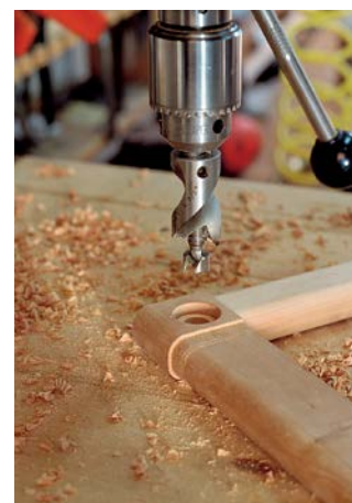
DRILL THE STEPPED MORTISES in the seat frame. Center the undercarriage on the seat frame and mark the mortise locations (left). The author uses a commercial counterbore bit (above) to machine the two-stage mortise accurately, in one shot.
