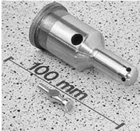
Fig. 10.14 Diesel engine pre-chamber made of PM 2000 (pin and burner base) [2, 51].
