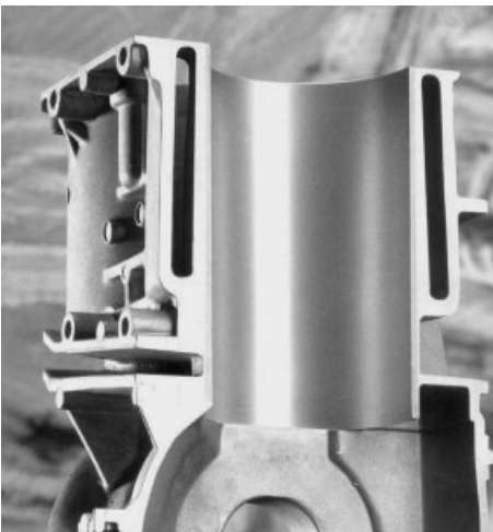
Fig. 3.19 Crankcase part with running surface reinforcement (Lokasil).
