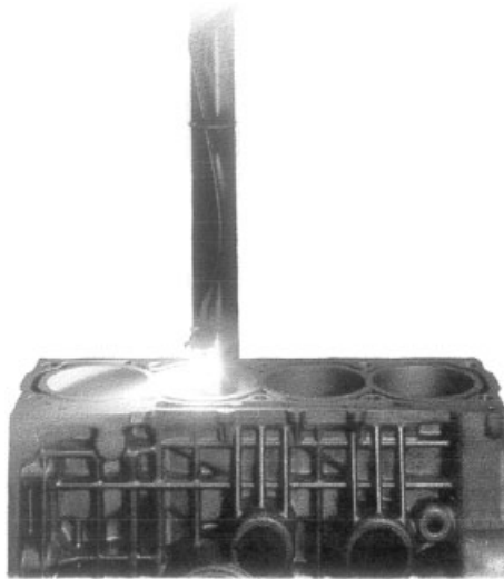
Fig. 9.17 Plasma spraying allows the application of various coating types.
