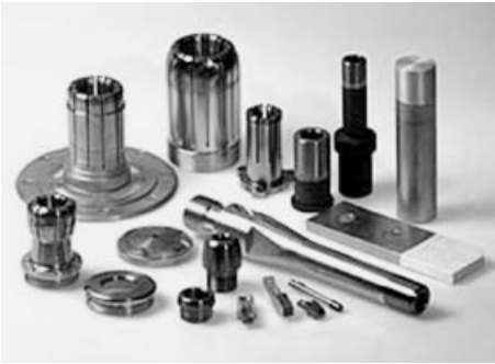
Fig. 10.20 Burn down contacts of W–Cu [2, 51].
