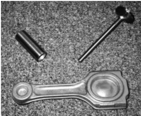
Fig. 10.17 Valve, piston rod and pin, made of CermeTi composite [101].
