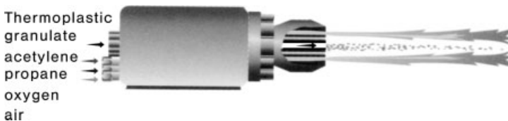
Fig. 5.5 Principle of plastic flame spraying (Linde AG).
