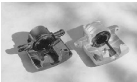
Fig. 1.64 Disk brake calliper for passenger cars of conventional cast iron (left) and an aluminum matrix composite material (AMC) with Nextel® ceramic fiber 610 [67].
