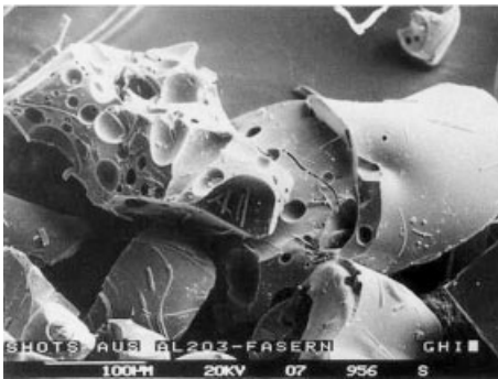
Fig. 3.5 Shot particles in aluminum oxide fibers.
