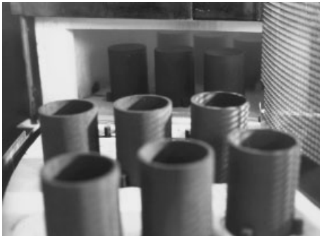
Fig. 4.15 Heated preforms taken out of the preheating furnace [12].
