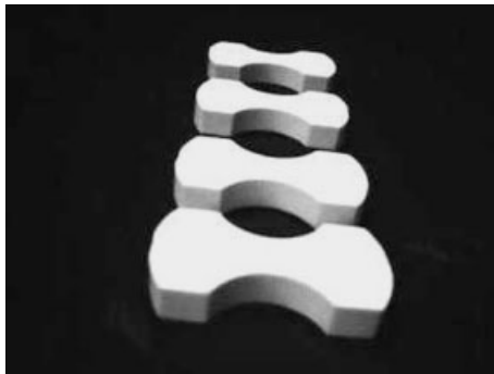
Fig. 3.17 Cylinder head preforms to reinforce the valve bridges.
