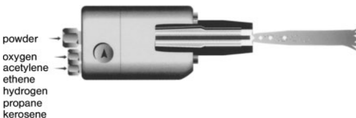
Fig. 5.8 Principle of high speed flame spraying (Linde AG).
