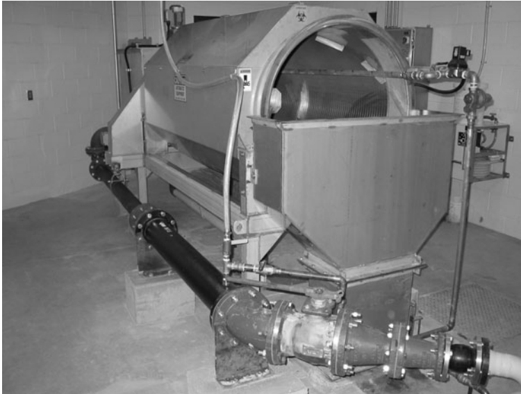
FIGURE 9.20 An example of a rotary drum thickener (courtesy of Vulcan Industries, Inc.).
