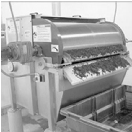
FIGURE 9.3 An example of a Rotostrainer® externally fed rotary drum screen (courtesy of Parkson Corporation, Fort Lauderdale, Florida).
