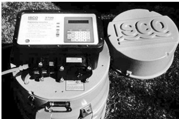
FIGURE 3.6 An example of a commercially available automatic sampler (courtesy of TELEDYNE ISCO, Lincoln, Nebraska).
