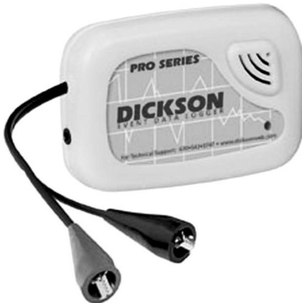
FIGURE 3.2 An example of an event recorder (Model EV100) (courtesy of Dickson Company, www.DicksonData.com ).
