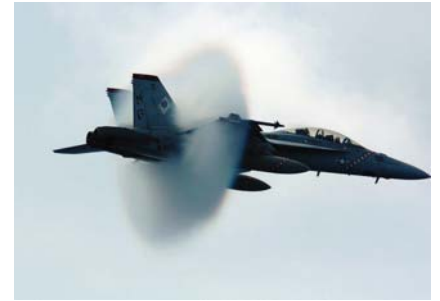
FIGURE 2–15 Vapor cloud around an F/A-18F Super Hornet as it flies near the speed of sound.
