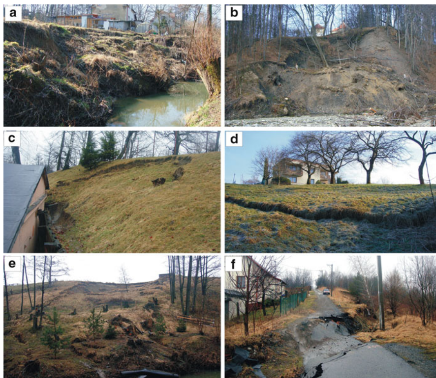
Fig. 13.4 Examples of typical landslides of the May 2010 event. (a) Right bank of the Horní Datyňka River is affected by translational landslides along a length of 100 m due to lateral erosion (Horní Datyně village). (b) A debris slide situated below the church in Skalice village formed due to lateral erosion of the Morávka River. (c) Incipient translational landslide in Orlová town. (d) Tension cracks in the upper part of a shallow translational landslide, Horní Bludovice village. (e) Rotational landslide in the Quaternary deposits, endangering two houses in Stonava village. (f) Large rotational landslide in Doubrava village. Two houses suffered structural damage and had to be demolished (Photos by L. Kubiszová)
