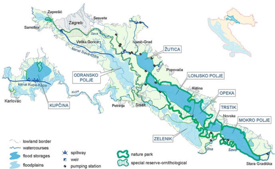
Fig. 9.8 Flood protection system in the Central Sava region (Srednje Posavlje)
