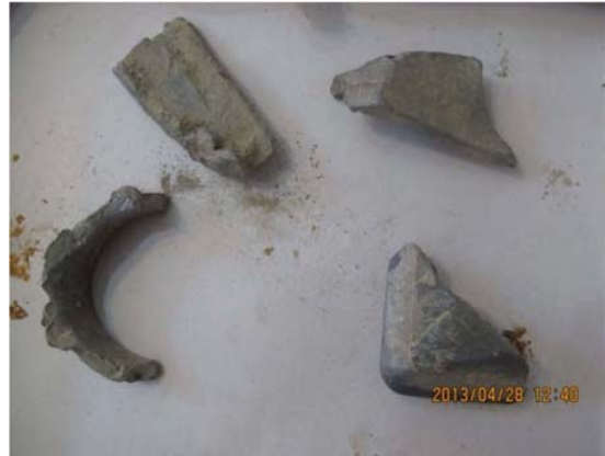
Figure 6-Broken piece of nails and rollers in slurry line
