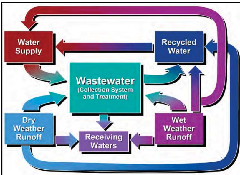
Figure 1-2: City of LA's One Water Vision (2006 City of Los Angeles Recycled Water Master Plan)
