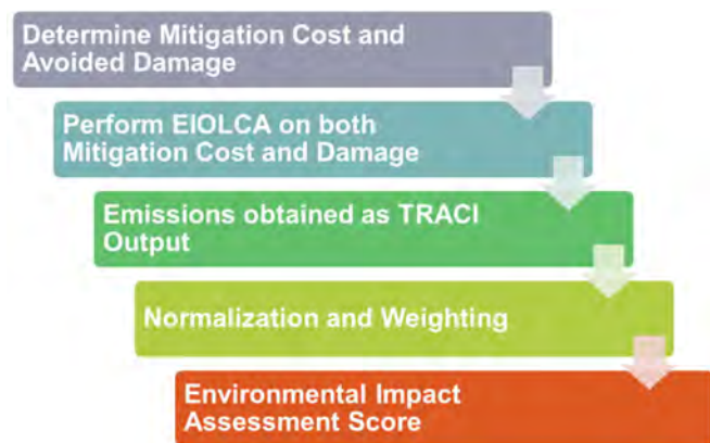
Figure 4: The process of converting the cost and benefits of seismic retrofit from dollars to environmental impacts.
