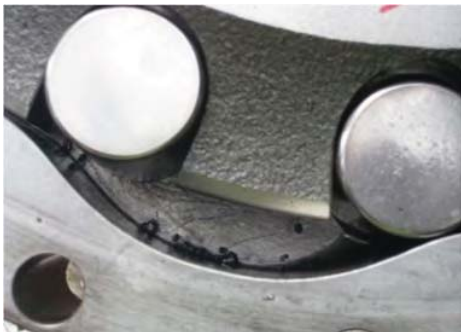
Figure 5-a- details of damaged hydro motor
