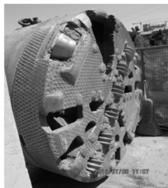
Figure 17-b-Damage of Cutter head in facing boulders
