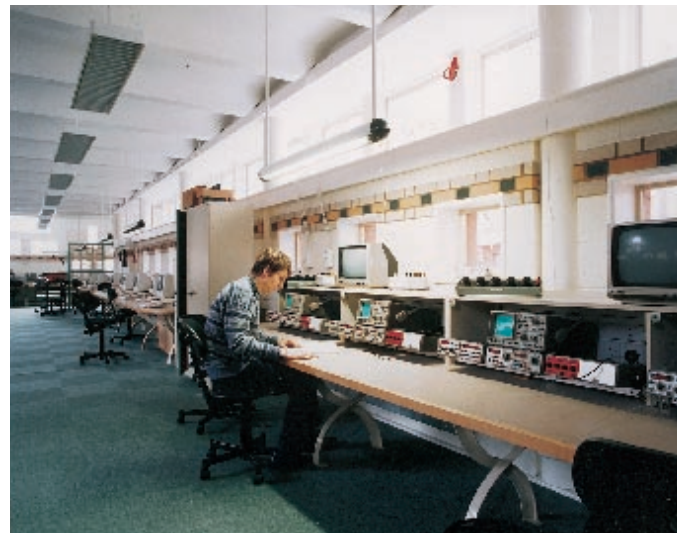
Figure 1.13 De Montfort Engineering Building, Leicester, maximises daylight by incorporating high windows; light shelves reduce glare. Smaller windows provide a view for individuals sitting at the workstations
