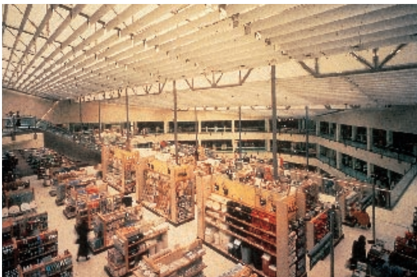
Figure 1.2 Daylight brought into the centre of the John Lewis store, Kingston, to provide natural colour
