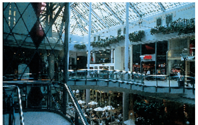
Figure 1.9 The atrium at the Harlequin Centre, Watford, allows daylight to penetrate far into the interior of the shopping mall
