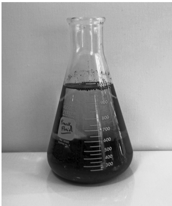
FIGURE 4.1 Water is combined with sand and a cocktail of chemicals to help in the fracking process.
