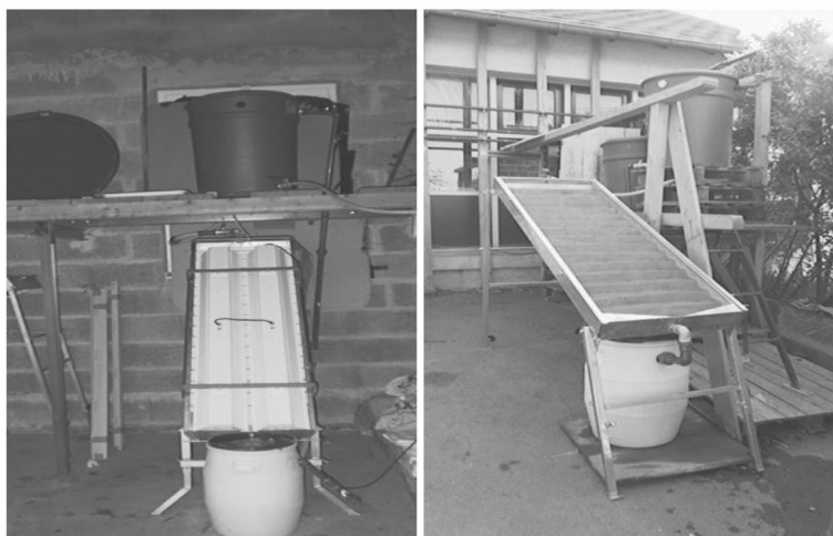
Figure 18. Treatment of vine pesticide-containing rinsing waters in a Cascade Falling Film photoreactor, working either in sunlight during day time (right) or with UV-lamps in a workshop in periods of intense vine treatments (left).
