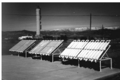
Figure 13. Picture and scheme of the CPC photoreactor at PSA.
