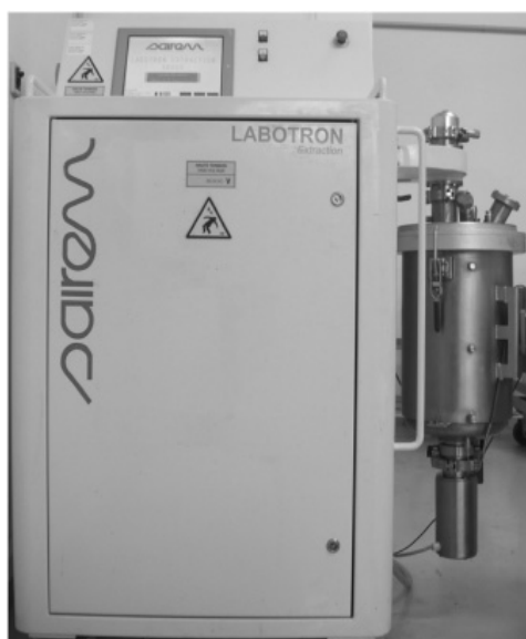
Figure 16. Labotron Extraction™ reactor (SAIREM) for the extraction of phytoactive compounds using vegetable oils.
