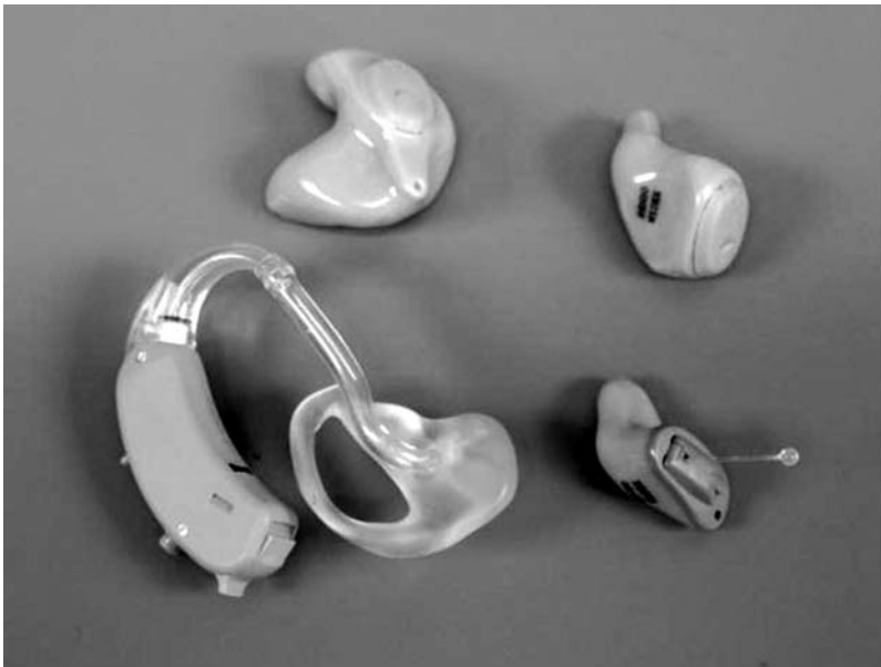
Figure 2 Four styles of hearing aids ( clockwise from bottom left ): behind the ear, in the ear, in the canal, completely in the canal.
