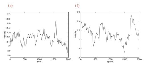
Figure 10.10.1 Typical (a) temporal and (b) spatial variation of a velocity component in a turbulent flow.
