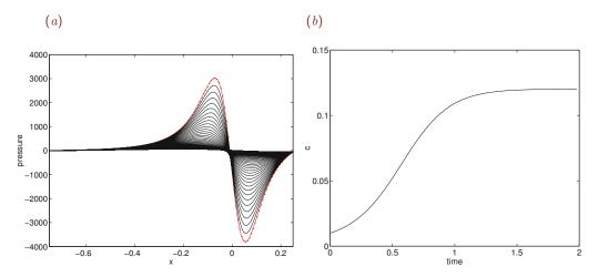
Figure 9.1.6 Evolution of (a) the pressure distribution and (b) the lubrication gap, computed by the numerical method implemented in the code bear\_2d. The initial distribution is plotted by connected dots in (a).
