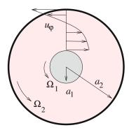
**Figure 7.6.1** Illustration of swirling flow between two rotating concentric cylinders. When the gap between the cylinders in small, we obtain Couette flow between two translating parallel plates in the absence of a pressure gradient.
