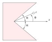
**Figure 9.8.1** Because the local Reynolds number of the flow near a corner is small, the motion of the fluid is governed by the equations of Stokes flow. Similarity solutions can be derived working in local plane polar coordinates,  $(r, \theta)$ .
