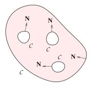
Figure 12.7.2 A control area in the xy plane confined by a collection of closed contours, C, is used to establish Green's third identity; N is the unit vector normal to the boundaries pointing into the fluid.
