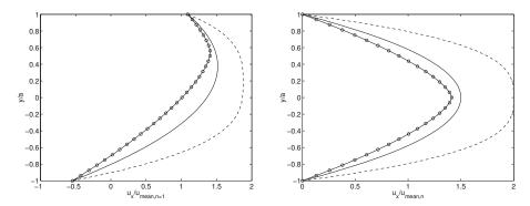
Figure 7.1.8 Velocity profiles for a typical configurations with power-law exponent n=0.5 (broken line), 1 (solid line), and 2 (connected circular symbols). The velocity has been scaled with the mean velocity of a Newtonian fluid.
