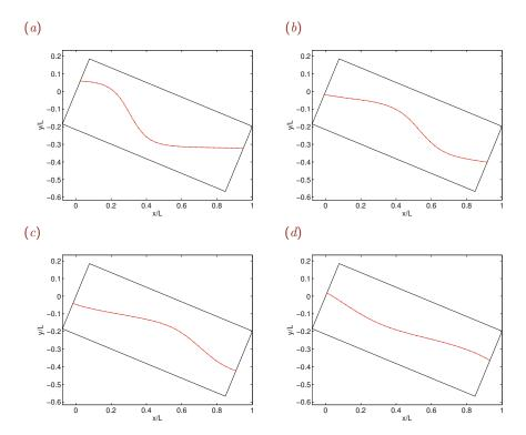
Figure 9.4.2 Snapshots of an evolving interface between two layers in a channel confined between two parallel walls computed by code *chan2l\_exp*.
