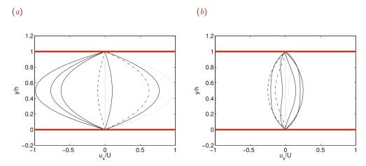
Figure 7.8.3 Velocity profiles of pulsating pressure-driven flow in a two-dimensional channel confined between two parallel walls at phase angles  $\Omega\,t/\pi=0$  (dashed lines), 0.25 (dashed-dotted lines), 0.50 (dotted lines), 0.75, 1.0, 1.25, 1.50, 1.75, and 2.0, for Womersley number (a) Wo = 1/2 and (b) 3.0.
