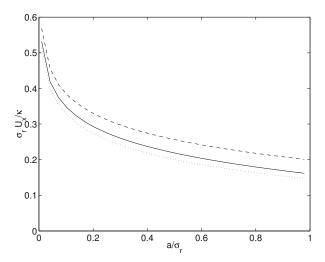
Figure 11.5.6 Self-induced velocity of a vortex ring of radius  $\sigma_r$  and circulation  $\kappa$  plotted against the ratio of the core to the ring radius,  $a/\sigma_r$ . The solid and dashed lines correspond, respectively, to a ring with uniform or diffuse vorticity distribution described by equations (11.5.36) and (11.5.37). The dotted line represents Kelvin's asymptotic prediction for small core radius expressed by equation (11.5.38).
