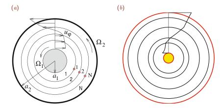
Figure 7.6.2 (a) Illustration of multi-layer annular swirling flow between two rotating concentric cylinders. (b) Velocity profile across five annular layers.
