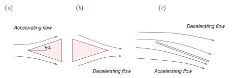
Figure 10.5.1 Boundary layers in accelerating or decelerating flow: (a, b) flow past a wedge and (c) uniform flow past a flat plate at a non-zero angle of attack.
