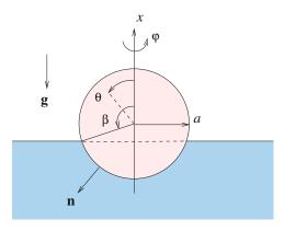
Figure 5.2.2 Illustration of a sphere floating in the flat surface of a liquid at floating angle  $\beta$ . The dashed line represents the horizontal circular contact line.
