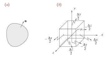
Figure 5.1.1 (a) Illustration of a parcel of a stationary fluid showing the outward unit normal vector, n. (b) A parcel with a rectangular parallelepiped shape serves as a control volume for deriving the differential equations governing the pressure distribution in hydrostatics.
