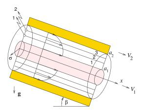
Figure 7.4.2 Illustration of unidirectional annular flow through an annular tube with translating walls for N=3 layers. The interface labels are shown on the left and the layer labels are shown on the right.
