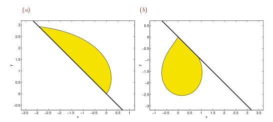
Figure 5.8.2 Interfacial shapes of (a) a sessile two-dimensional drop for inclination angle  $\beta=0.25\,\pi$ , and (b) pendant two-dimensional drop for inclination angle  $\beta=1.25\,\pi$ , generated by the FDLIB code  $drop\_2di1$ .
