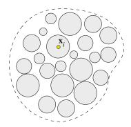
Figure 11.3.1 A vortex region in a two-dimensional flow is discretized into small parcels. Each parcel is then condensed into a point vortex located at a designated parcel center. As the number of parcels tends to infinity, the velocity induced by the point vortices is expressed by the integral representations given in (11.3.4) and (11.3.5).
