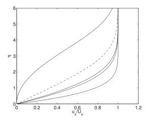
Figure 10.5.2 Velocity profiles across Falkner–Skan boundary layers for several values of the acceleration parameter m; from bottom to top, m=1.5 (dotted line),  $1.0,\ 0.25,\ 0.176,\ 0.0$  (dashed line), and -0.0904.
