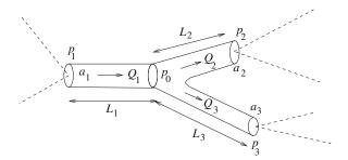
Figure 7.3.3 Illustration of a bifurcating tube in a network. The dashed lines represent other tube segments.
