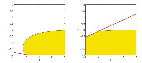
Figure 5.5.2 A semi-infinite meniscus attached to an inclined plate generated by the FDLIB code  $men\_2d\_plate$ . The plate inclination angles  $\chi$  are different, but the contact angle  $\alpha$  is the same in both cases.
