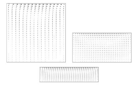
Figure 8.8.2 Velocity vector fields of two-dimensional Stokes flow in cavities with different aspect ratios driven by a sliding lid computed on a staggered grid using the FDLIB code cvt\_stag.
