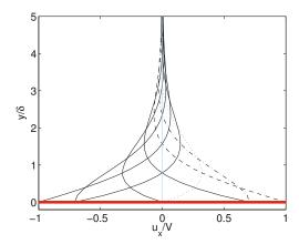
Figure 7.8.2 Velocity profiles due to the in-plane oscillation of a plate in a semi-infinite viscous fluid at phase angles  $\Omega t/\pi=0$  (dashed line), 0.25 (dashed-dotted line), 0.50 (dotted line), 0.75, 1.0, 1.25, 1.50, 1.75, and 2.0. The y coordinate is scaled by the Stokes boundary layer thickness,  $\delta$ , defined in (7.8.14).
