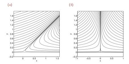
Figure 9.8.2 Streamline pattern of flow in the neighborhood of a stagnation point on a plane wall with a rectilinear dividing streamline. The angle subtended between the dividing streamline and the wall is (a)  $\alpha = \pi/4$  and (b)  $\pi/2$ .
