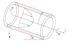
Figure 7.3.1 Illustration of steady unidirectional flow through a horizontal or inclined circular tube.
