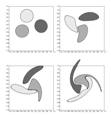
Figure 11.3.6 Evolution of three vortex patches computed by the method of contour dynamics for two-dimensional flow implemented in a code entitled *vp\_2d*. In the course of the interaction, the three vortices merge into a larger vortex with spiral filaments.
