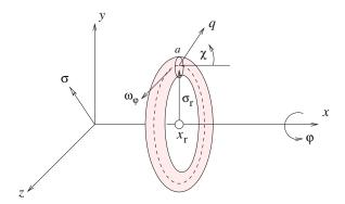
Figure 11.5.5 Illustration of a vortex ring with radius  $\sigma_r$  and a circular core of radius a.
