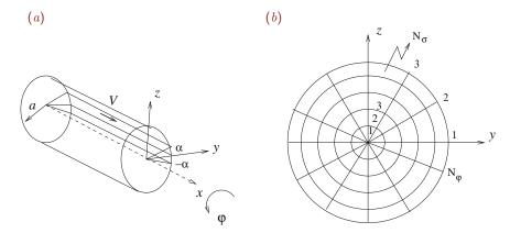
Figure 7.3.6 (a) Illustration of unidirectional flow through a circular tube due to the translation of a sector with semi-angle  $\alpha$ . (b) Discretization of the tube cross-section for the purpose of computing the flow rate using the mid-point rule.
