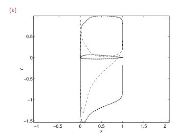
Figure 12.4.2 (a) Streamline pattern and distribution of the pressure coefficient on the upper and lower surfaces of an airfoil for angle of attack  $\alpha=5^{\circ}$ , computed using the linear vortex panel method. (b) Distribution of the pressure coefficient (dashed line) and panel strength (connected dots) around another airfoil. These solutions were generated by the FDLIB code  $airf\_2d\_lvp$ .
