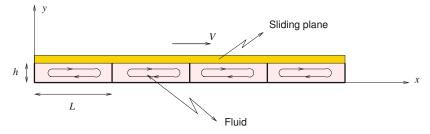
Figure 7.1.4 Illustration of a plate sliding over a stationary surface fitted with vertical plates. The space between the plates is filled with a viscous fluid.
