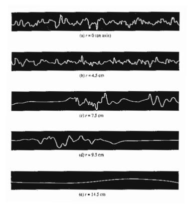
**Figure 10.10.4** Temporal velocity fluctuations in turbulent pipe flow at different distances from the tube wall, showing the presence of the laminar sublayer and the buffer zone near the wall, after Corrsin, S. (1943) Investigation of flow in an axially asymmetric heated jet-air. *NACA Rep. 3L23*.
