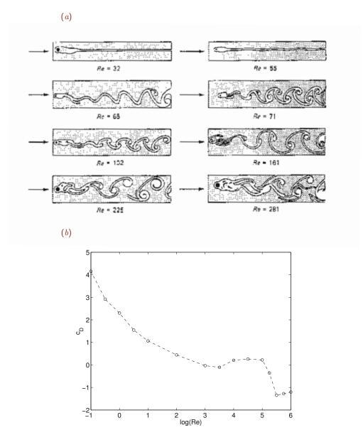
Figure 10.1.1 (a) Schematic illustration of changes in the structure of streaming flow past a circular cylinder with increasing Reynolds numbers, showing boundary-layer separation and the development of a wake, after *Homann*, *F*. (1936) Einfluss grosser zähigkeit bei strömung um zylinder. Forschg. Ing.-Wes. 7, 1–10. (b) Drag coefficient plotted against the Reynolds number defined with respect to the cylinder diameter.
