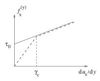
Figure 4.8.1 Rheological response of a Bingham plastic showing a yield-stress behavior in unidirectional flow.
