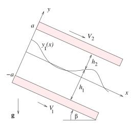
Figure 9.4.1 Illustration of flow of two layers in a channel confined between two parallel plane walls driven by gravity, boundary motion, or an imposed pressure gradient.
