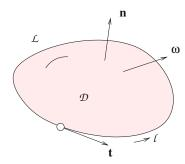
Figure 11.4.1 Illustration of a loop in three-dimensional flow,  $\mathcal{L}$ , enclosing a patch,  $\mathcal{D}$ . The circulation around the loop is equal to the surface integral of the normal component of the vorticity,  $\boldsymbol{\omega} \cdot \mathbf{n}$ , over  $\mathcal{D}$ .
