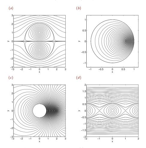
Figure 11.2.2 Streamline pattern of the flow due to (a) a pair of point vortices with opposite strength, (b) a point vortex inside a circular cylinder, (c) a point vortex outside a circular cylinder, and (d) a periodic array of point vortices. These streamline patterns were generated by the program strml residing in directory 04\_various of FDLIB.
