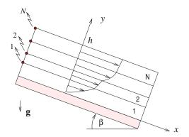
Figure 7.2.2 Illustration of gravity-driven multi-film flow down a plane that is inclined by an angle  $\beta$  with respect to the horizontal. The interfacial labels are printed on the left and the film labels are printed on the right.
