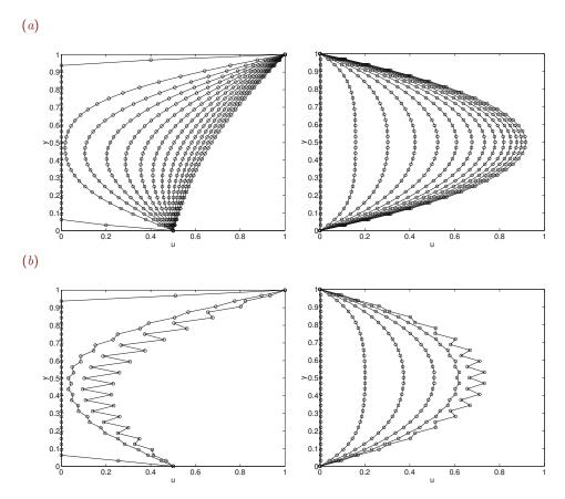
Figure 8.2.2 Evolving profiles of unidirectional flow in a channel computed by an explicit finite-difference method for numerical diffusion number (a)  $\alpha = 0.40$  and (b) 0.51. The scary oscillations in the second case are a manifestation of numerical instability.
