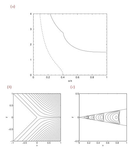
Figure 9.8.3 (a) Graphs of the real part (solid line) and imaginary part (broken line) of the exponent  $\lambda$  with the smallest real part for antisymmetric flow between two walls intersecting at an angle  $2\alpha$ . When  $0.41\pi < \alpha < \pi$ ,  $\lambda$  is real; when  $0 < \alpha < 0.41\pi$ ,  $\lambda$  is complex. (b, c) Streamline pattern of antisymmetric flow in a corner with half-angle (b)  $\alpha = 135^{\circ}$ , and (c)  $10^{\circ}$ .
