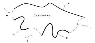
Figure 6.2.1 Illustration of a stationary control volume (cv) in a flow bounded by solid or fluid surfaces.
