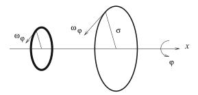
Figure 6.6.2 The vorticity of a point particle in an axisymmetric flow increases as the particle moves farther away from the axis of symmetry due to vortex stretching.
