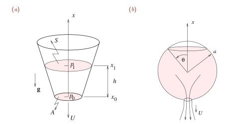
Figure 6.4.2 Illustration of the gravitational drainage of a fluid from a (a) conical or (b) spherical tank. The exit velocity can be computed from Bernoulli's equation for irrotational flow, resulting in Torricelli's law.
