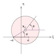
Figure 12.2.3 A Joukowski airfoil is generated by mapping conformally a circle in the  $\xi\eta$  plane to an airfoil contour in the xy plane. The first singular point, located at the  $\xi$  axis at  $\xi=-\sigma$ , is mapped to the airfoil trailing edge. The second singular point, located at  $\xi=\sigma$ , is mapped inside the airfoil.
