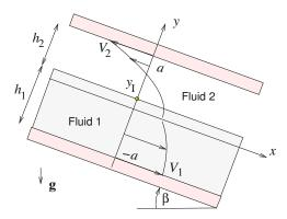
Figure 7.1.5 Illustration of steady two-layer flow through an inclined channel confined between two parallel walls located at  $y=\pm a$ .
