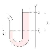
Figure 5.1.2 Illustration of a U-tube manometer. The pressure distribution in the fluid is described by the equations of hydrostatics even if the fluid has a convoluted shape, as long as it remains contiguous and uninterrupted.
