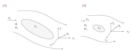
Figure 6.7.1 Illustration of flow in two similar domains. If the Reynolds numbers of the two flows are equal, as shown in equation (6.7.10), the velocity and pressure field of the second flow may be deduced those in the first flow, and *vice versa*, by rescaling.
