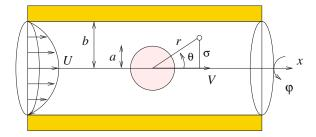
Figure 9.6.2 Illustration of a spherical particle moving along the axis of a circular tube with velocity V in the presence of an ambient Poiseuille flow.
