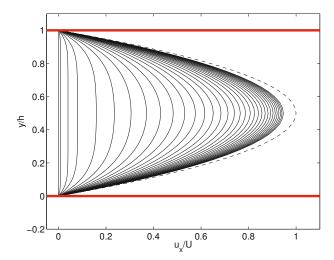
Figure 7.7.3 Transient velocity profiles in a channel with parallel walls separated by distance h, due to the sudden application of a constant pressure gradient or sudden tilting. Profiles are shown at dimensionless times  $\nu t/h^2=0.001,\ 0.005,\ 0.01,\ 0.02,0.03,\ \dots$  The dashed line describes the parabolic profile of the Hagen flow with centerline velocity U established at long times.
