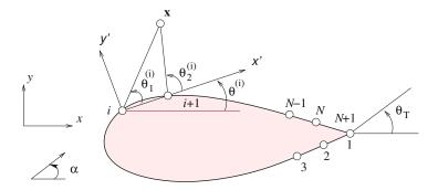
Figure 12.4.1 Discretization of the contour of an airfoil into N flat panels defined by a set of N+1 nodes.
