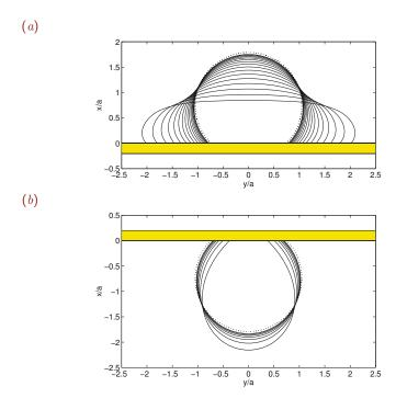
Figure 5.7.2 Shapes of (a) sessile and (b) pendant two-dimensional drops for contact angle  $\alpha = \frac{3\pi}{4}$  and different surface tensions computed using the FDLIB code  $drop\_2d$ . The dotted lines trace the approximate circular shape established for small drops or high surface tension. The x and y coordinates have been scaled by the equivalent drop radius, a, defined in terms of the drop area as  $A_D = \pi a^2$ .
