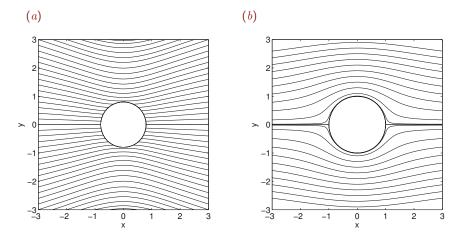
**Figure 9.5.1** Streamline pattern of axisymmetric Stokes flow due to the translation of a sphere along the x axis in an infinite fluid. Streamlines are drawn (a) in a stationary frame of reference and (b) in a frame of reference moving with the sphere.
