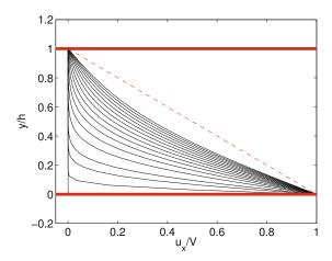
Figure 7.7.1 Transient Couette flow in a channel with parallel walls due to the impulsive translation of the lower wall. Profiles are shown at dimensionless times  $\nu t/h^2 = 0.001, \, 0.005, \, 0.010, \, 0.020, \, 0.030, \, \ldots, \, 0.14, \, \text{and} \, 0.15$ . The straight line is the linear profile established at long times.
