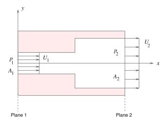
Figure 6.2.1 Simplified model of flow through a duct with a sudden enlargement. An integral momentum balance allows us to compute the rise in pressure,  $p_2 - p_1$ , in terms of the inlet and outlet cross-sectional areas,  $A_1$  and  $A_2$ .
