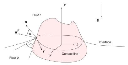
Figure 5.12.1 Illustration of a three-dimensional particle straddling the interface between two immiscible fluids.
