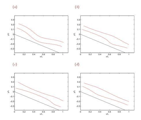
Figure 9.3.2 Snapshots of an evolving two-layer film down an inclined plane generated by code *films*. The interface and the free surface tend flatten under the combined action of gravity and interfacial tensions.
