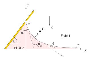
Figure 5.5.1 Illustration of a semi-infinite interface attached to an inclined plate. Far from the plate, the interface becomes horizontal.
