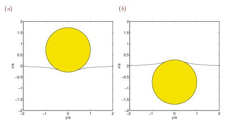
Figure 5.11.2 Axisymmetric interfacial profiles attached to a floating sphere for  $\lambda/a=1$  and (a)  $\kappa=0.5, \ \alpha=0.98\pi, \ \text{or} \ (b) \ \kappa=-0.5, \ \alpha=0.0242\pi.$
