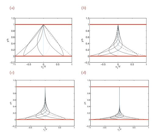
Figure 7.8.1 Periodic velocity profiles of oscillatory Couette flow in a two-dimensional channel confined between two parallel walls at phase angles  $\Omega t/\pi=0$  (dashed lines),  $0.25,\ 0.50$  (dotted lines),  $0.75,\ 1.0,\ 1.25,\ 1.50,\ 1.75,$  and 2.0, and Womersley number (a) Wo = 1, (b) 3, (c) 10, and (d) 20. In the first case, Wo = 1, the flow is nearly quasi-steady. As Wo increases, a Stokes boundary layer is established over the oscillating lower plate.
