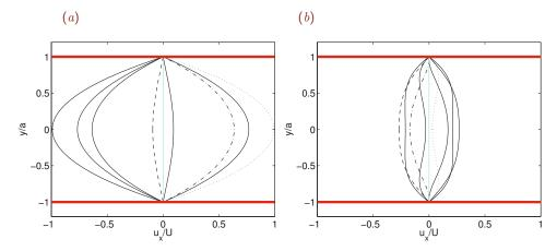
Figure 7.9.3 Velocity profiles of oscillatory pressure-driven flow in a circular tube at phase angles  $\Omega t/\pi=0$  (dashed lines), 0.25 (dash-dotted lines), 0.50 (dotted lines), 0.75, 1.0, 1.25, 1.50, 1.75, and 2.0, for Womersley number (a) Wo = 1 and (b) 6.
