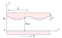
Figure 9.1.4 Lubrication flow in a furrowed channel confined between a translating plane wall and a stationary wavy wall.
