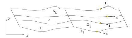
Figure 11.3.4 Illustration of an arrangement of  $N_L$  adjacent periodic vortex layers in two-dimensional flow in the xy plane.
