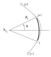
Figure 11.3.5 Local approximation of a vortex contour with a circular arc passing through three points, defined by its center and radius.
