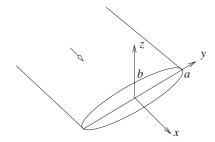
Figure 7.5.1 Illustration of steady unidirectional flow through a tube with elliptical cross-section.
