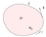
Figure 11.1.1 Illustration of a closed loop in a two-dimensional flow in the xy plane,  $\mathcal{L}$ , enclosing an area,  $\mathcal{D}$ . The circulation around the loop is equal to the areal integral of the strength of the vorticity,  $\omega_z$ , over  $\mathcal{D}$ . If the flow is irrotational, the circulation is zero.
