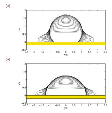
Figure 5.10.2 Shapes of (a) a sessile and (b) a pendant drops for contact angle  $\alpha = \frac{3}{4}\pi$  and  $\alpha = \frac{1}{4}\pi$  computed by code *drop\_ax* of FDLIB. The dotted lines show the approximate spherical shape arising for small drops or large surface tension.
