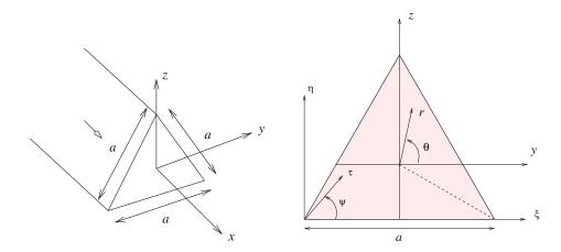
Figure 7.5.2 Illustration of steady unidirectional flow through a tube with equilateral triangular crosssectional shape. Cross-section of a triangular tube carrying fluid in pressure- or gravity-driven flow.
