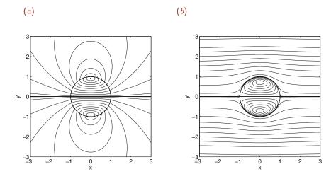
Figure 11.5.2 Streamline pattern associated with Hill's spherical vortex (a) in a stationary frame of reference and (b) in a frame of reference translating with the vortex.
