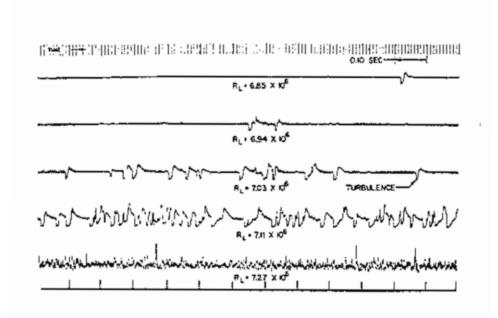
Figure 10.10.2 Record of the streamwise velocity component in flow past a flat plate at a sequence of increasing Reynolds numbers,  $\mathrm{Re}_L$ , defined with respect to the length of the plate, L. The signal shows the onset of oscillations, the development of turbulent spots, and the ultimate establishment of fully turbulent flow.
