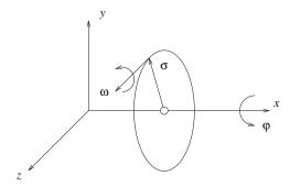
**Figure 11.5.1** Illustration of an axisymmetric flow without swirling motion. The vorticity vector points in the direction of the azimuthal angle,  $\varphi$ , at any point.
