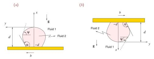
Figure 5.7.1 Illustration of a two-dimensional (a) sessile liquid drop or gas bubble resting on a horizontal plane and (b) pendant liquid drop or gas bubble hanging below a horizontal plane.
