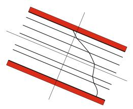
Figure 7.1.7 Velocity profile across six layers in channel flow between two inclined walls generated by code *chan\_2d\_ml*.
