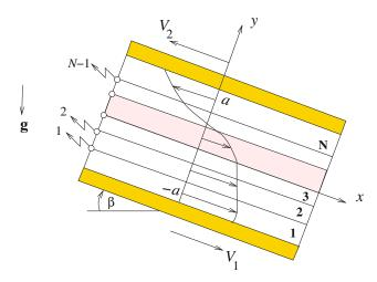
Figure 7.1.6 Illustration of steady flow of N layers through an inclined channel confined between two parallel walls located at  $y=\pm a$ . The interfacial labels are printed on the left and the layer labels are printed on the right.
