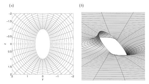
Figure 5.12.2 (a) Illustration of grid lines based on orthogonal elliptic coordinates. (b) Hydrostatic shape of a meniscus attached to a rotated circle computed in the elliptic coordinates.
