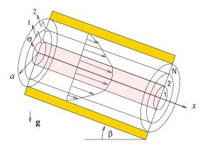
Figure 7.3.4 Illustration of multi-layer flow through a circular tube. The interface labels are shown on the left and the layer labels are shown on the right.
