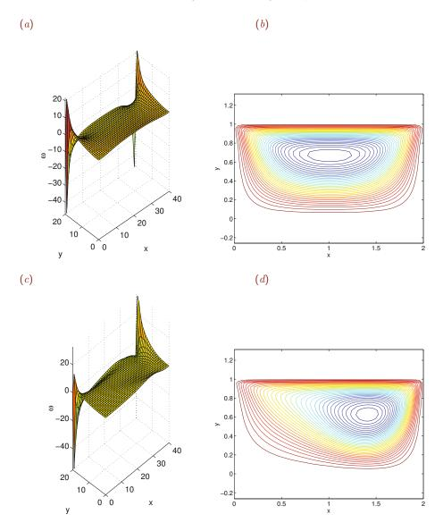
Figure 8.5.2 Vorticity and stream function contour plots for flow in a rectangular cavity with aspect ratio  $L_x/L_y=2$ , at Reynolds number  $(a,\ b)\ \mathrm{Re}=VL_x/\nu=1$  and  $(c,\ d)\ 100$ .
