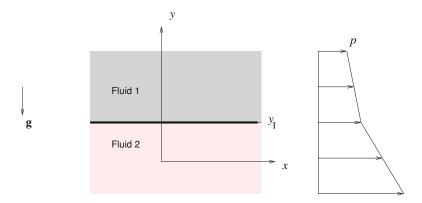
Figure 5.4.1 Illustration of an infinite horizontal interface located at  $y = y_{\rm I}$ , separating two stationary fluids. The pressure distribution is shown on the right.
