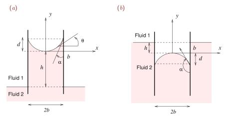
Figure 5.6.1 Illustration of a meniscus between two parallel vertical plates for contact angle (a)  $\alpha < \frac{1}{2}\pi$  and (b)  $\alpha > \frac{1}{2}\pi$ . In the second case, the meniscus submerges and the capillary rise h is negative.
