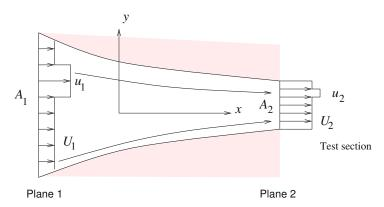
Figure 6.4.3 Illustration of flow in a wind or water tunnel with a contraction that dampens small perturbations.
