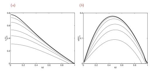
Figure 10.8.3 Instability of an inviscid shear flow with hyperbolic tangent velocity profile described by equation (10.8.16) with  $\alpha=1$ . Graphs of (a) the scaled imaginary part of the phase velocity,  $c_{\rm I}/U_0$ , and (b) scaled growth rate,  $\sigma_{\rm I}\delta/U_0$ , for  $a/\delta=b/\delta=2.0, 2.5, 3.0, 4.0, 5.0$ , and 6.0 (heavy lines), in the regime of unstable wave numbers.
