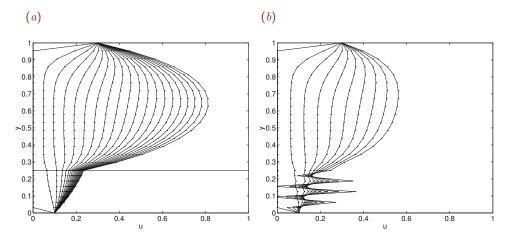
Figure 8.2.3 Evolving profiles of two-layer flow in a channel, computed by an explicit finite difference method for (a)  $\alpha = 0.4$  and (b) 0.52, where  $\alpha$  is the minimum of  $\alpha_1$  and  $\alpha_2$ . A numerical instability arises in the second case.
