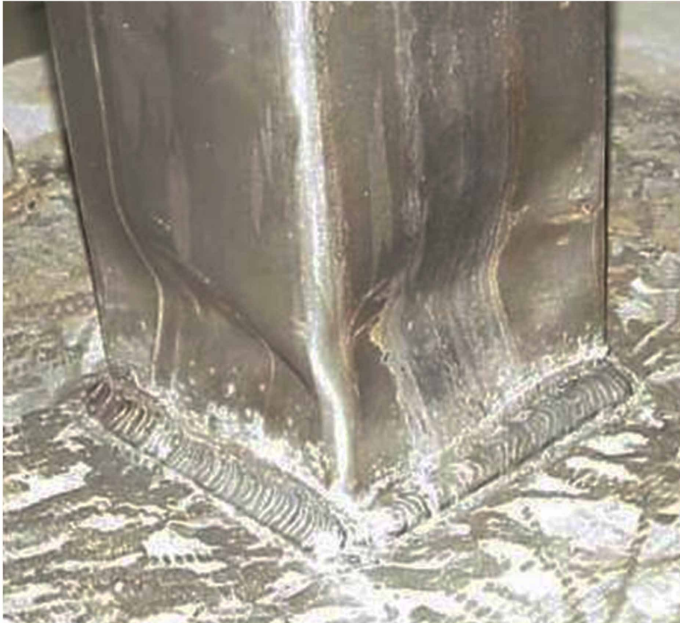
Figure 23. Local buckling in a biaxial test
