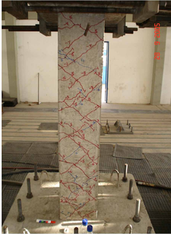
Figure 42. Cracking pattern in a square element subjected to cyclic loads
