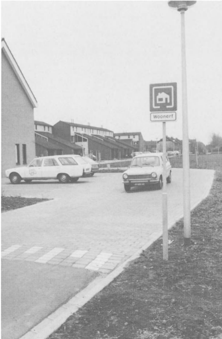
Figure 4. A woonerf , or “residential yard,” has a special sign to announce that cars, pedestrians, children playing, and bicycles all have equal rights.
