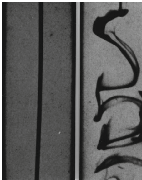
Fig. 10.1 Laminar and turbulent flows. Laminar and turbulent flows in a circular pipe. In order to make the flow visible, a fine jet of ink is added to a water filament in the middle of the pipe cross section at the upper end of the pipe. The capillary, from which the ink jet is added, is visible at the upper edge of the figure. In the panel on the right, axial velocities are larger than on the left. The streaklines entering from the capillary are now driven to the side and torn apart, so that eventually the entire cross section is filled with the dye added to the capillary fluid. From P. FRAUENFELDER and P. HUBER, Einführung in die Physik, Ernst Reinhardt Verlag, Basel
