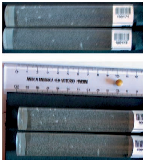
FIGURE 17.7. Showing both the unscreened Defenders used in the cavitation run with the Iron Nitrate solution. The bubbles are spread all over the detecting volume
