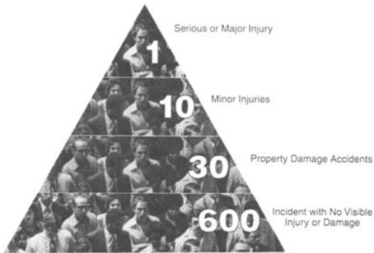
Figure 8-4 Safety Accident Pyramid. Source: Bird and Germain, Loss Control Management: Practical Loss Control Leadership , 3 Figure 1-3, adapted for use, designed by Damon Carter. See also Roughton and Mercurio, 5 p. 70.
