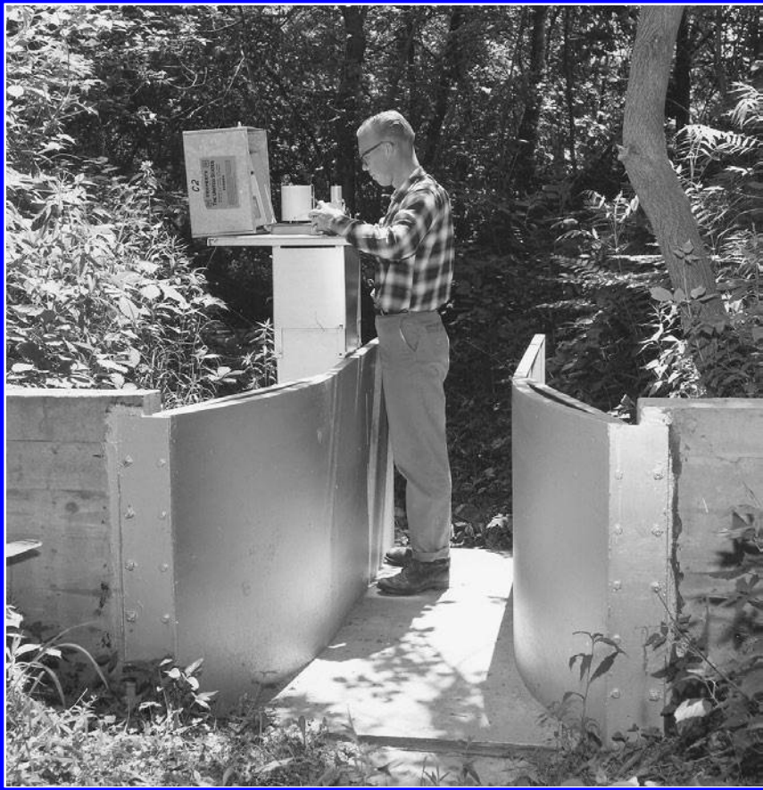
Figure 9.8 A San Dumas flume weir with recording device. Note the solid concrete walls to which the steel flume is attached. A special mortar mix assures that these dams are tightly connected to bedrock so that no leakage occurs. (USDA Forest Service photo by B. Muir)
