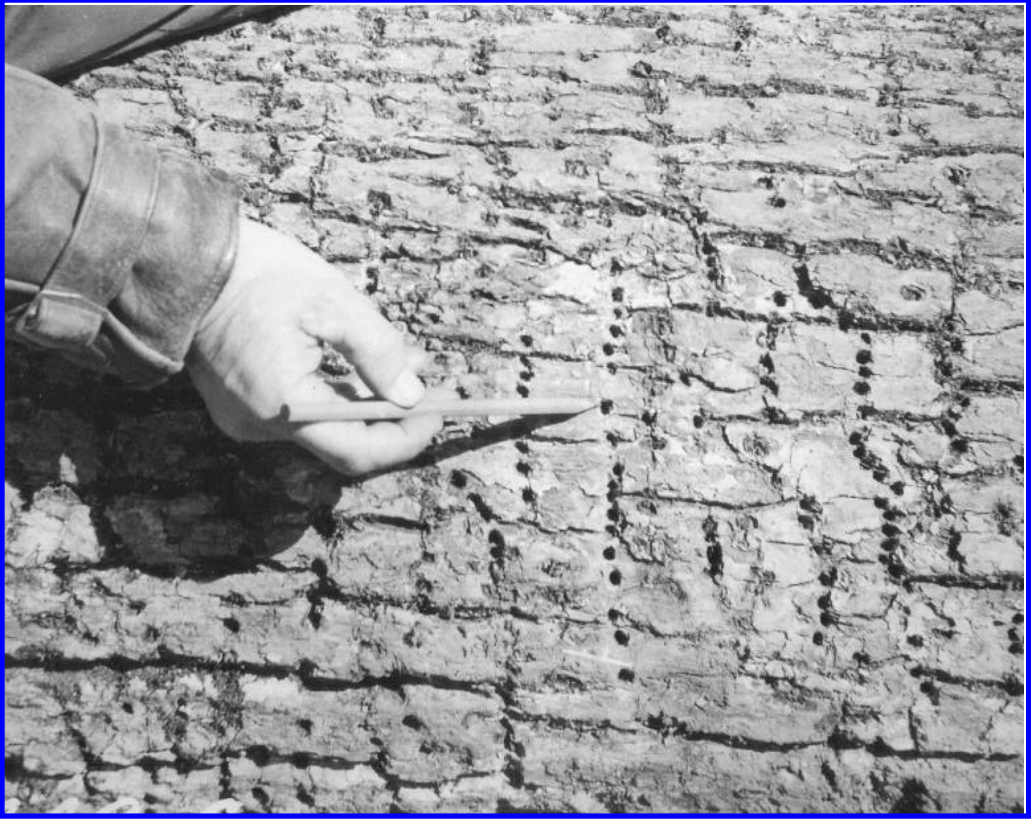
Figure 6.20 Bird-peck on a yellow-poplar bole. Such defects may affect the quality of lumber sawn from the logs of these trees. (Tennessee Valley Authority photo)
