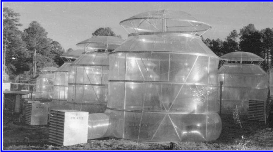
Figure 6.30 Plastic tents for acid-rain studies. Gases and ambient air piped into these structures in which trees have been planted enable researchers to analyze the effects of effluent contaminants in the atmosphere.
