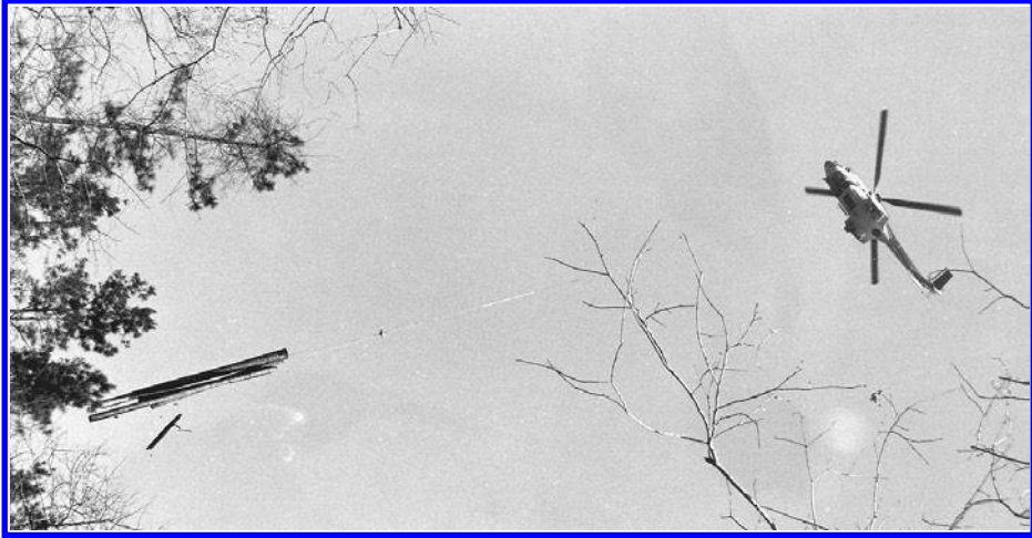
Figure 9.12 Helicopter logging. Four logs are cabled together for aerial skidding to salvage beetle-killed pines or to remove hurricane-downed, fire-hazard, windthrown trees without otherwise disturbing the site in a wilderness area. (Texas Forest Service photo by R. Billings)
