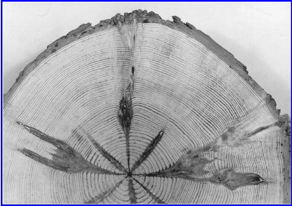
Figure 7.5 Knots reduce lumber and wood quality. This cross-section at the place on the bole where a whorl of branches radiates from the trunk shows the effect. Once the tree is pruned, whether manually or naturally, wood later laid down on the trunk is free of the defect. (USDA Forest Service photo)
