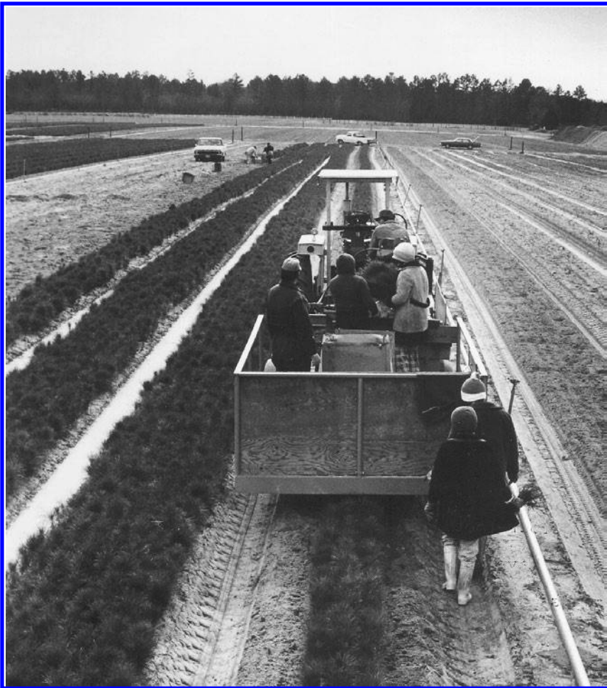
Figure 5.17 Mechanized tree-lifting machine. Pine seedlings are removed from four-foot-wide nursery beds and bundled. Trees in the beds to the right have been harvested, and the beds now await spring planting. (authors' collection)
