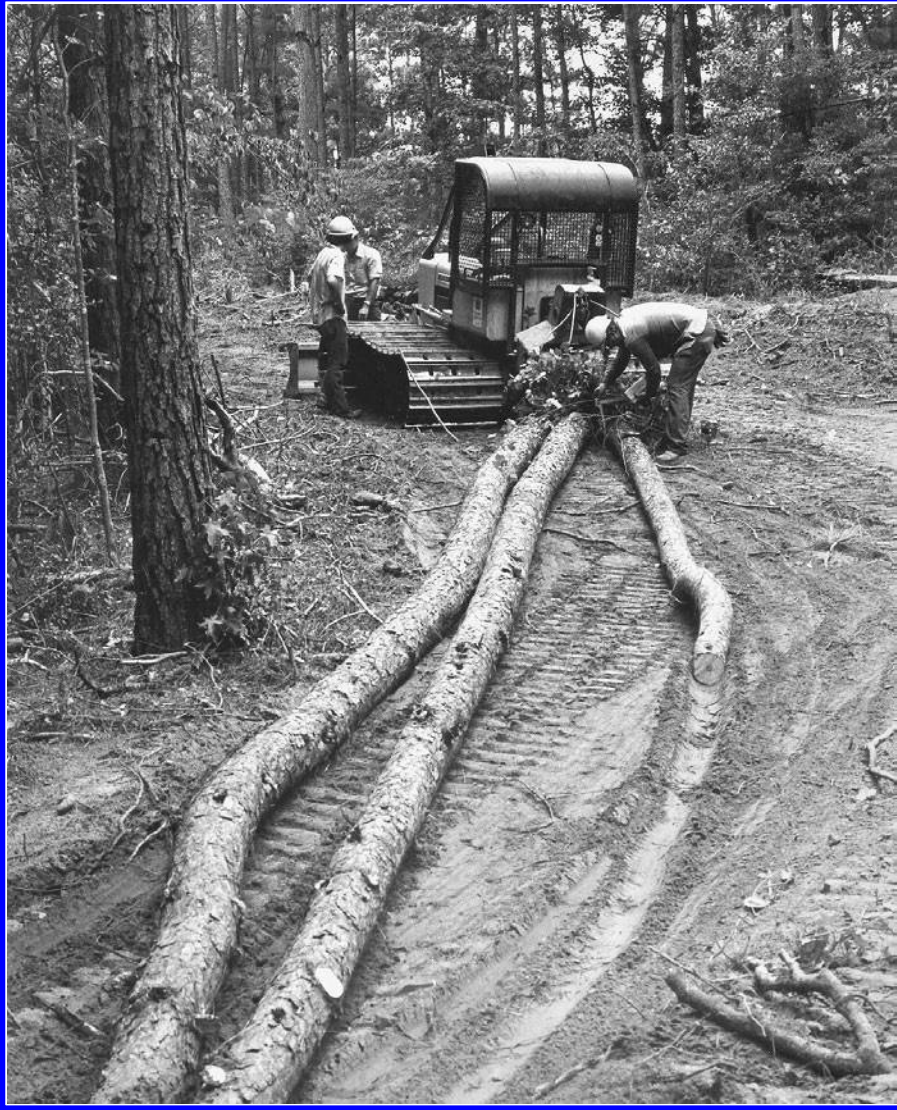
Figure 9.11 Wide-track crawler tractor. While logging should cease during wet periods, the wide tracks disperse the weight of the machines, thereby reducing soil compaction and puddling of the soil. (Texas Forest Service photo by R. Billings)
