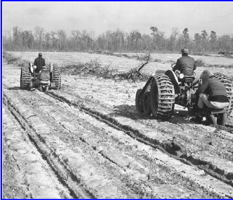
Figure 5.22 Tree-planting machines expedite reforestation. Rear wheels pack the soil around the roots after the worker has placed the seedling in a slit made by the plow. (authors' collection)
