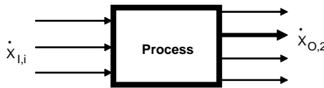
FIGURE 2.5 The transfer of substance X into output flow 2 is given as TC_2 = \dot{X}_{O,2} / \sum_i \dot{X}_{1,i} .
