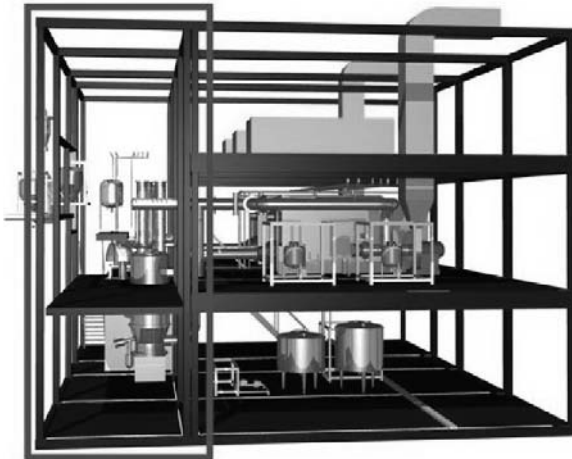
Fig. 2. Modular construction of a pharmaceutical facility. The frames indicate the steel modules used to assemble the facility (reproduced with kind permission of Pharmadule, Sweden).
