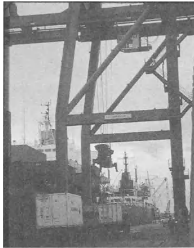
Figure 1.2. Overhead shipyard crane loader/unloader in Gulfport, Mississippi
