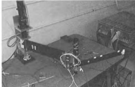
Figure 1: WAYA Research, Inc. designed, manufactured, and delivered flexible two-link robot for Sandia By permission of WAYA Research, Inc. ©1995
