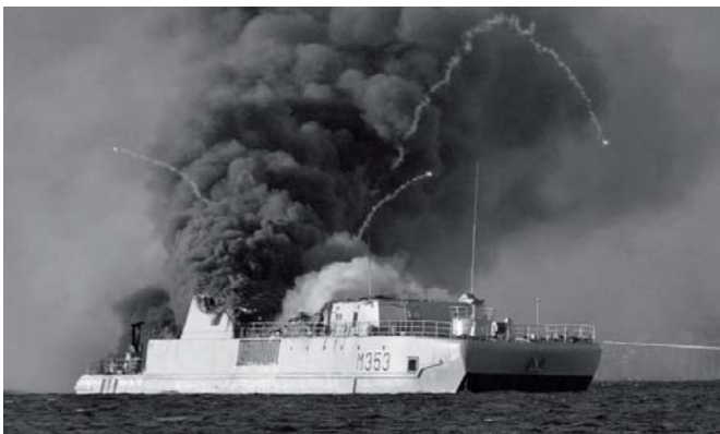
Figure 1.14. The composite minesweeper KNM Orkla sunk due to fire. Photograph supplied courtesy of Summmørsposten.
