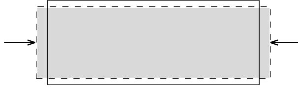
Fig. 57. A compression of a body in one direction leads to an expansion in the other directions. The relative size is given by the Poisson ratio \nu .
