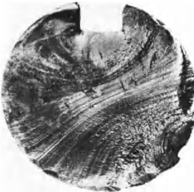
Fig. 2.4 Failure case due to fatigue crack growth on a shaft
